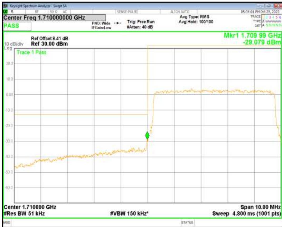
Band4 16QAM BW=5MHz Channel=20375 RB Size=25 Position=#0
