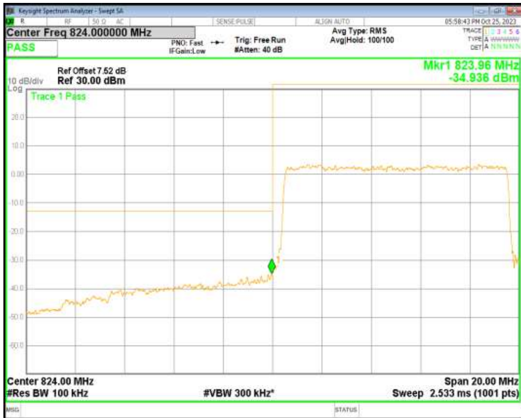
Band5 16QAM BW=10MHz Channel=20600 RB Size=50 Position=#0
