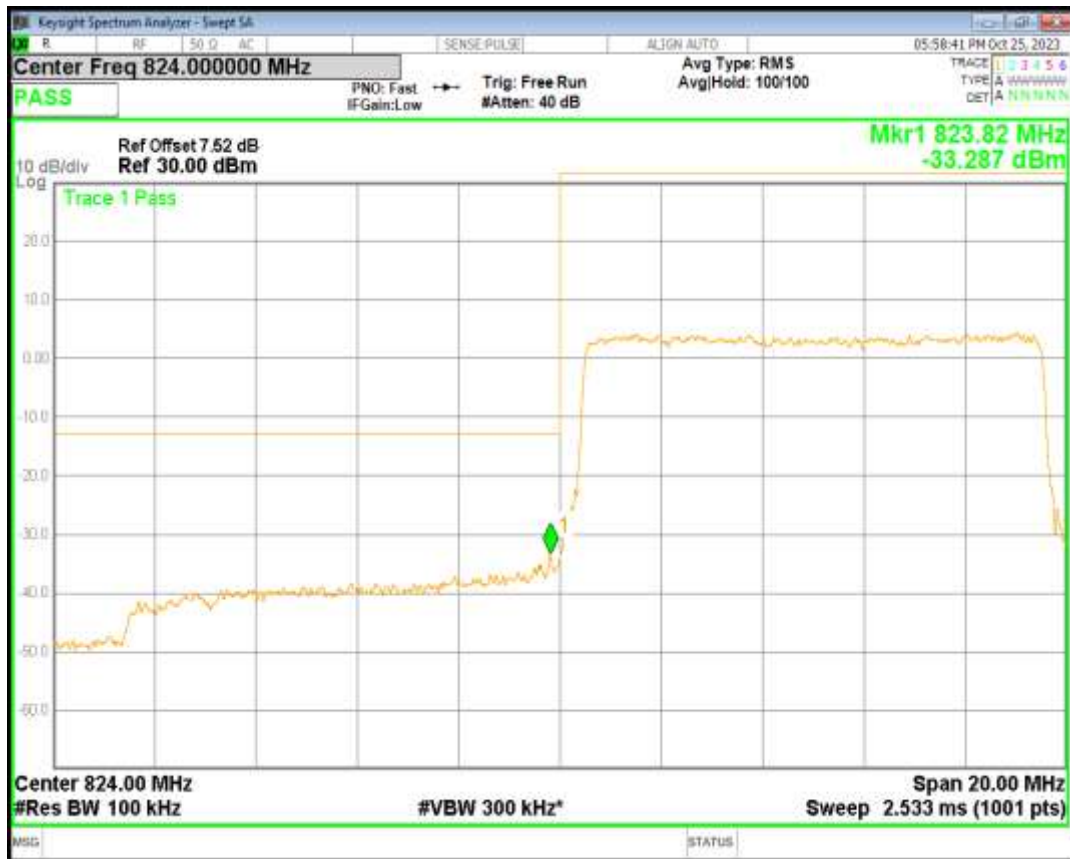
Band5 QPSK BW=10MHz Channel=20600 RB Size=50 Position=#0
