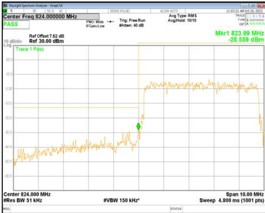
Band26(824-849) 16QAM BW=5MHz Channel=27015 RB Size=25 Position=#0
