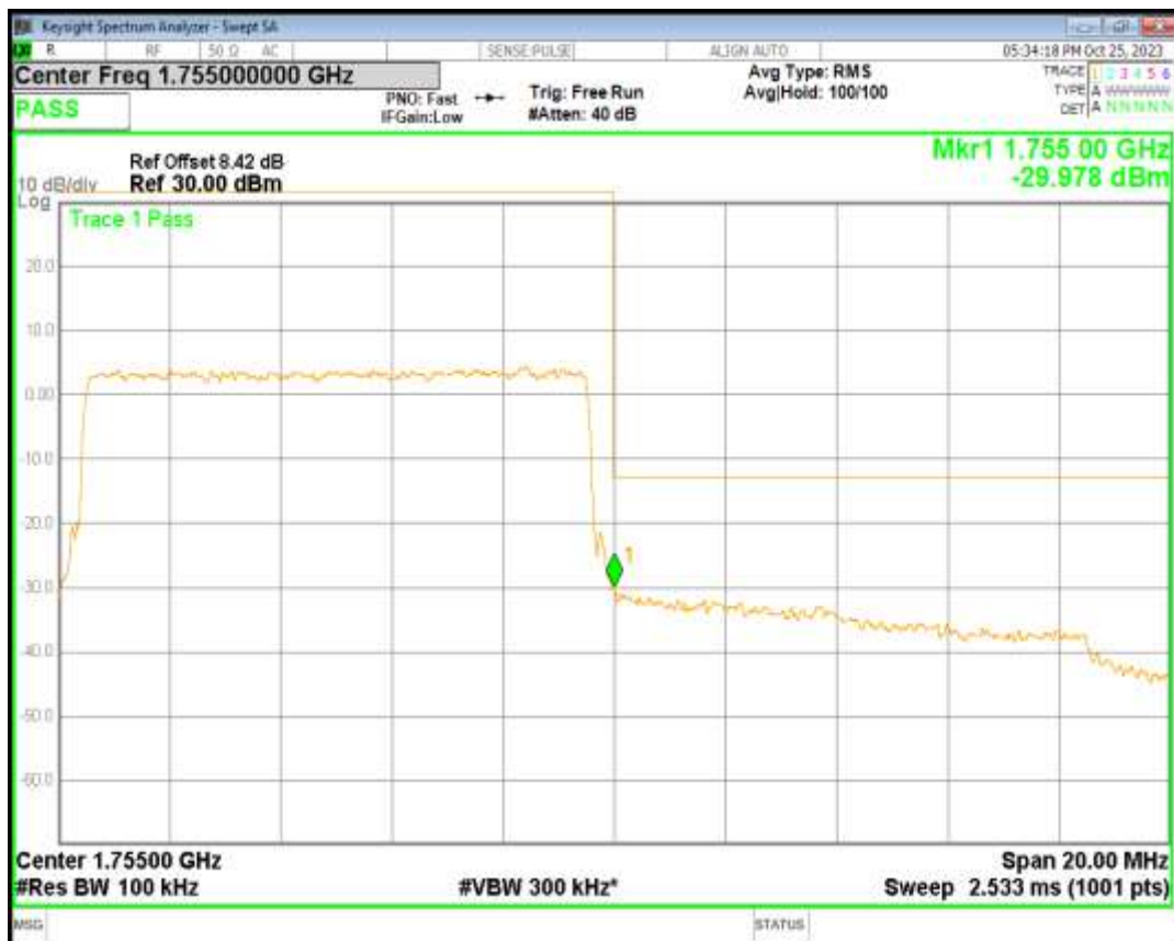
Band4 QPSK BW=15MHz Channel=20025 RB Size=75 Position=#0
