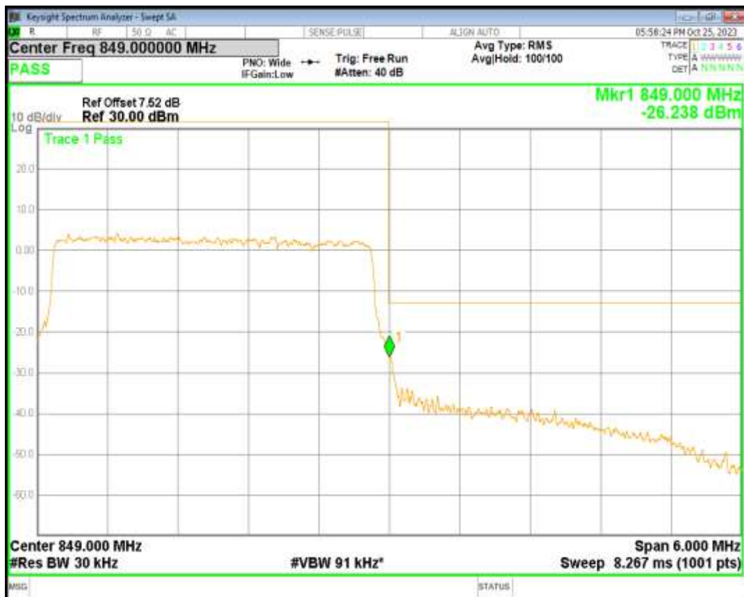
Band5 16QAM BW=5MHz Channel=20425 RB Size=25 Position=#0
