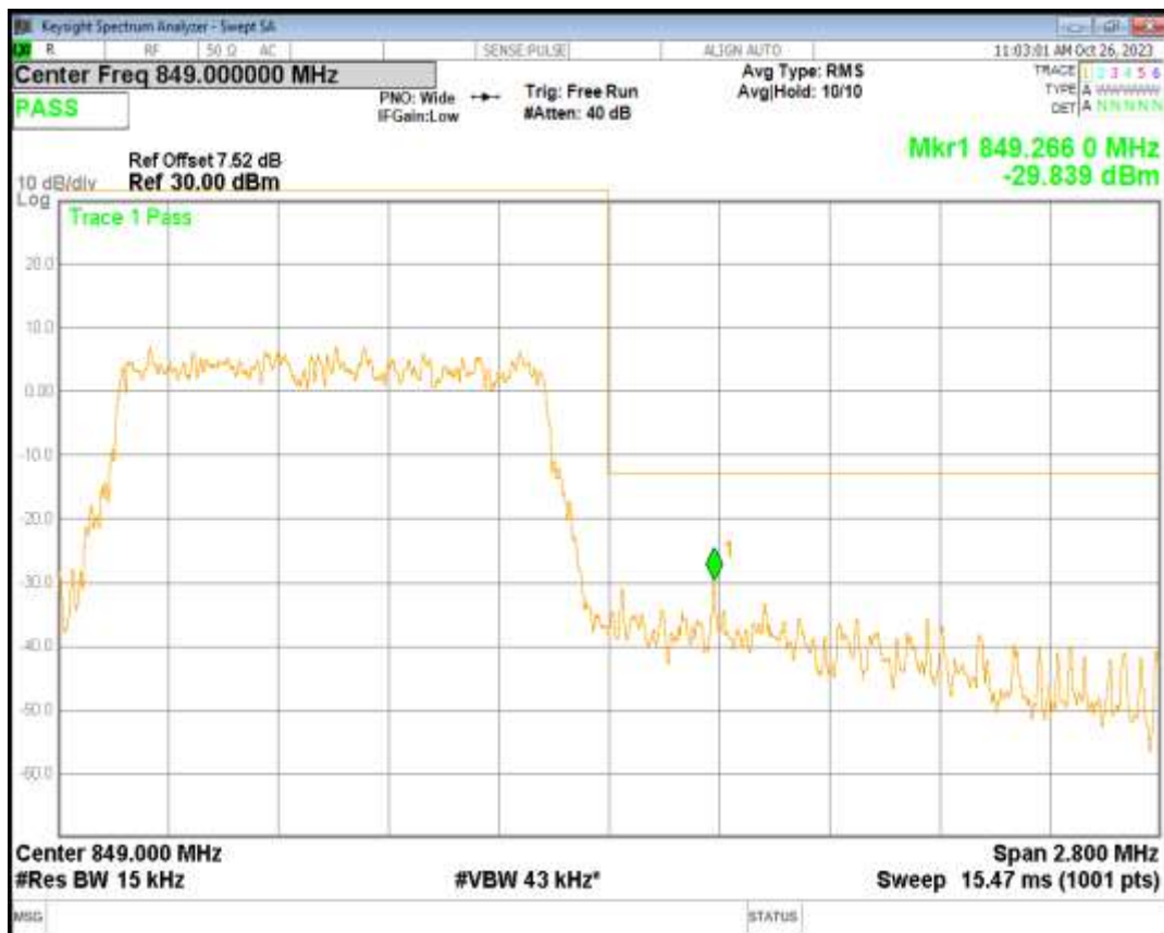
Band26(824-849) 16QAM BW=10MHz Channel=26840 RB Size=50 Position=#0
