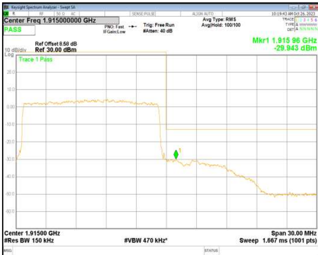
Band25 QPSK BW=20MHz Channel=26140 RB Size=100 Position=#0
