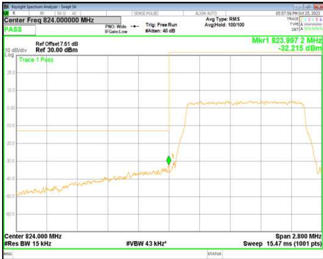
Band5 16QAM BW=1.4MHz Channel=20643 RB Size=6 Position=#0
