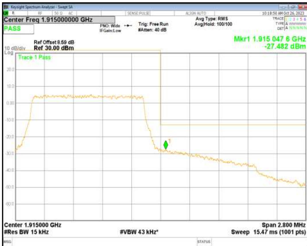
Band25 QPSK BW=10MHz Channel=26090 RB Size=50 Position=#0
