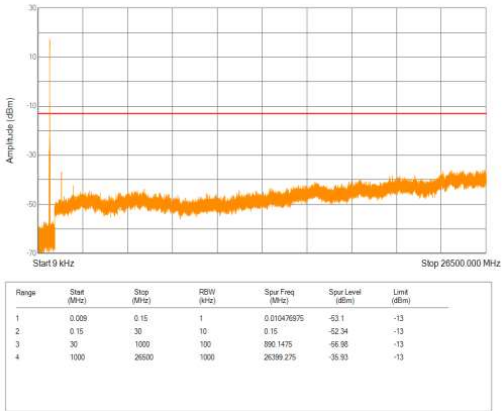
Band12 QPSK BW=3MHz Channel=23095 RB Size=15 Position=#0
