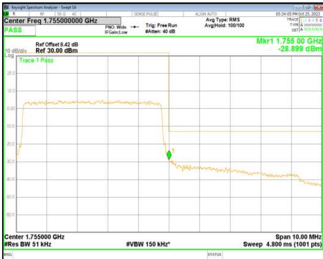
Band5 16QAM BW=1.4MHz Channel=20407 RB Size=6 Position=#0
