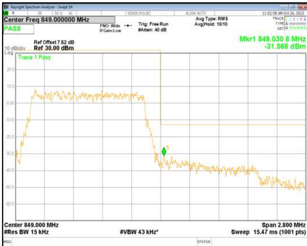
Band26(824-849) QPSK BW=10MHz Channel=26840 RB Size=50 Position=#0
