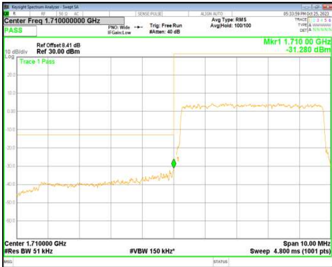
Band4 QPSK BW=5MHz Channel=20375 RB Size=25 Position=#0
