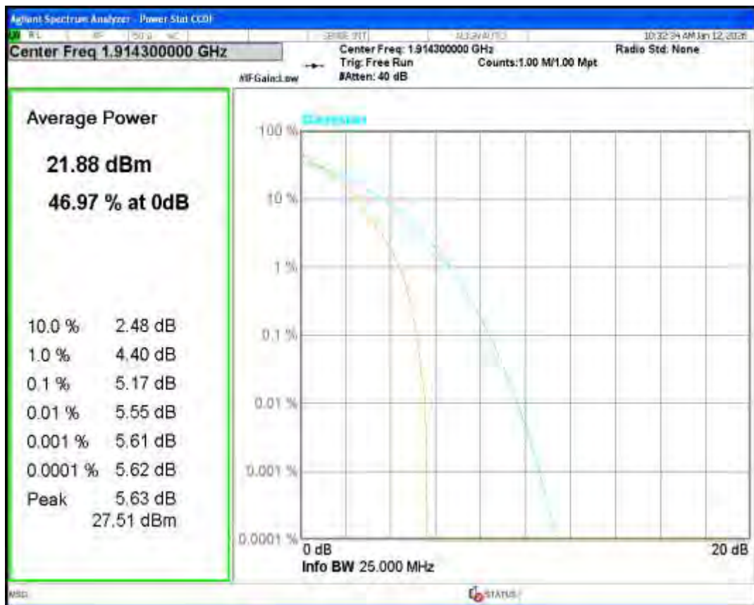
Band25 QPSK BW=3MHz Channel=26055 RB Size=1 Position=#0
