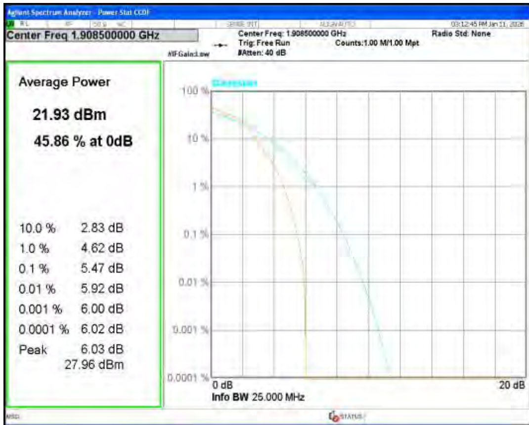
Band2 16QAM BW=5MHz Channel=18625 RB Size=1 Position=#0
