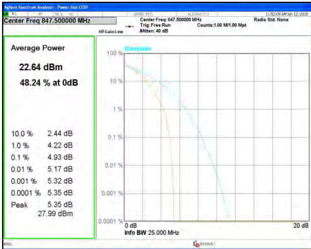
Band26(824-849) QPSK BW=5MHz Channel=26815 RB Size=1 Position=#0
