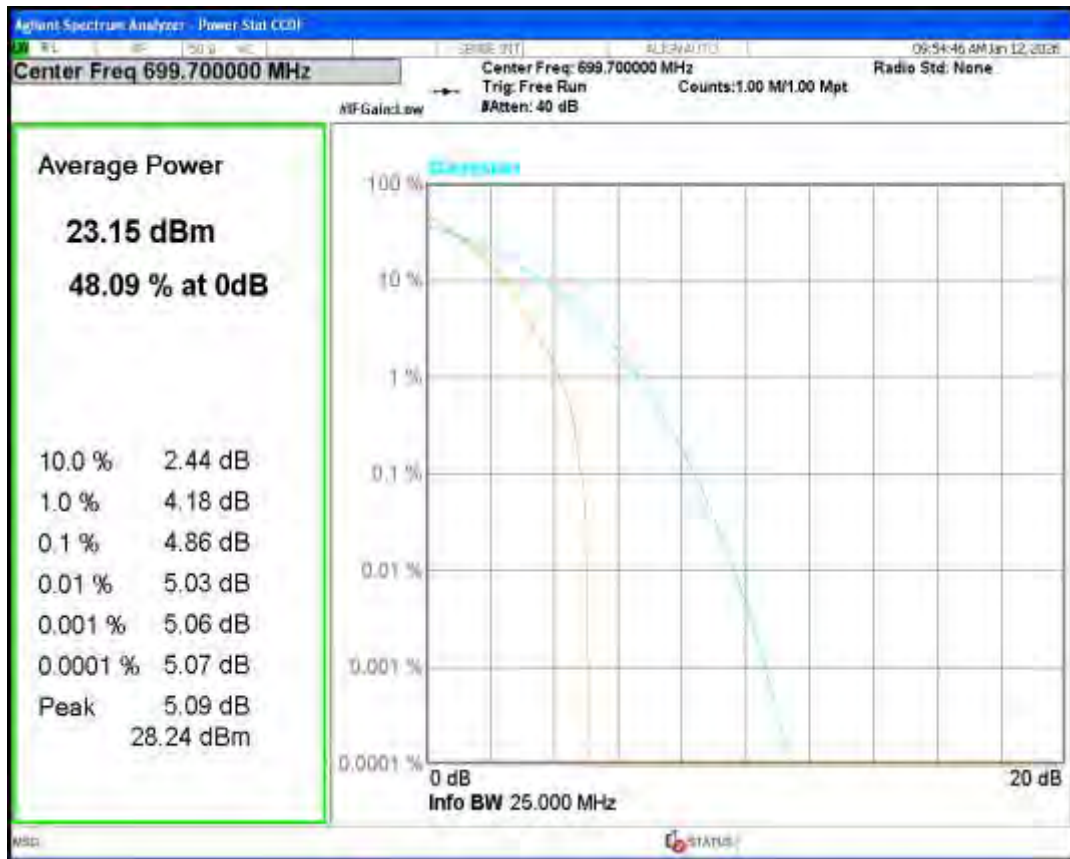
Band12 QPSK BW=1.4MHz Channel=23095 RB Size=1 Position=#0
