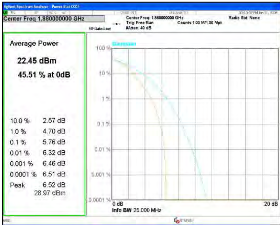
Band2 QPSK BW=20MHz Channel=19100 RB Size=1 Position=#0
