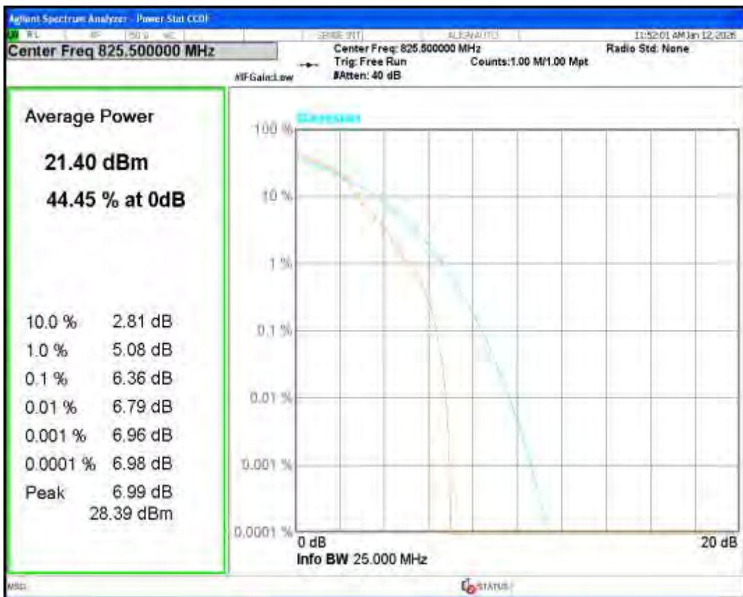
Band26(824-849) 16QAM BW=3MHz Channel=26915 RB Size=1 Position=#0
