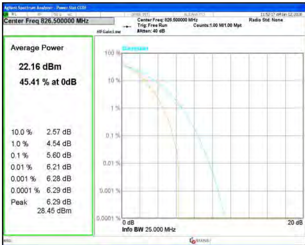
Band26(824-849) QPSK BW=5MHz Channel=26915 RB Size=1 Position=#0
