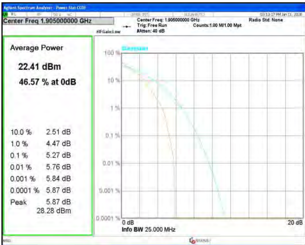
Band2 QPSK BW=15MHz Channel=18675 RB Size=1 Position=#0
