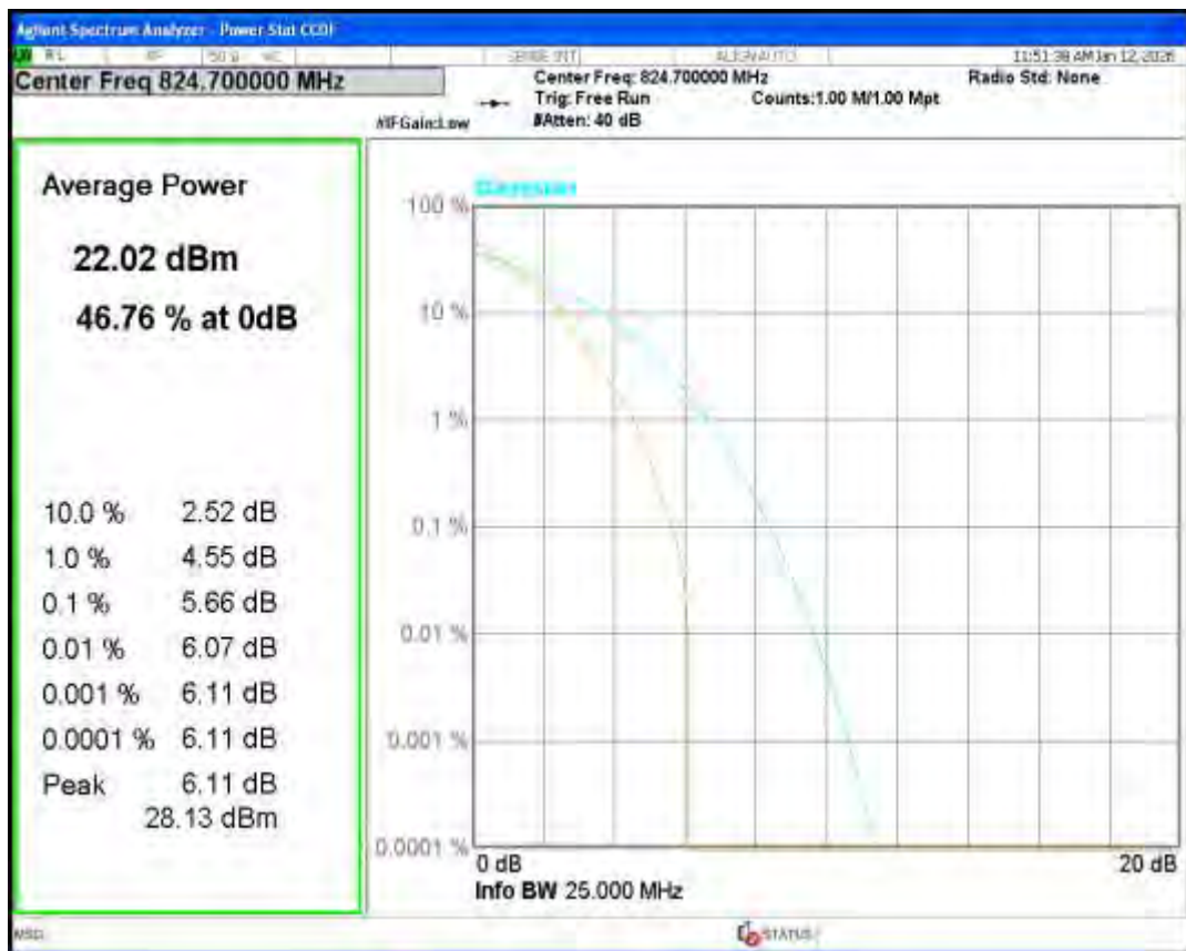
Band26(824-849) 16QAM BW=5MHz Channel=27015 RB Size=1 Position=#0
