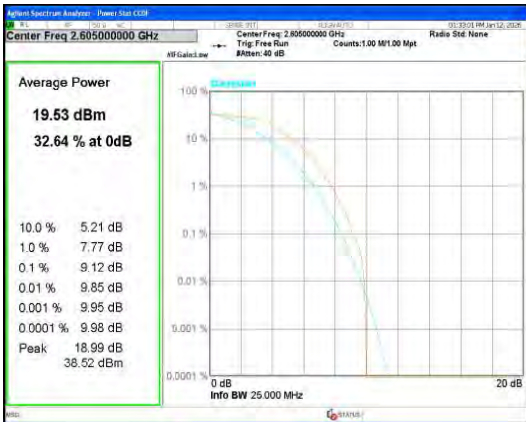
Band41(2555-2655) QPSK BW=10MHz Channel=41190 RB Size=1 Position=#0
