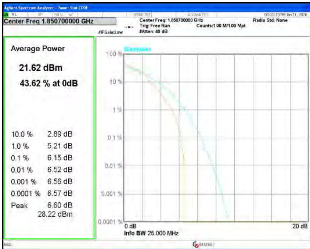
Band2 16QAM BW=1.4MHz Channel=18900 RB Size=1 Position=#0
