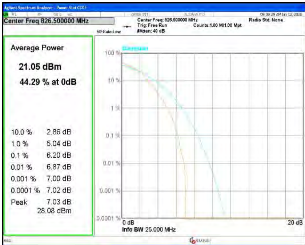
Band5 QPSK BW=1.4MHz Channel=20407 RB Size=1 Position=#0
