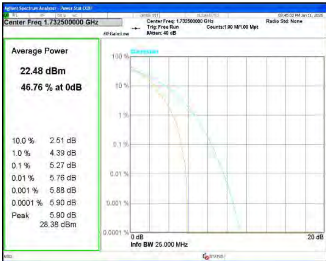
Band4 QPSK BW=1.4MHz Channel=20393 RB Size=1 Position=#0
