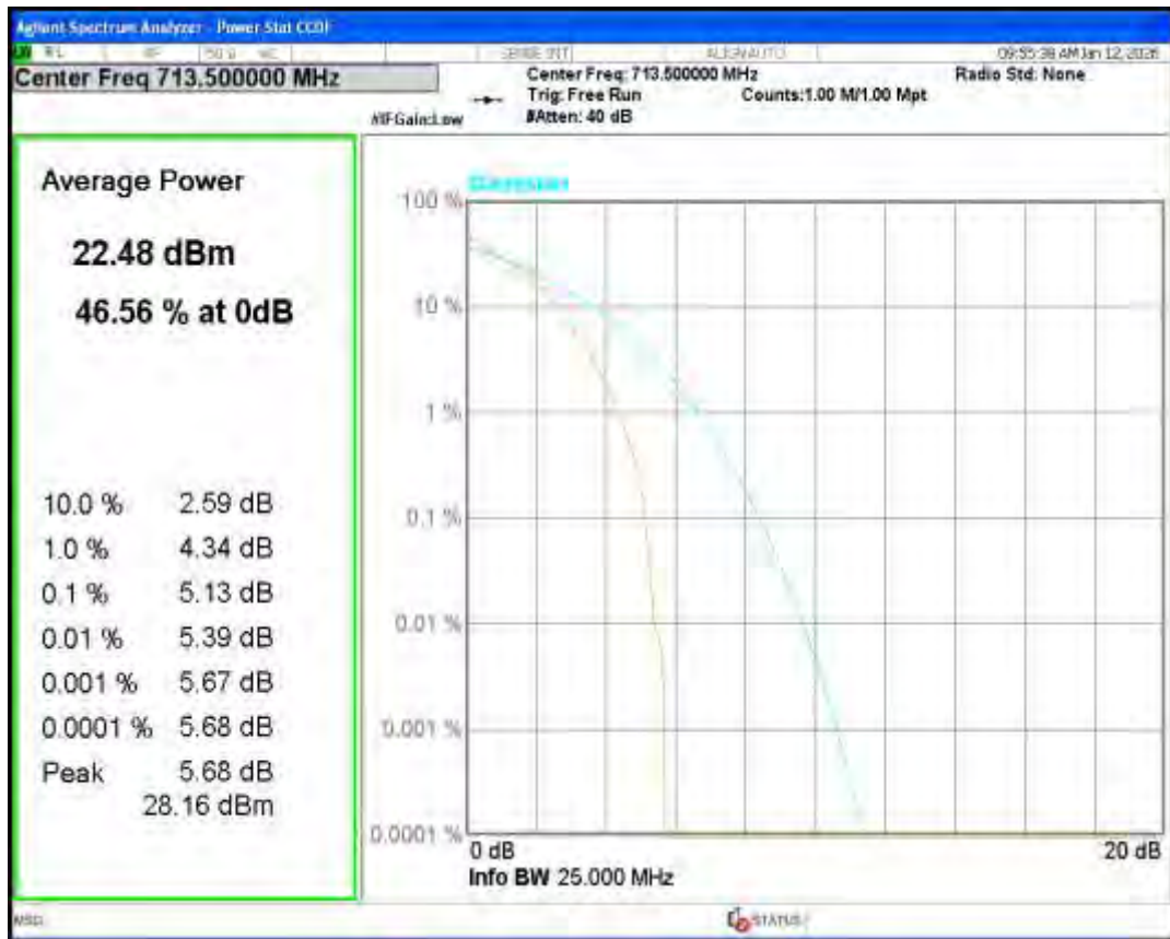
Band12 QPSK BW=10MHz Channel=23060 RB Size=1 Position=#0
