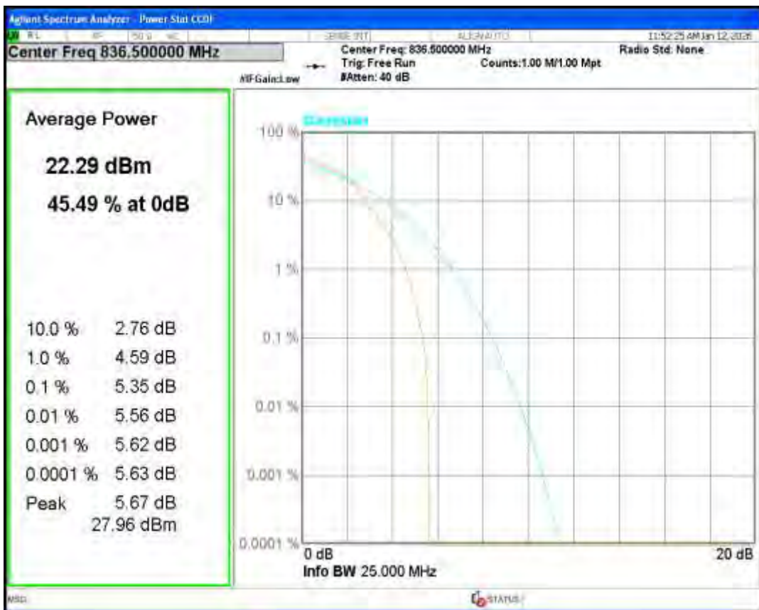
Band26(824-849) QPSK BW=1.4MHz Channel=26915 RB Size=1 Position=#0
