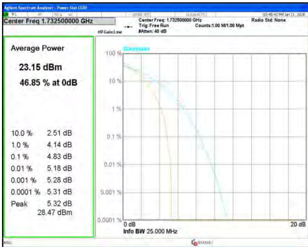
Band4 QPSK BW=5MHz Channel=20375 RB Size=1 Position=#0
