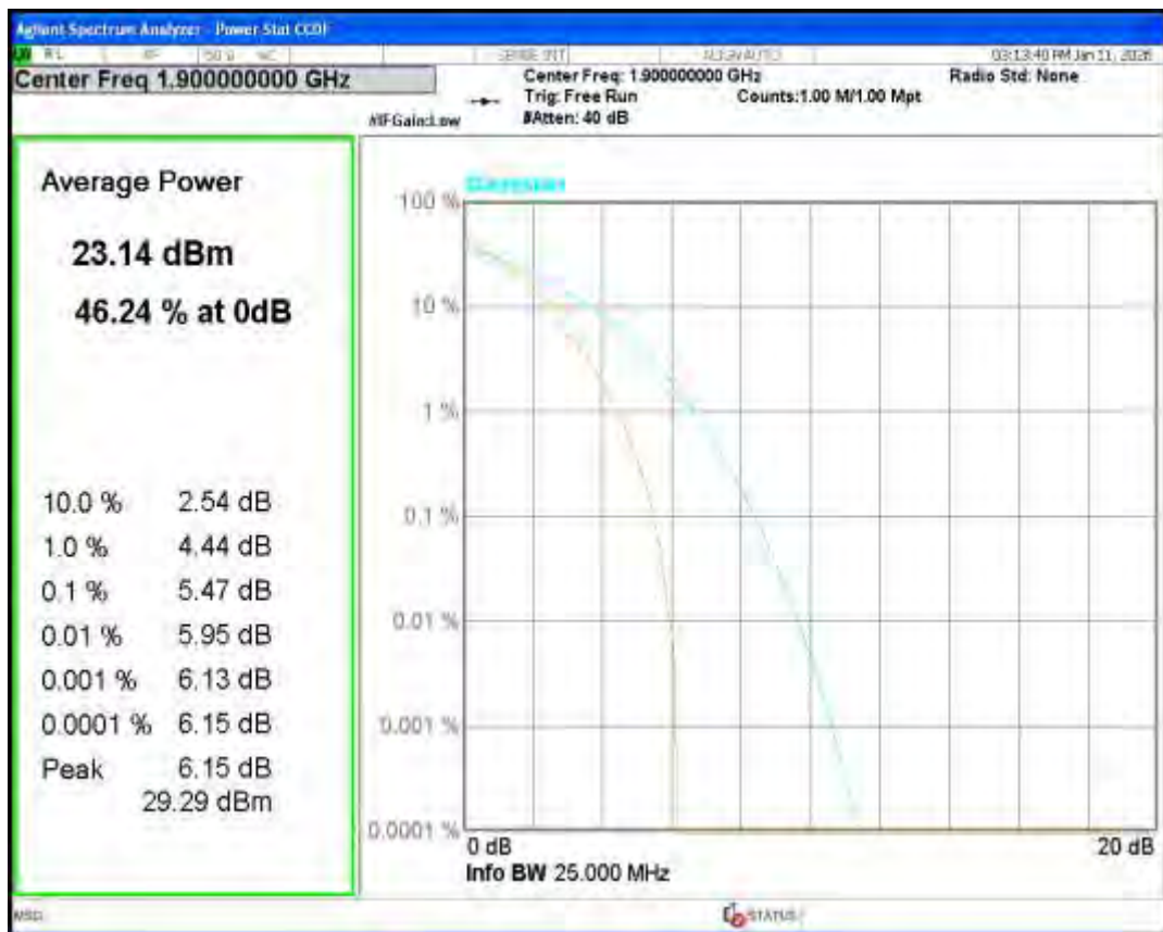
Band25 16QAM BW=1.4MHz Channel=26047 RB Size=1 Position=#0
