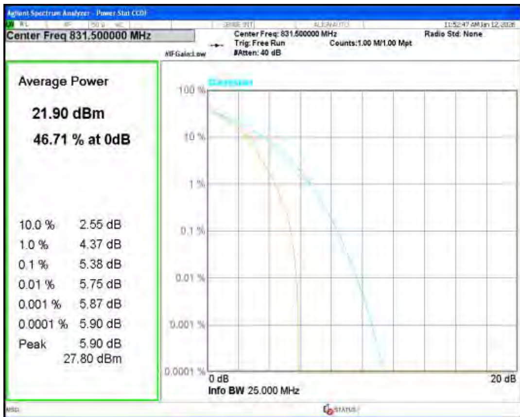
Band26(824-849) QPSK BW=15MHz Channel=26915 RB Size=1 Position=#0
