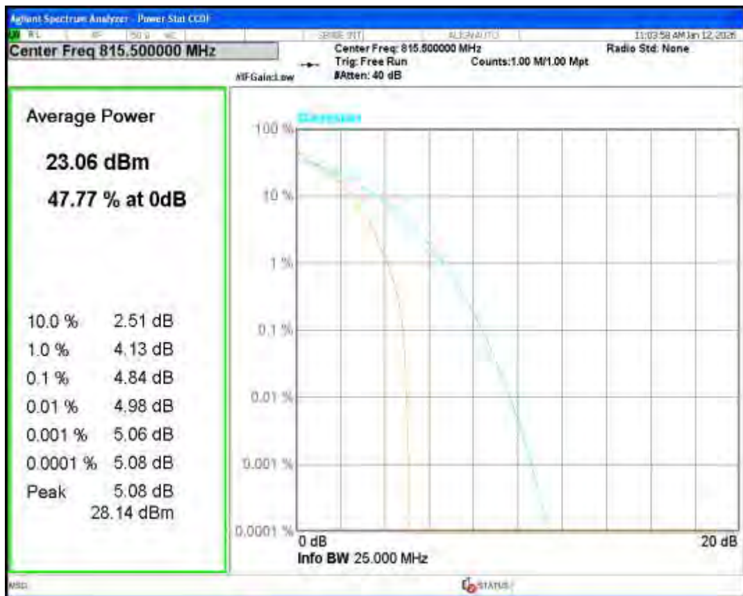
Band26(814-824) QPSK BW=3MHz Channel=26740 RB Size=1 Position=#0
