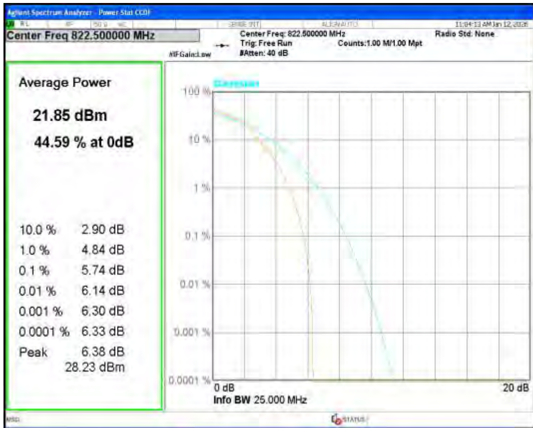
Band26(814-824) 16QAM BW=5MHz Channel=26715 RB Size=1 Position=#0
