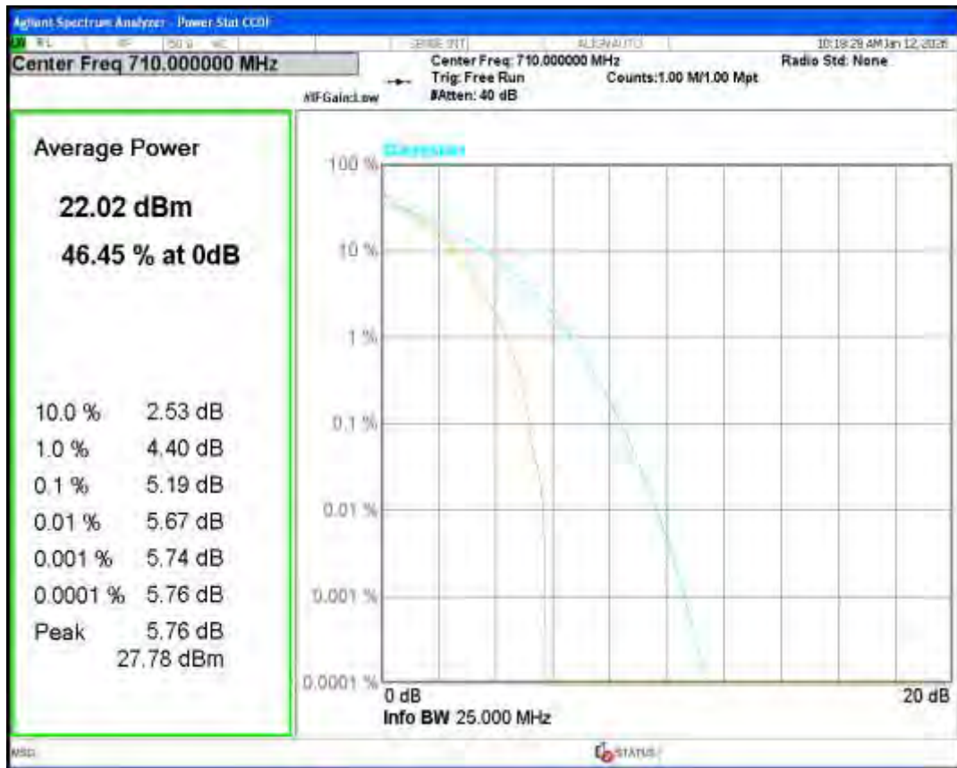
Band17 QPSK BW=5MHz Channel=23825 RB Size=1 Position=#0
