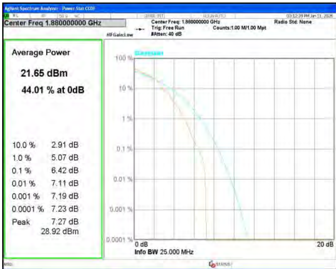
Band2 16QAM BW=3MHz Channel=19185 RB Size=1 Position=#0
