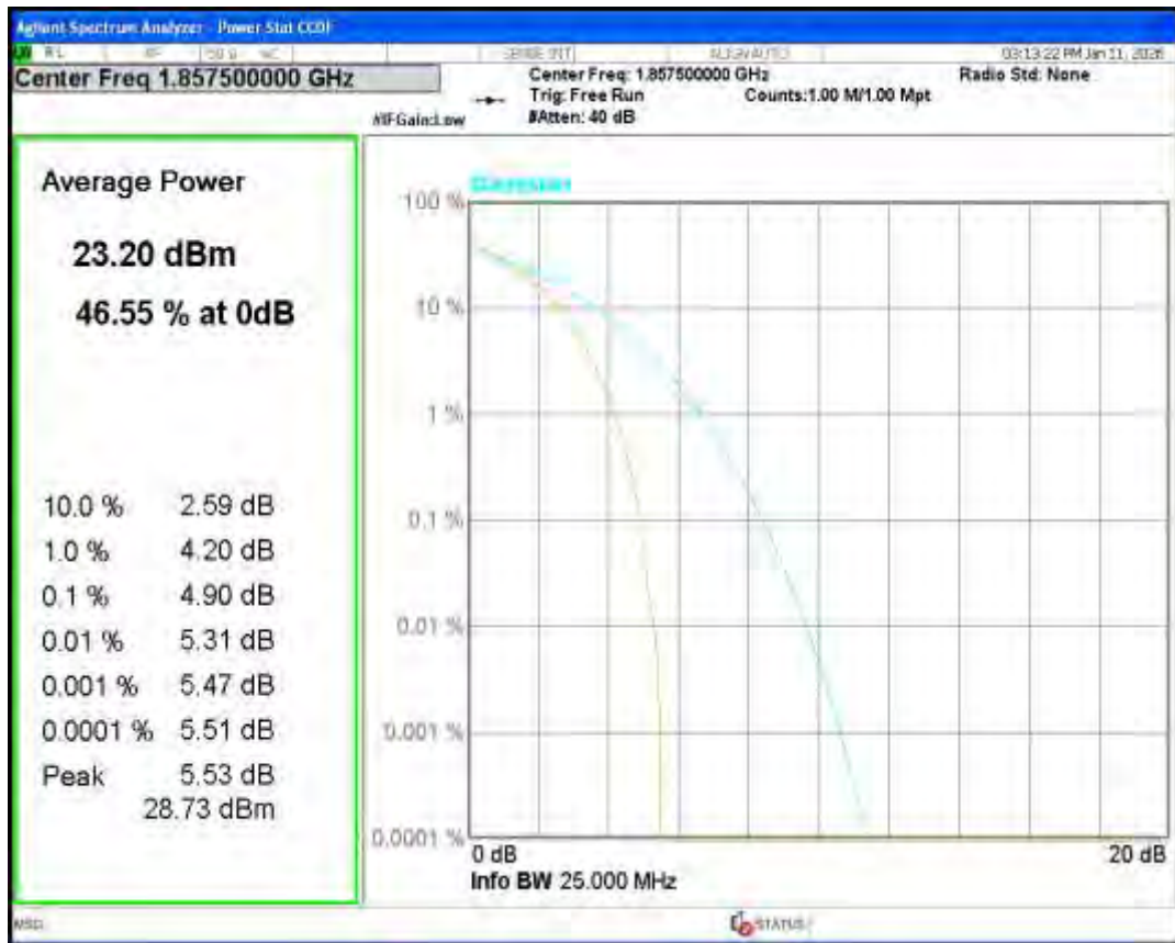
Band2 QPSK BW=15MHz Channel=18900 RB Size=1 Position=#0
