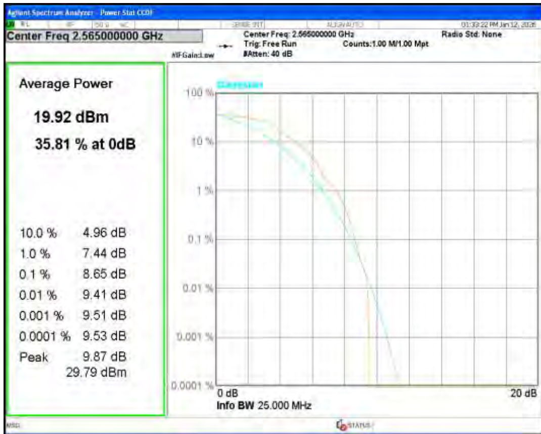
Band41(2555-2655) QPSK BW=20MHz Channel=40740 RB Size=1 Position=#0
