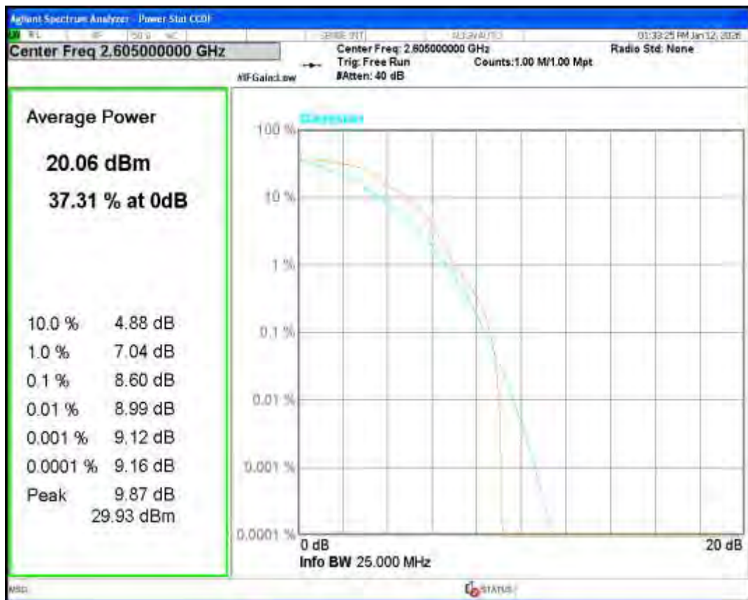
Band41(2555-2655) QPSK BW=20MHz Channel=41140 RB Size=1 Position=#0
