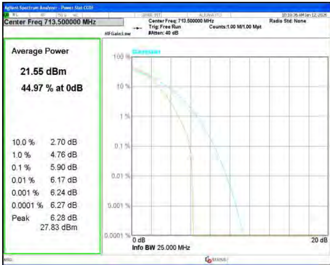
Band17 QPSK BW=5MHz Channel=23755 RB Size=1 Position=#0
