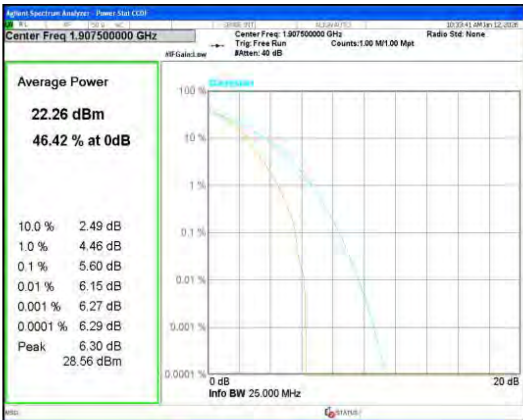
Band25 QPSK BW=20MHz Channel=26140 RB Size=1 Position=#0
