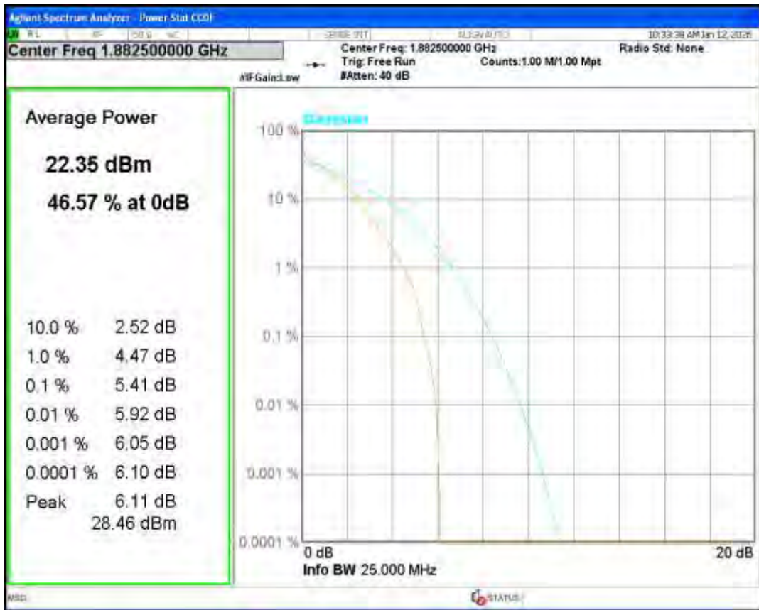
Band25 QPSK BW=15MHz Channel=26615 RB Size=1 Position=#0
