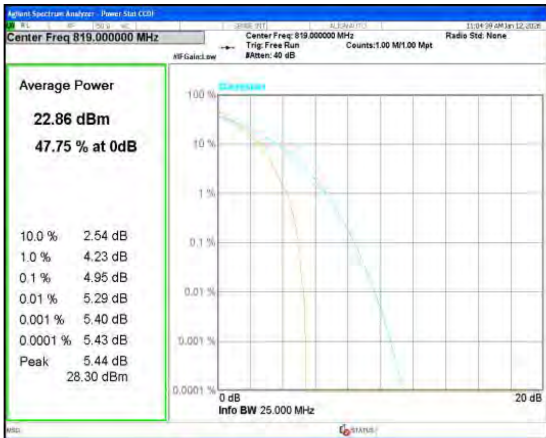
Band26(824-849) 16QAM BW=1.4MHz Channel=26797 RB Size=1 Position=#0
