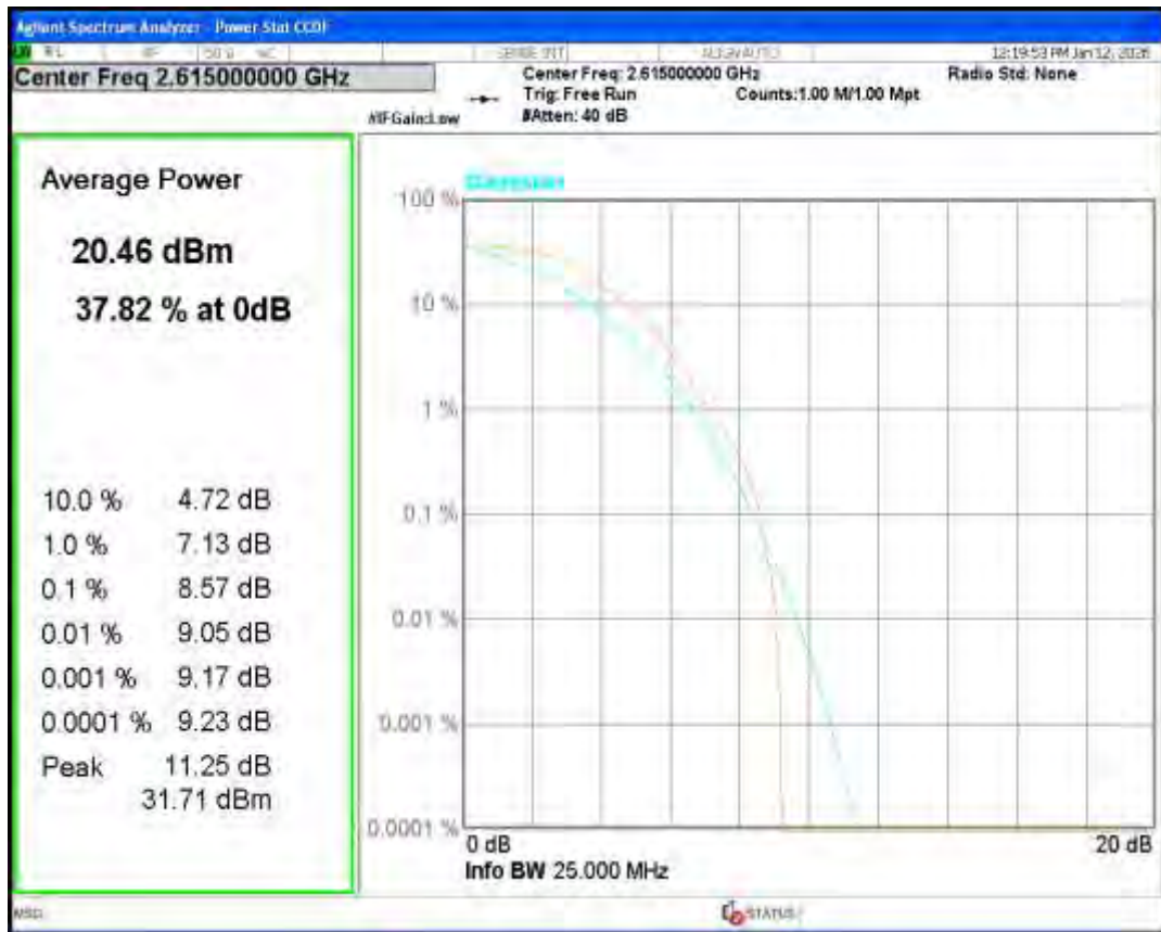
Band38 QPSK BW=15MHz Channel=37825 RB Size=1 Position=#0
