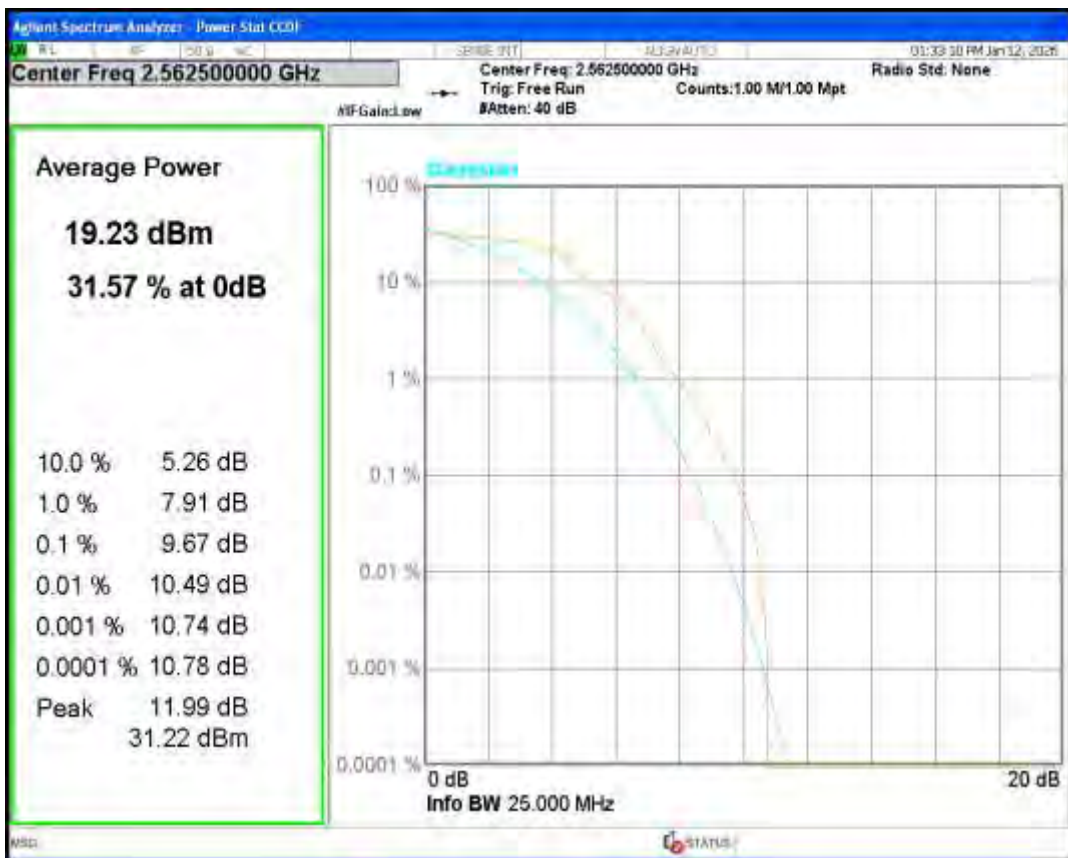
Band41(2555-2655) QPSK BW=15MHz Channel=40740 RB Size=1 Position=#0
