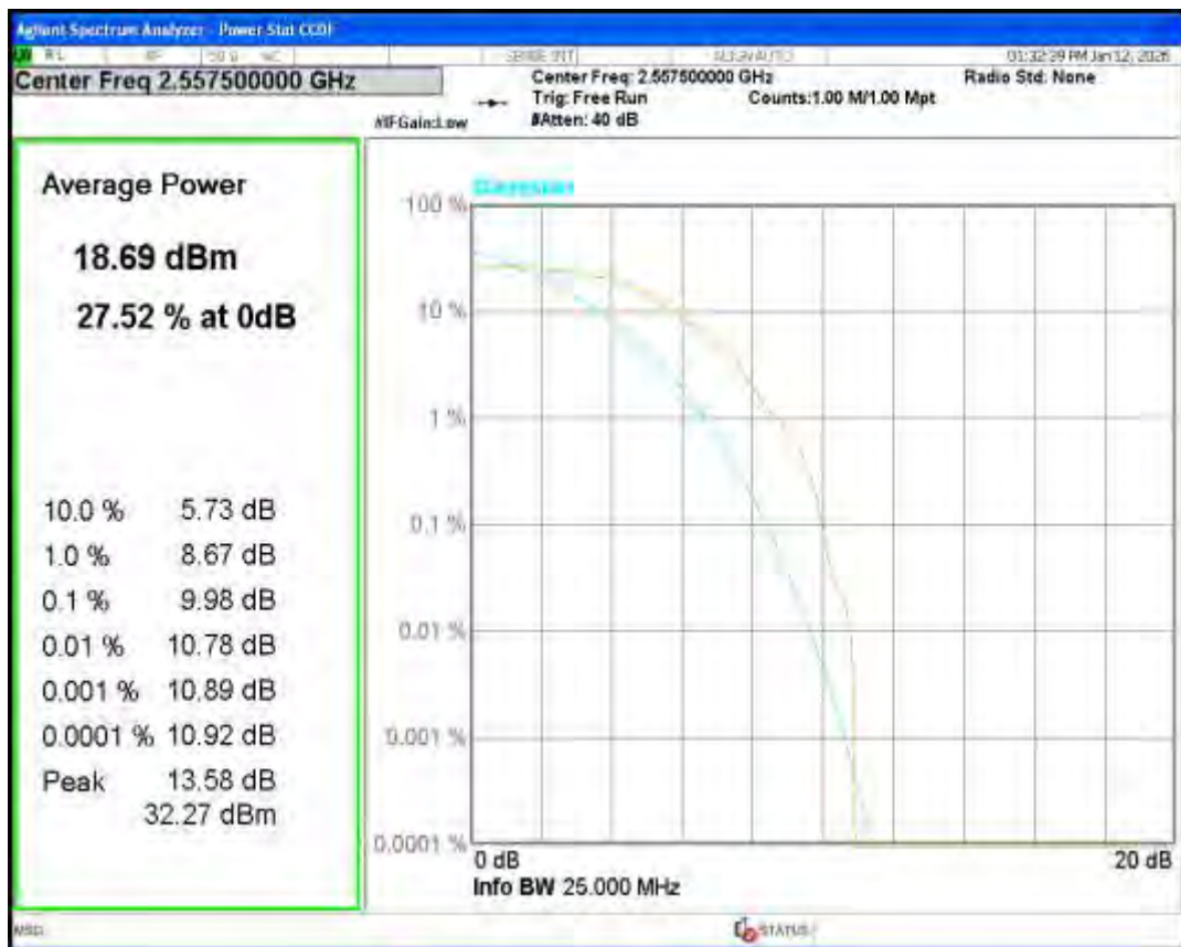
Band41(2555-2655) QPSK BW=5MHz Channel=40740 RB Size=1 Position=#0
