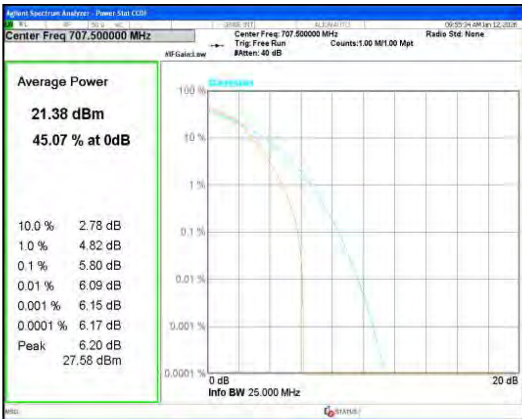
Band12 16QAM BW=5MHz Channel=23155 RB Size=1 Position=#0
