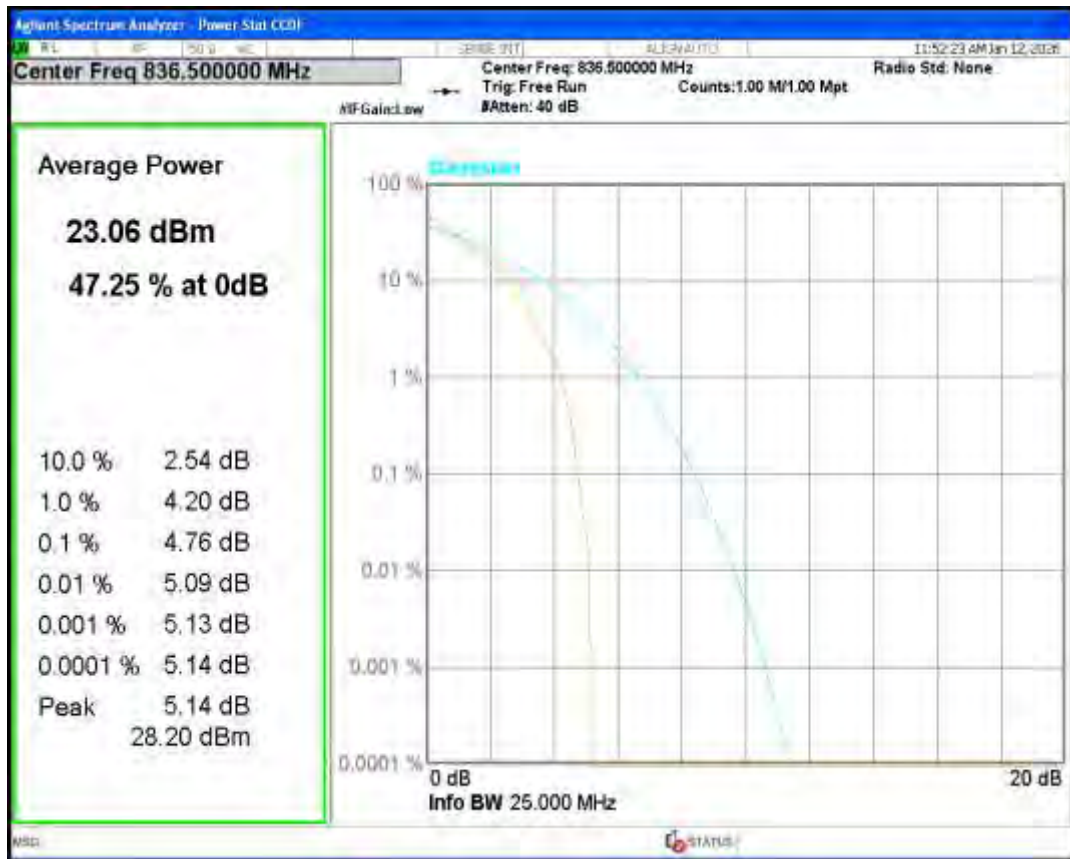
Band26(824-849) QPSK BW=5MHz Channel=27015 RB Size=1 Position=#0
