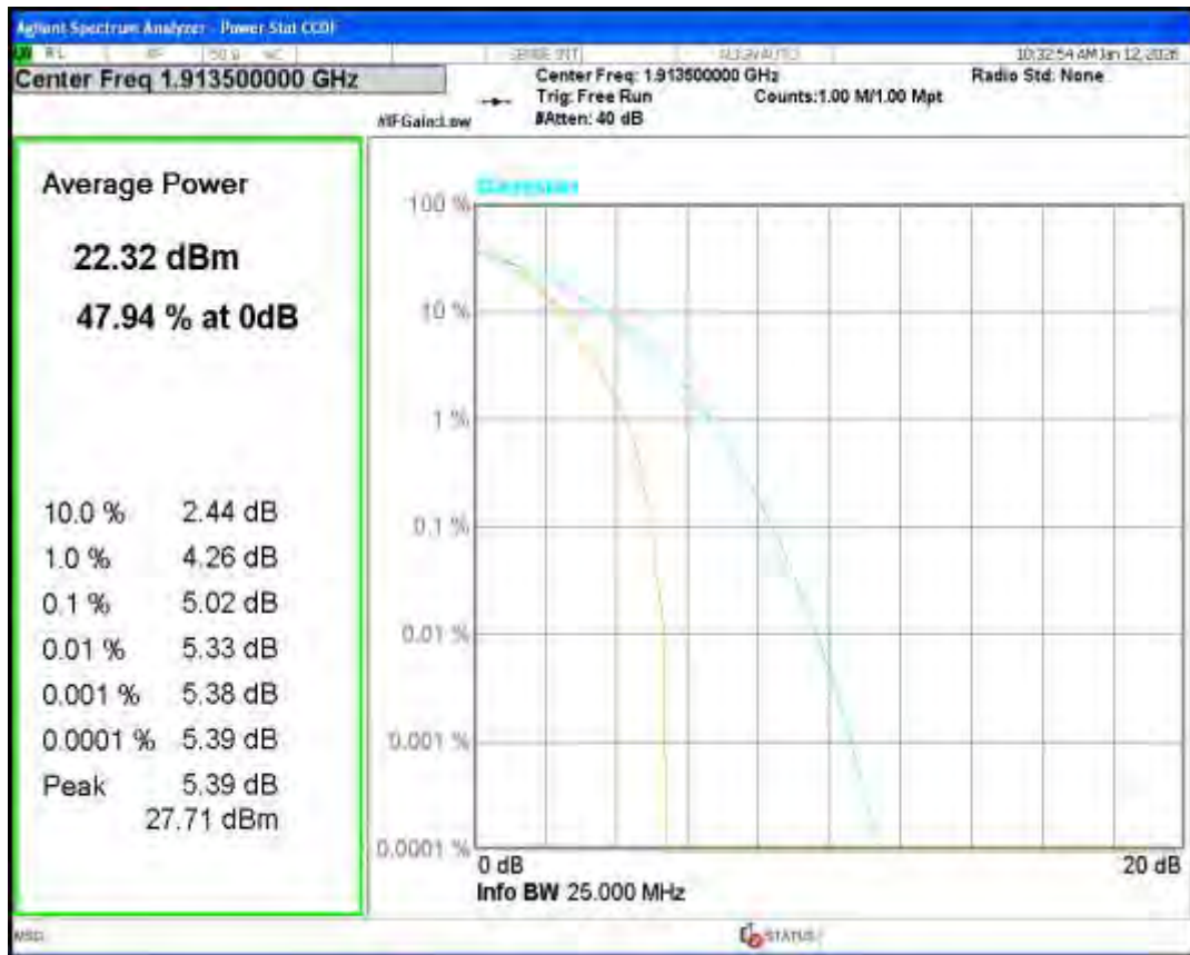
Band25 QPSK BW=5MHz Channel=26065 RB Size=1 Position=#0
