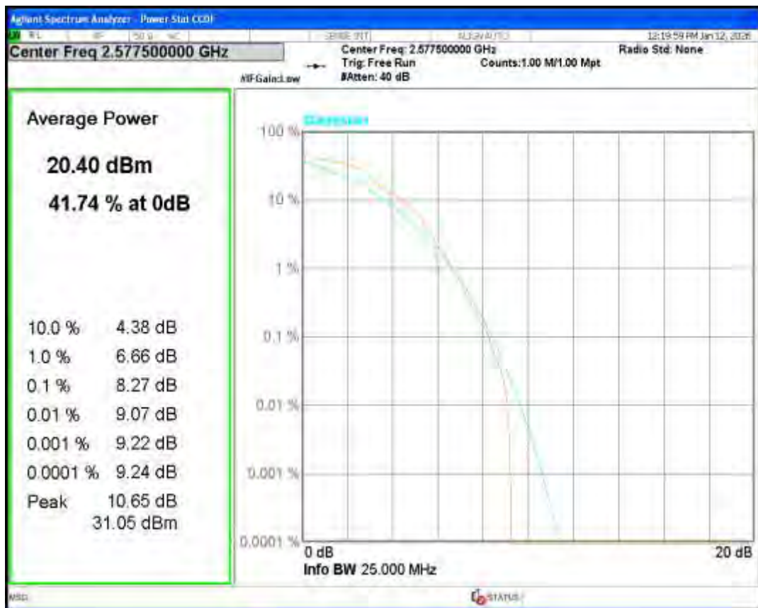
Band38 QPSK BW=15MHz Channel=38000 RB Size=1 Position=#0
