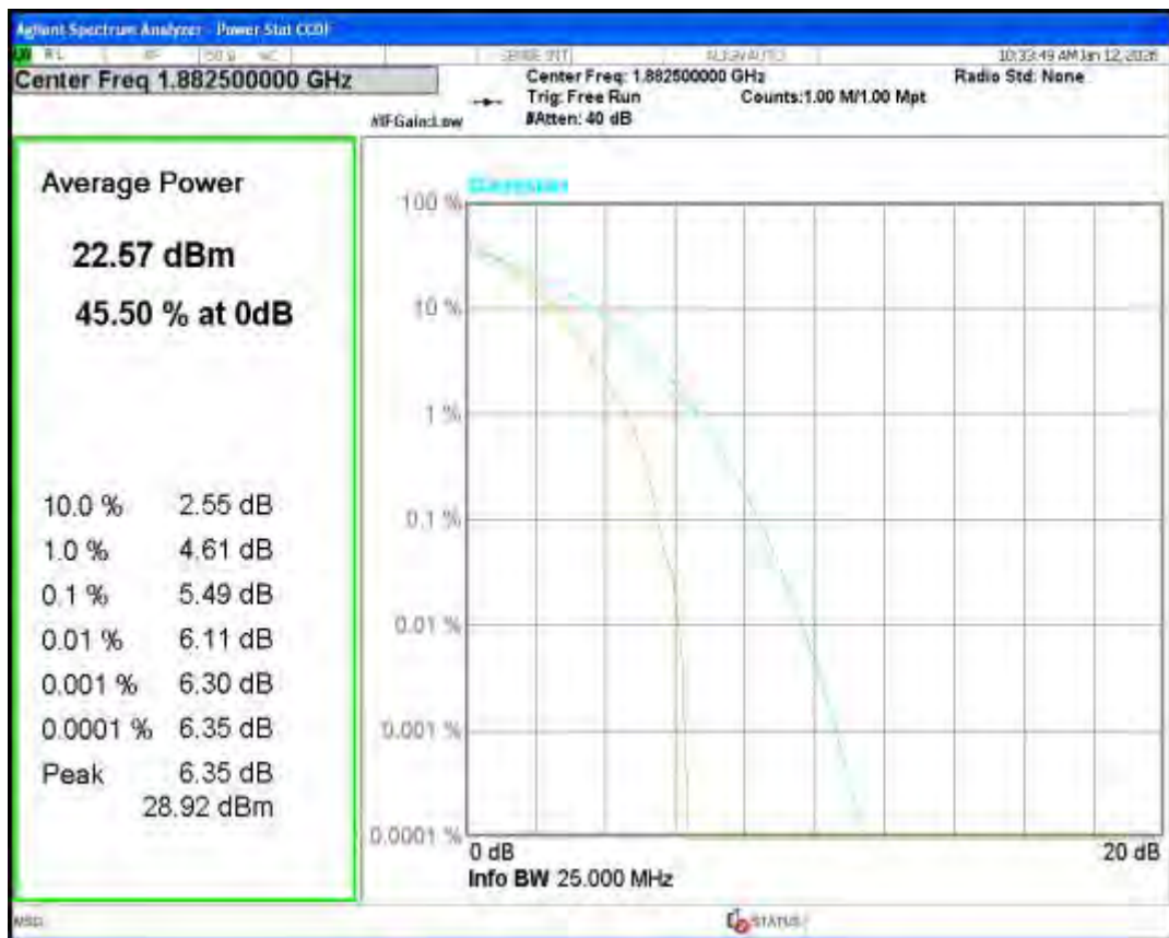
Band25 QPSK BW=20MHz Channel=26590 RB Size=1 Position=#0
