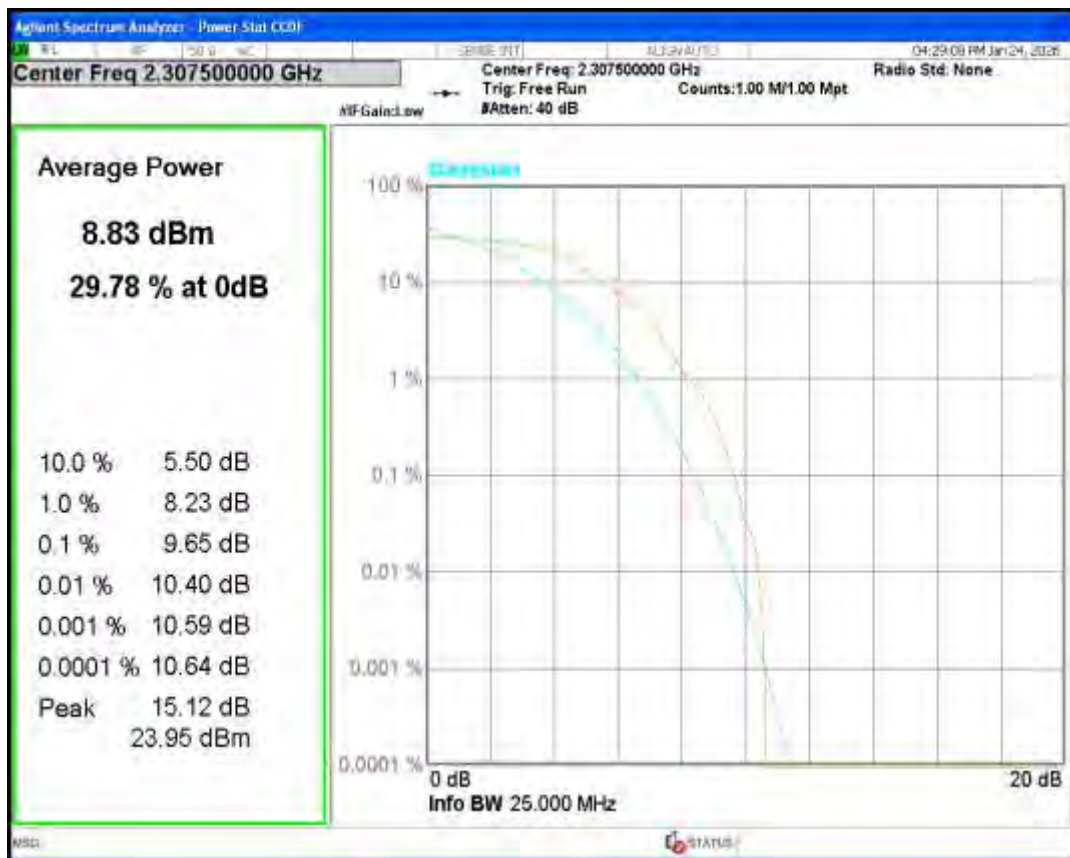
Band40(2305-2315) QPSK BW=5MHz Channel=38750 RB Size=1 Position=#0
