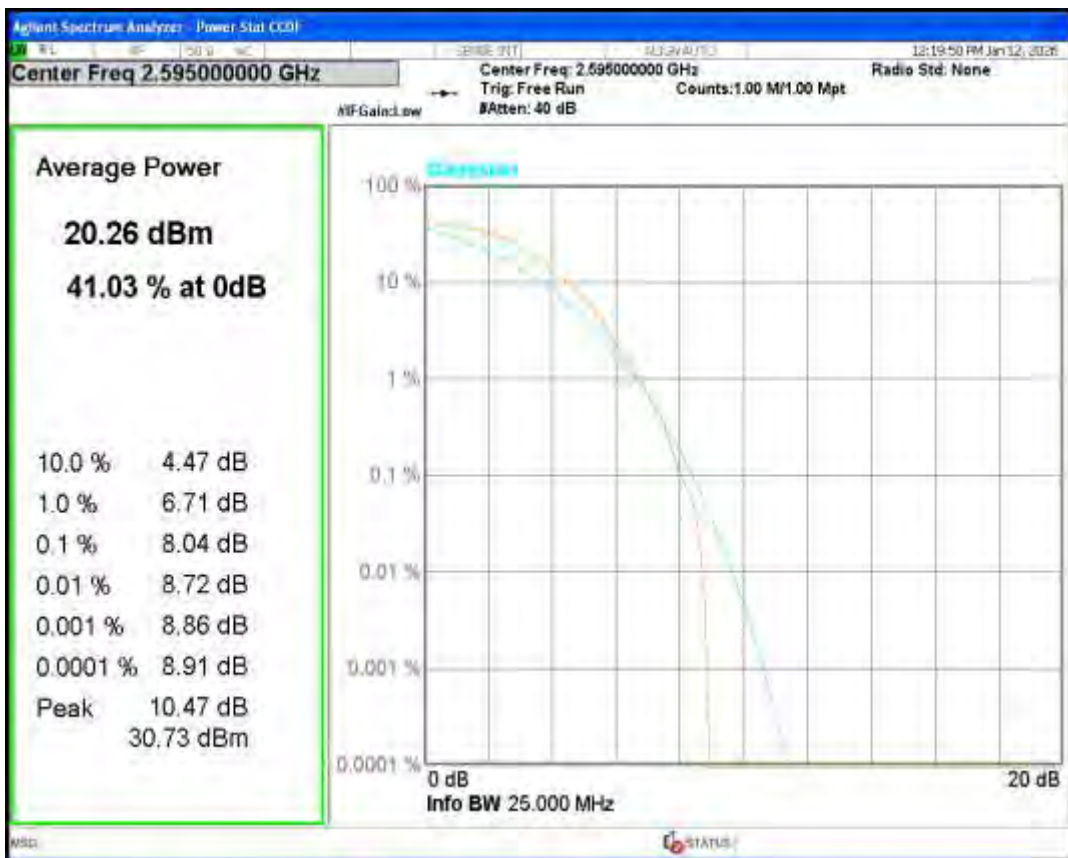
Band38 QPSK BW=10MHz Channel=38200 RB Size=1 Position=#0
