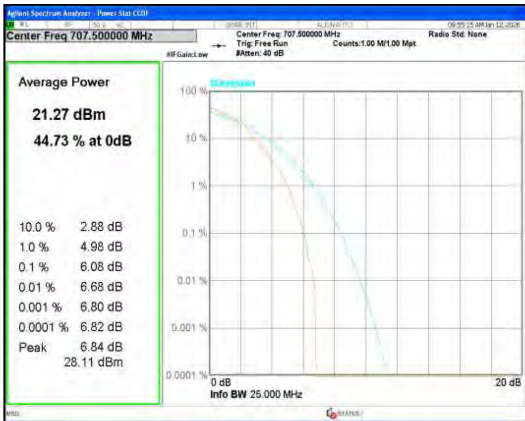
Band12 16QAM BW=3MHz Channel=23165 RB Size=1 Position=#0
