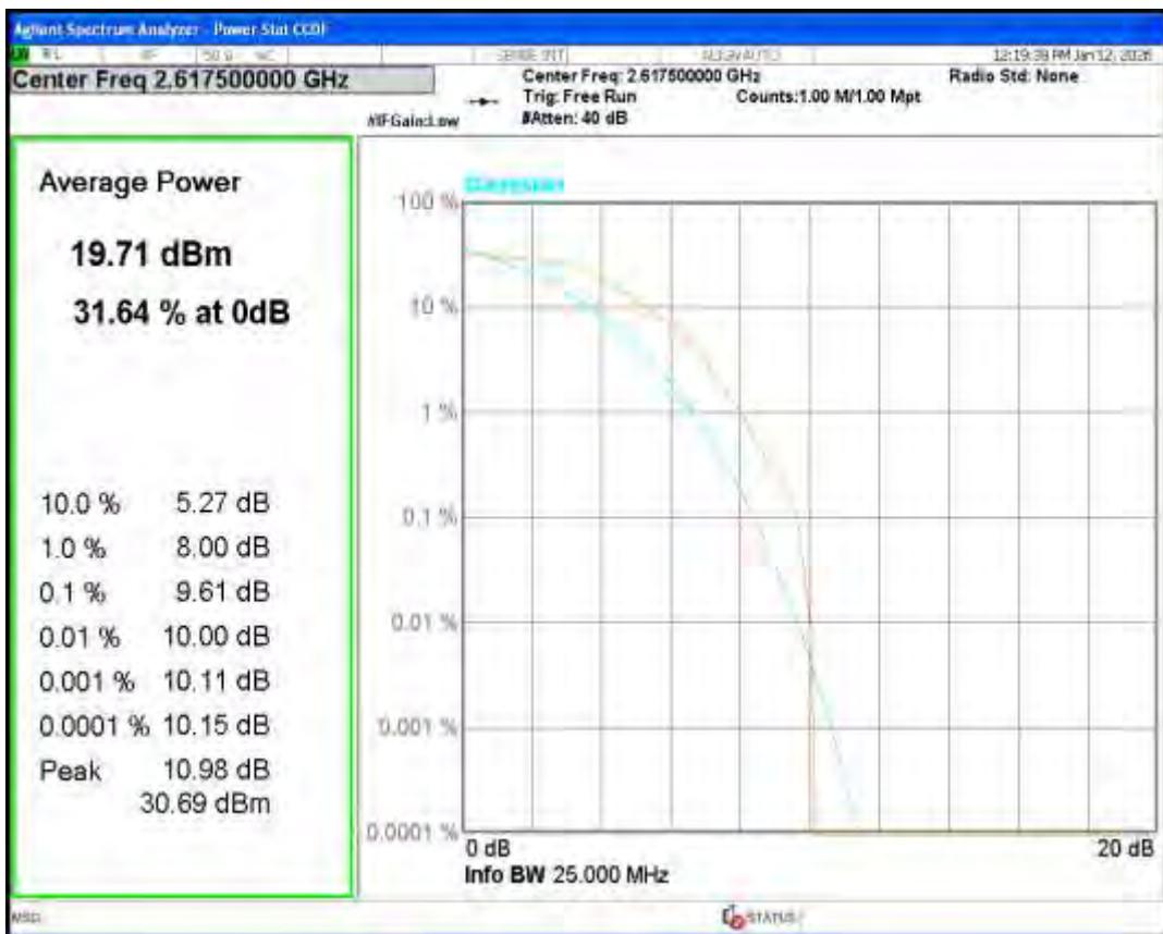
Band38 QPSK BW=10MHz Channel=37800 RB Size=1 Position=#0
