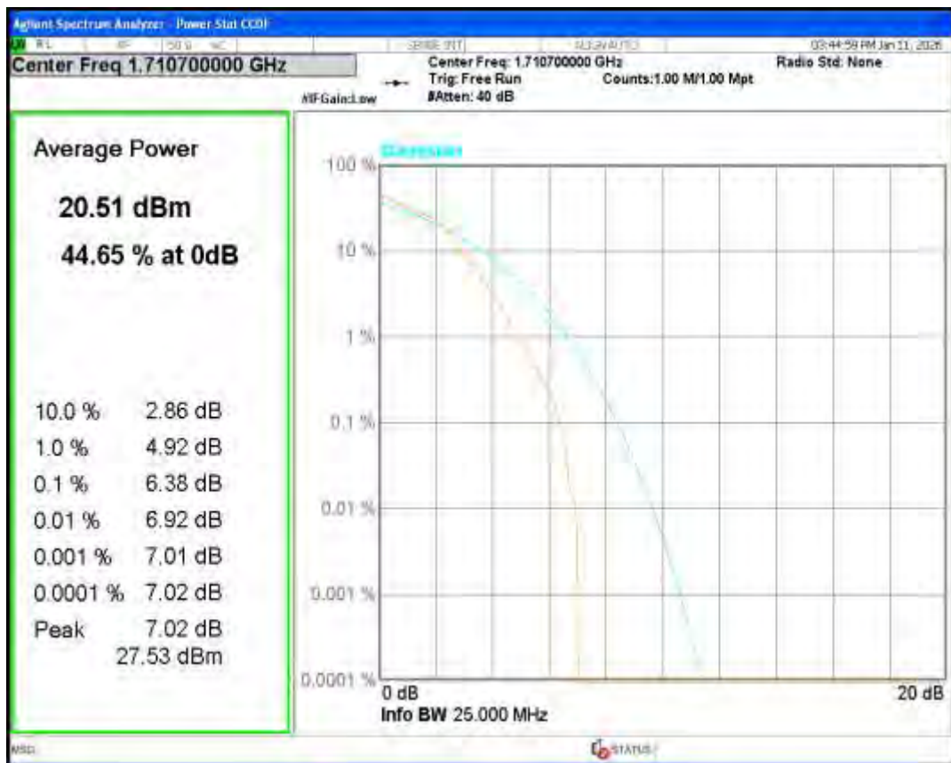
Band4 16QAM BW=1.4MHz Channel=20175 RB Size=1 Position=#0
