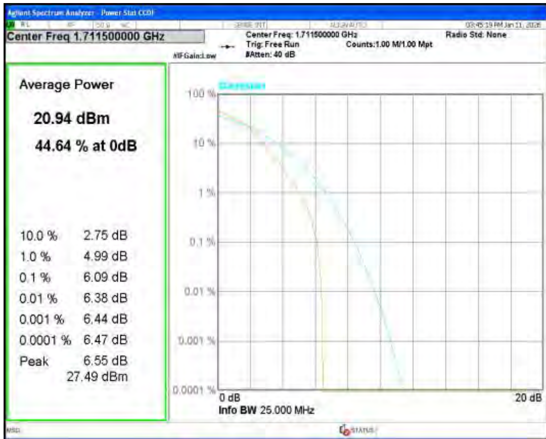
Band4 16QAM BW=3MHz Channel=20175 RB Size=1 Position=#0
