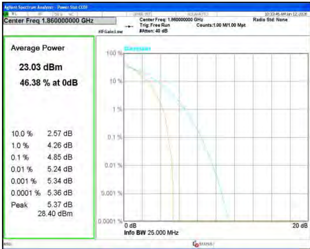
Band25 QPSK BW=20MHz Channel=26365 RB Size=1 Position=#0
