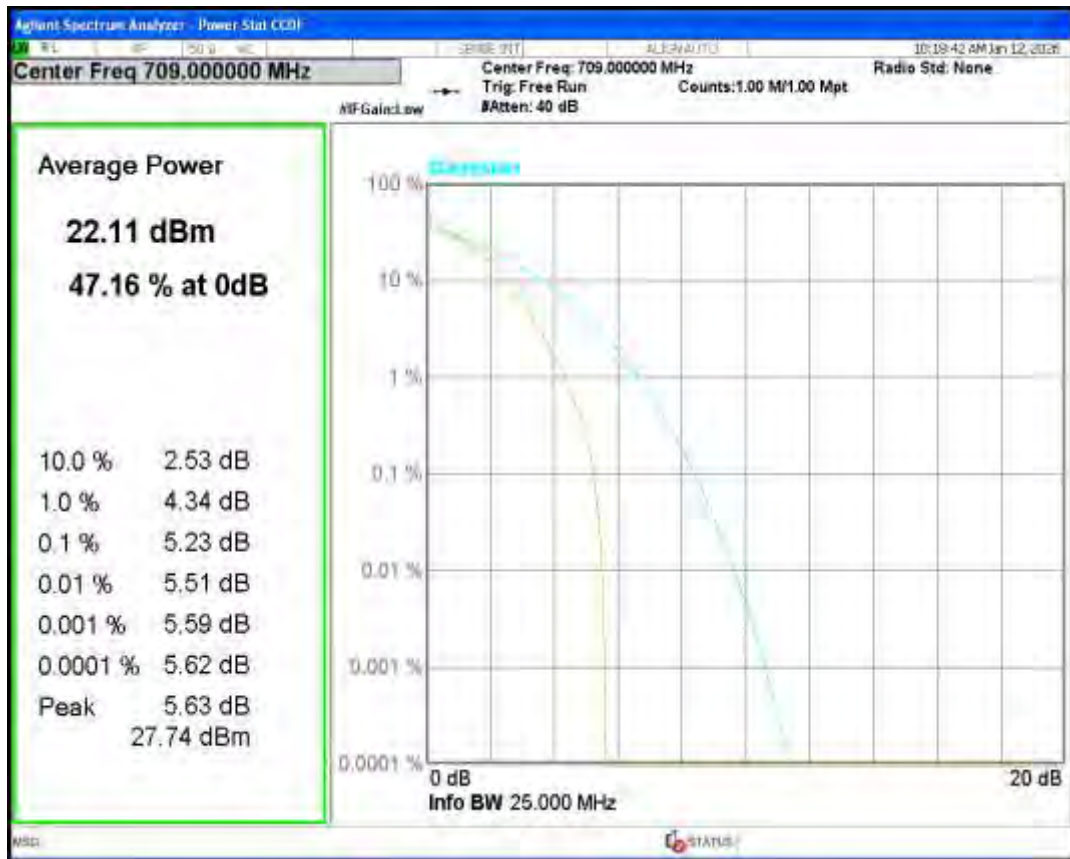
Band17 QPSK BW=10MHz Channel=23790 RB Size=1 Position=#0
