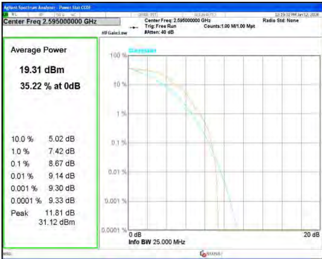
Band38 QPSK BW=5MHz Channel=38225 RB Size=1 Position=#0
