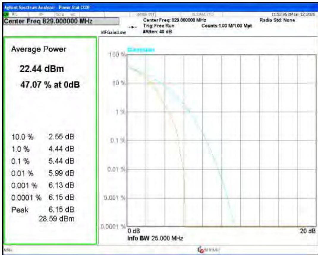
Band26(824-849) QPSK BW=10MHz Channel=26915 RB Size=1 Position=#0
