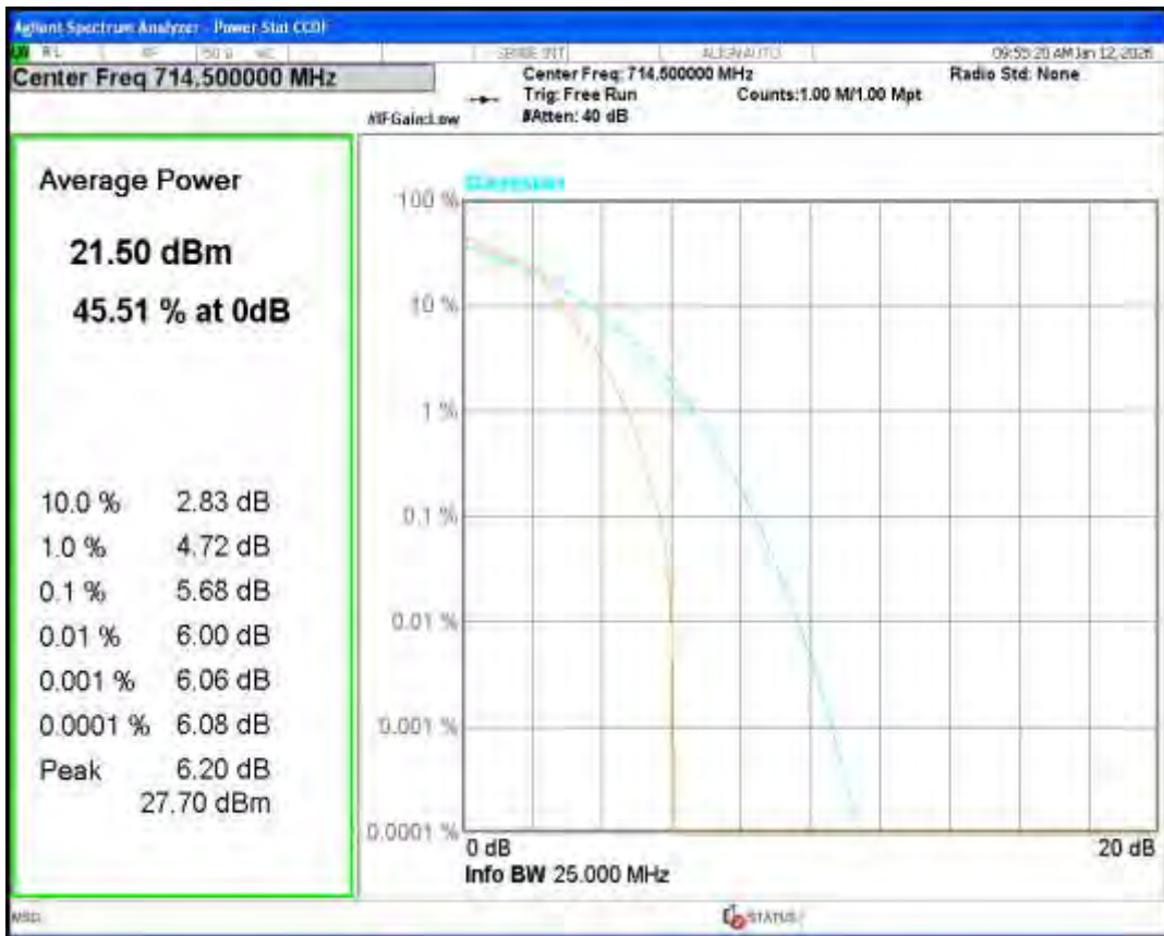
Band12 16QAM BW=5MHz Channel=23095 RB Size=1 Position=#0
