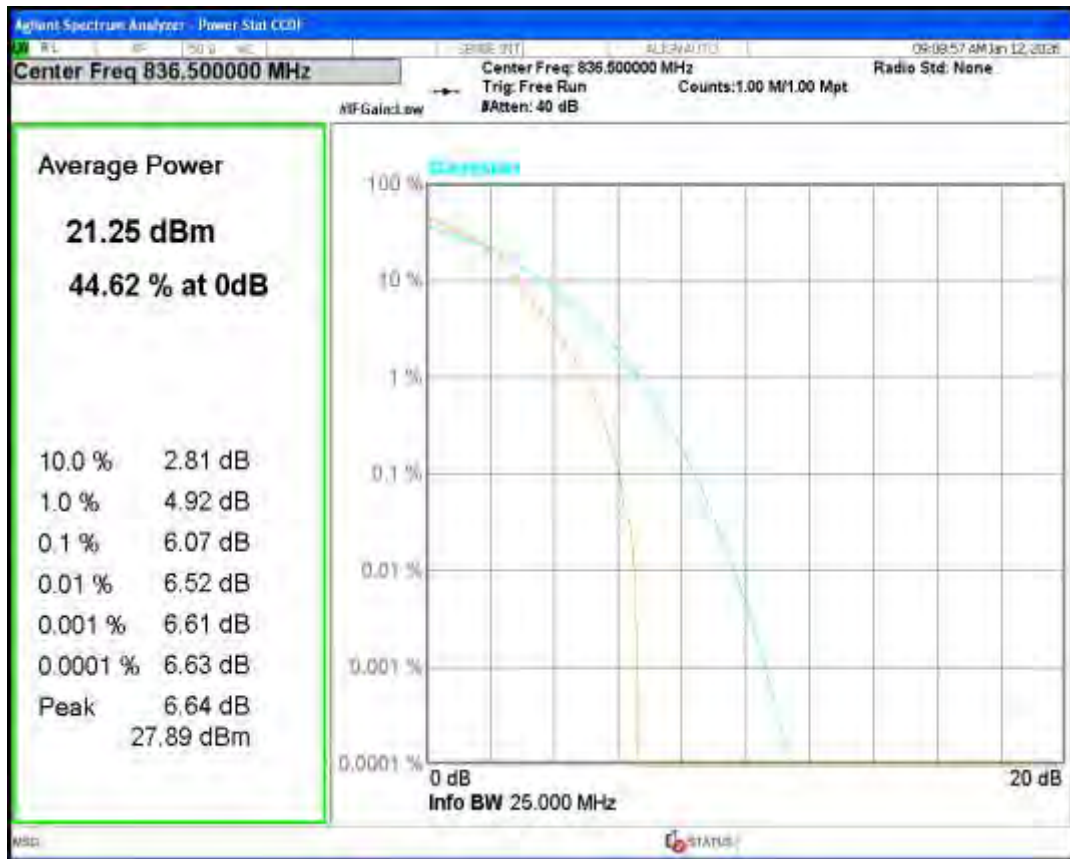
Band5 16QAM BW=1.4MHz Channel=20643 RB Size=1 Position=#0
