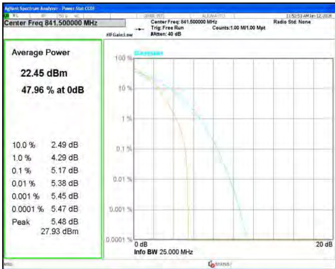
Band38 16QAM BW=5MHz Channel=37775 RB Size=1 Position=#0
