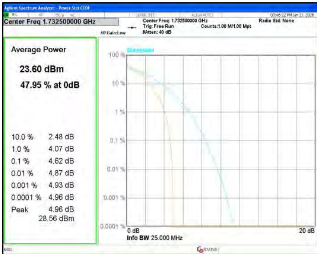
Band4 QPSK BW=15MHz Channel=20325 RB Size=1 Position=#0
