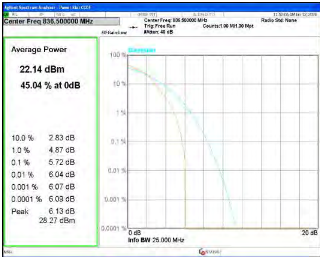
Band26(824-849) 16QAM BW=3MHz Channel=27025 RB Size=1 Position=#0
