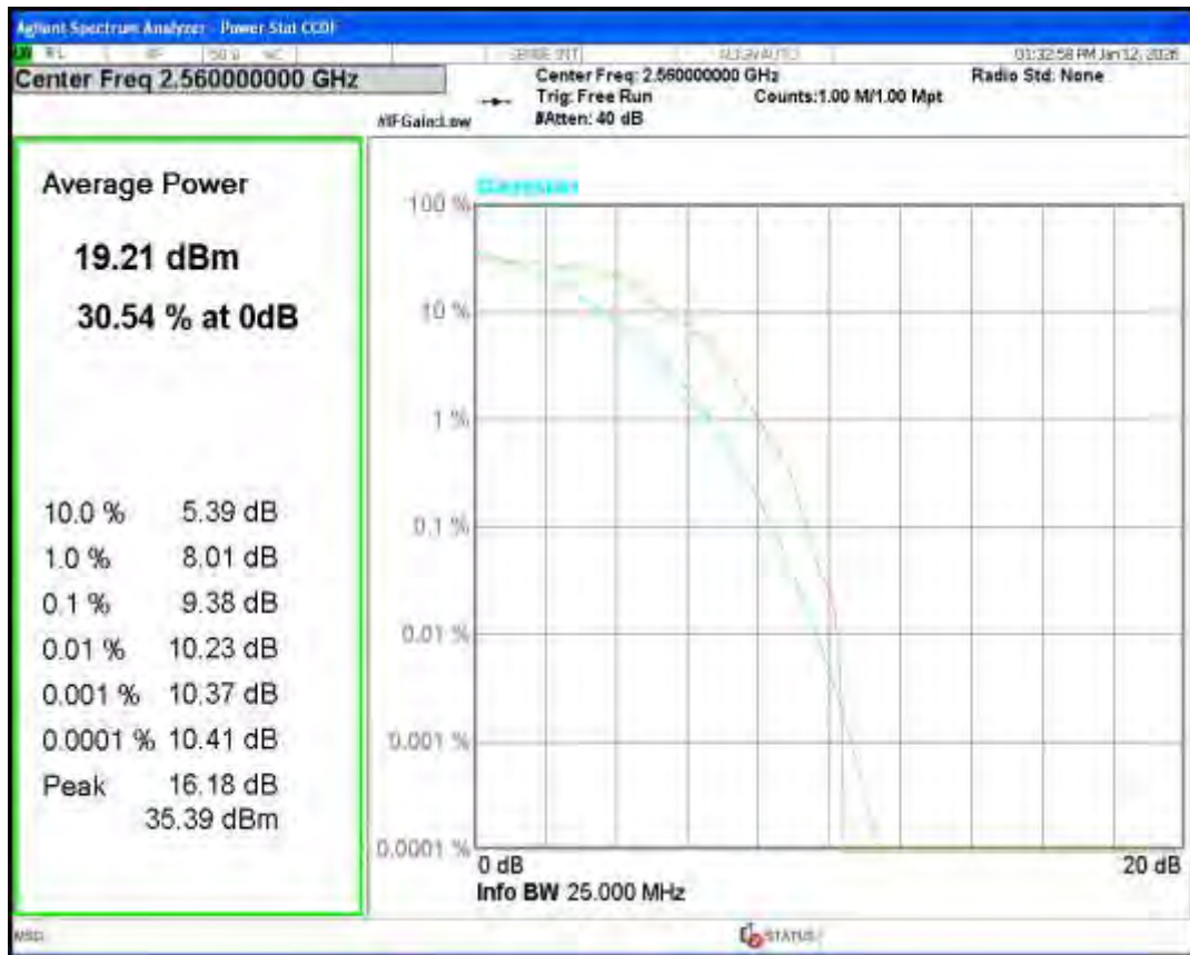
Band41(2555-2655) QPSK BW=10MHz Channel=40740 RB Size=1 Position=#0
