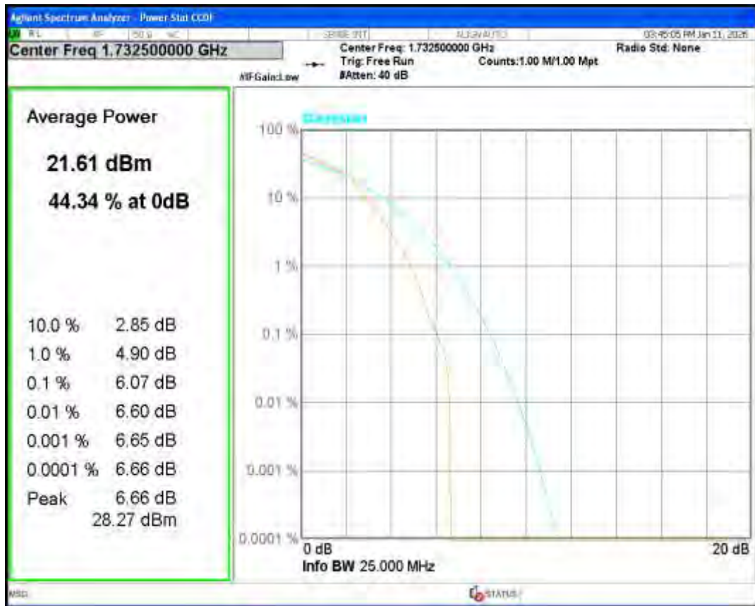
Band4 16QAM BW=1.4MHz Channel=20393 RB Size=1 Position=#0
