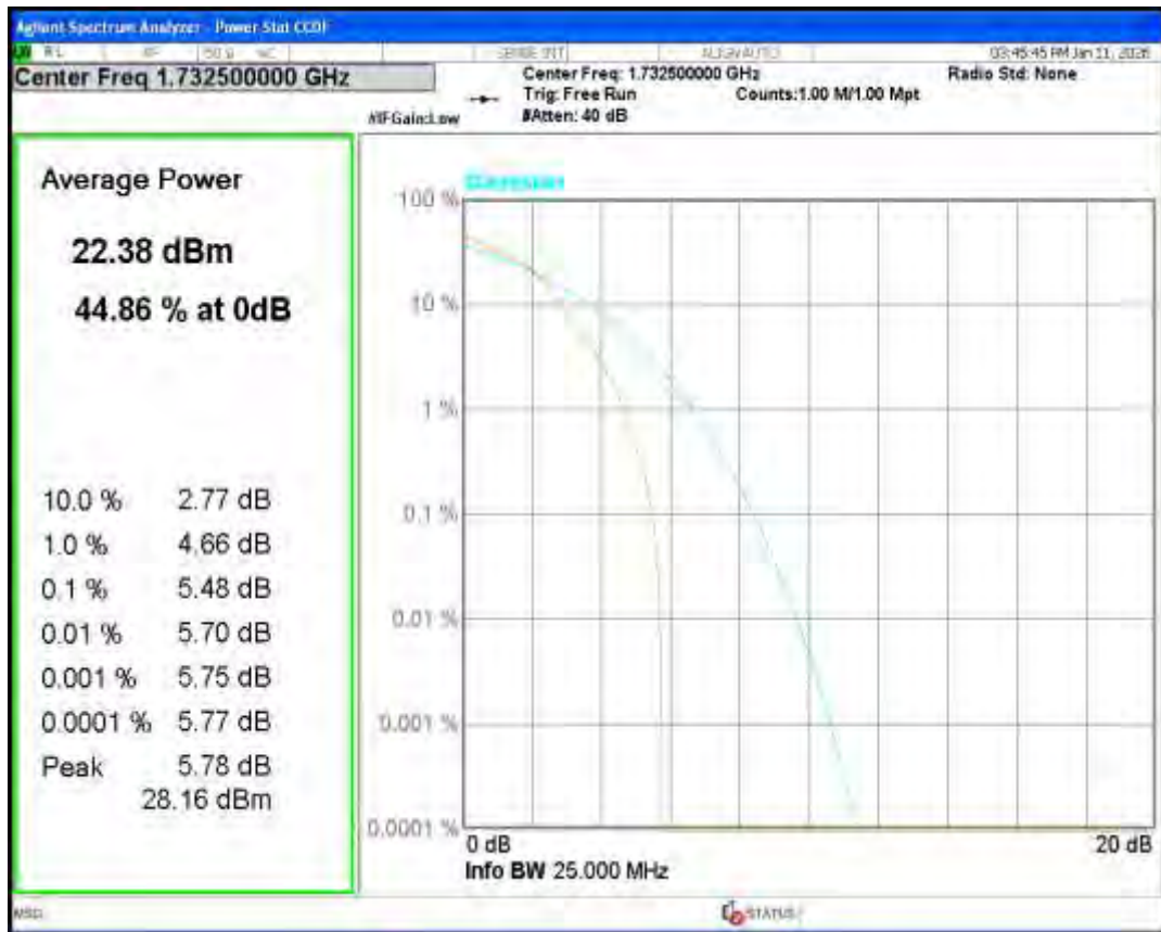
Band4 16QAM BW=5MHz Channel=20375 RB Size=1 Position=#0
