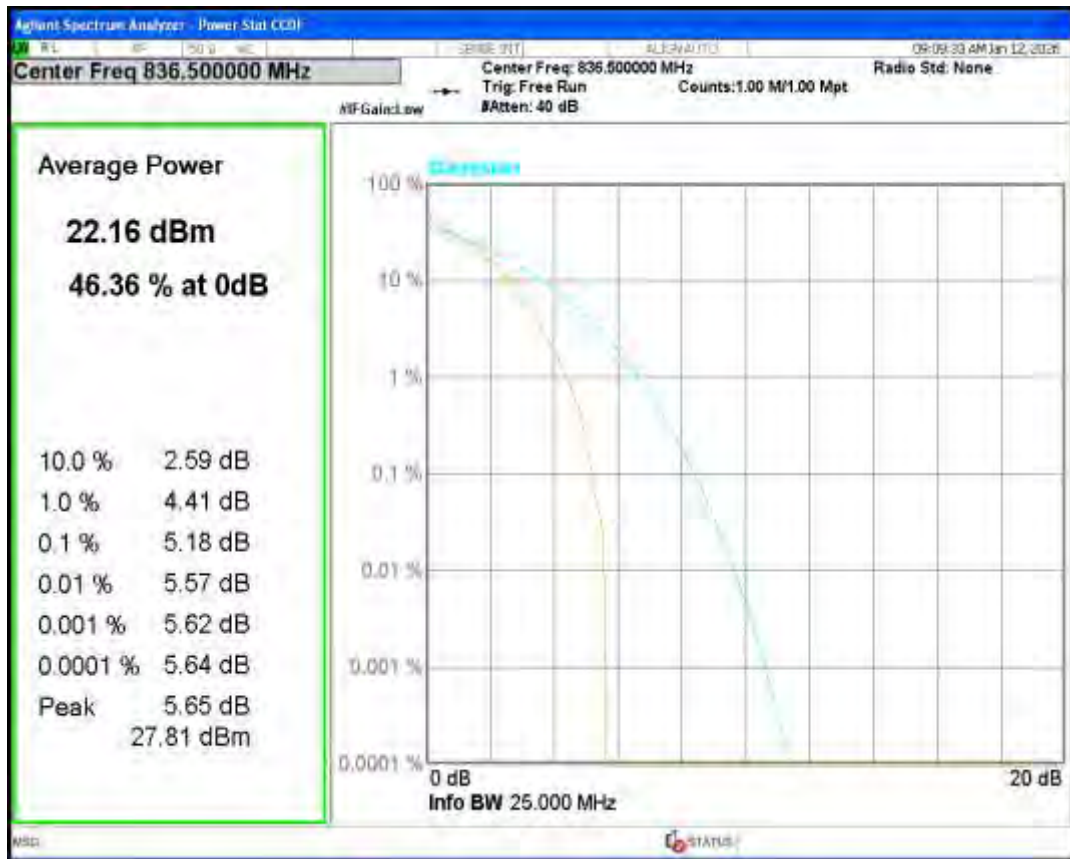
Band5 QPSK BW=5MHz Channel=20425 RB Size=1 Position=#0
