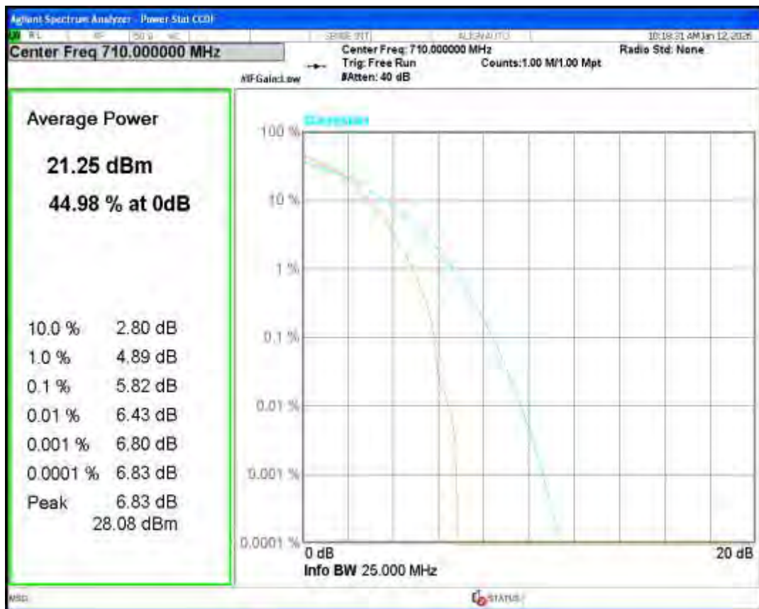
Band17 16QAM BW=5MHz Channel=23825 RB Size=1 Position=#0
