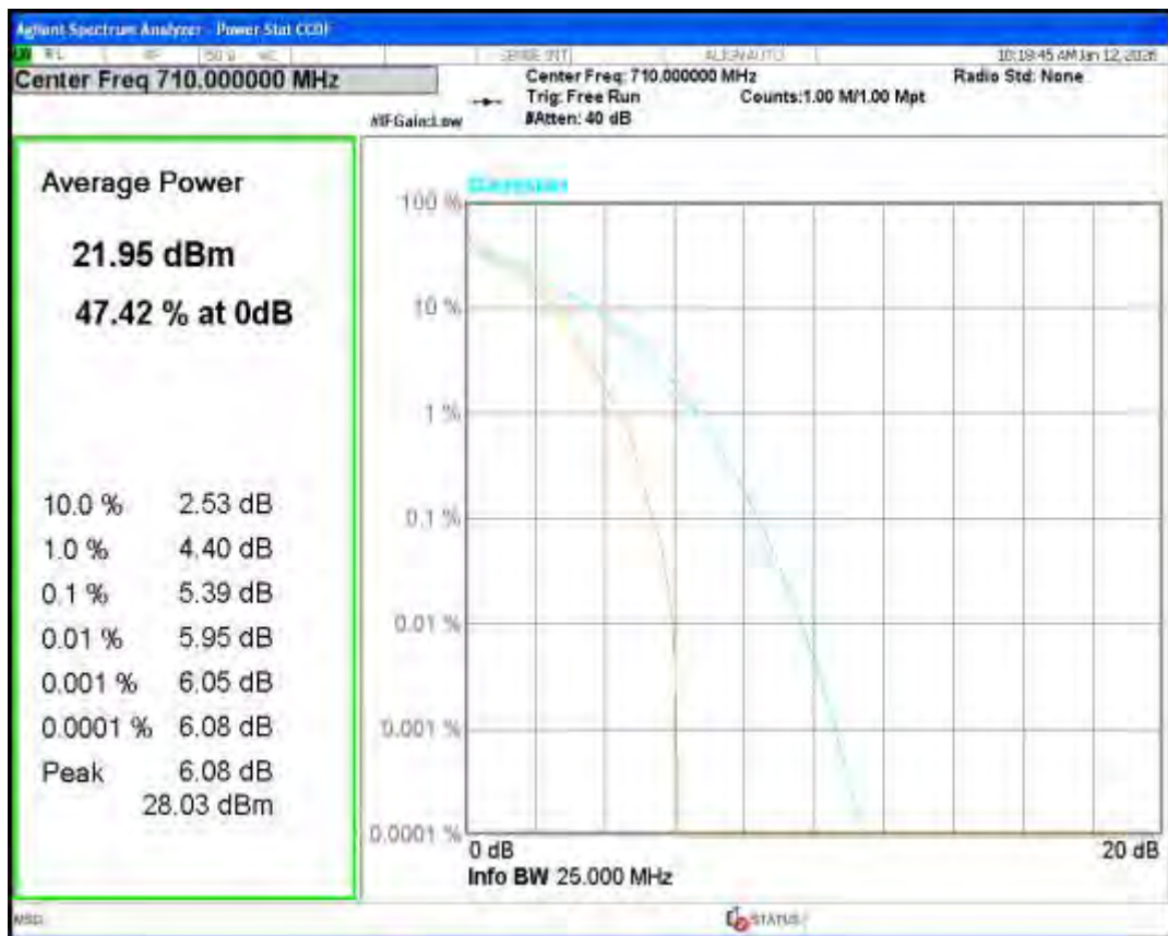
Band17 QPSK BW=10MHz Channel=23800 RB Size=1 Position=#0
