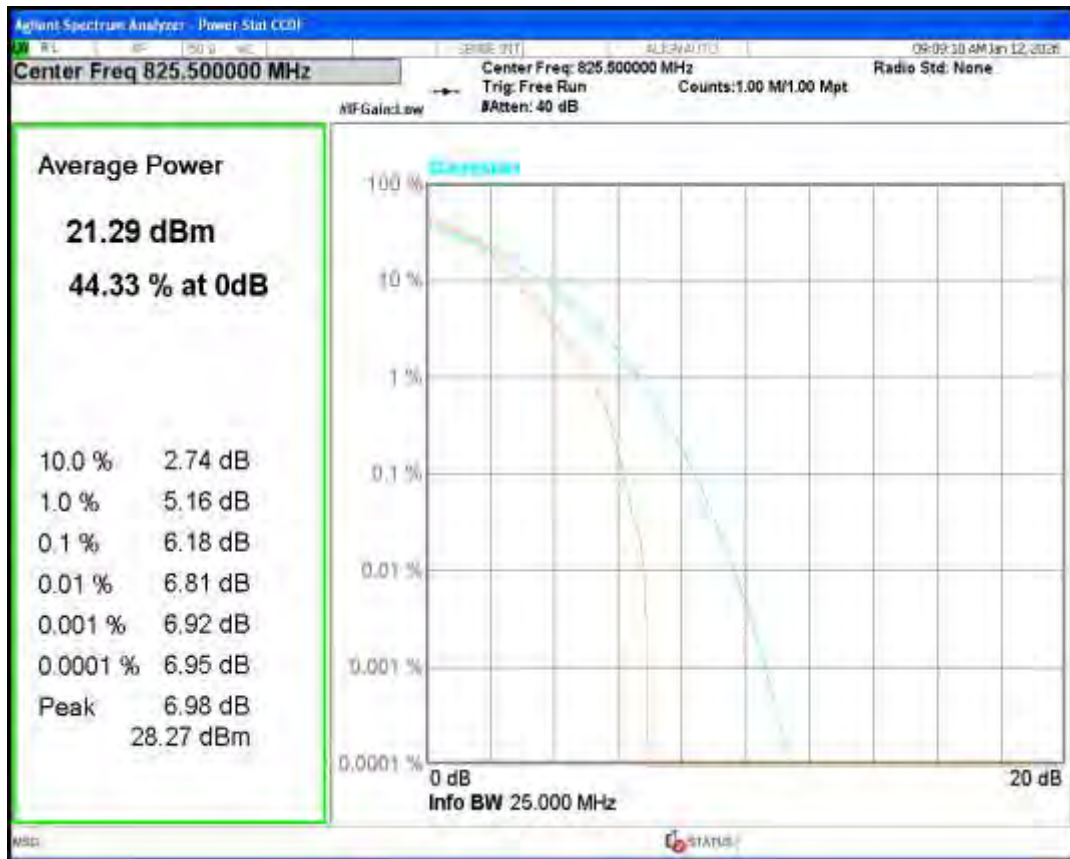
Band5 16QAM BW=3MHz Channel=20525 RB Size=1 Position=#0
