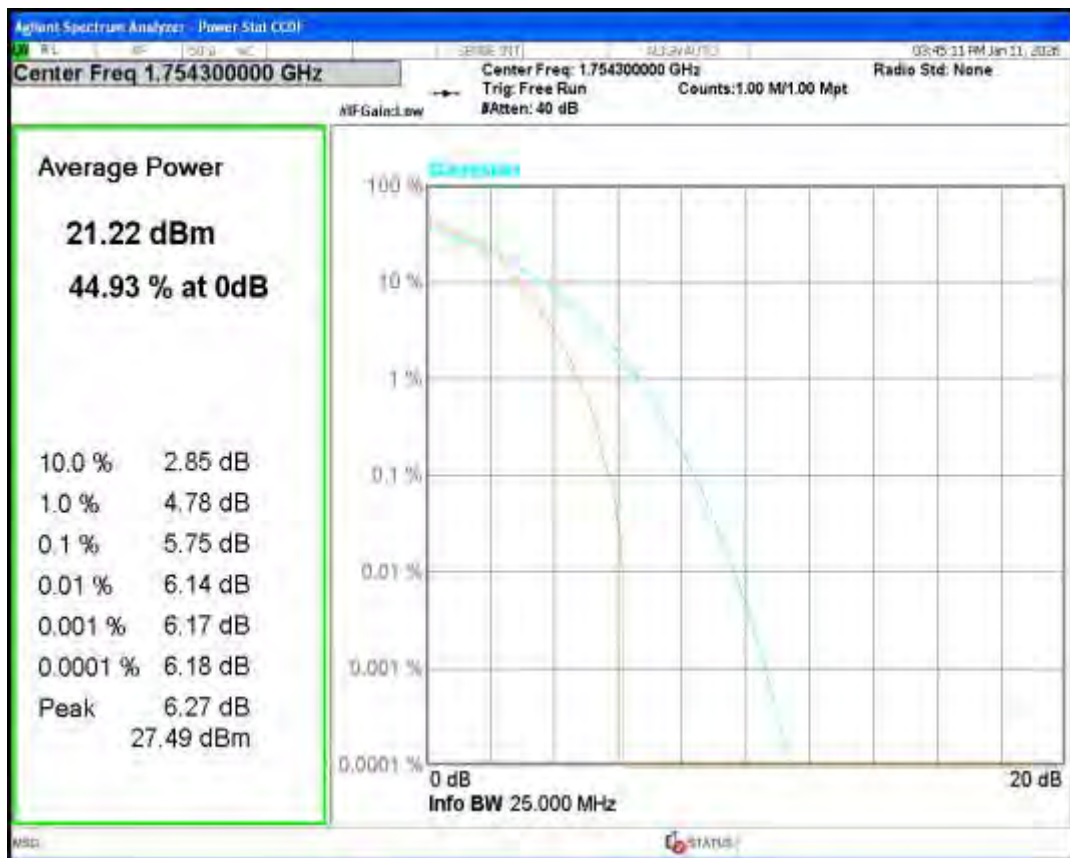
Band4 16QAM BW=3MHz Channel=19965 RB Size=1 Position=#0
