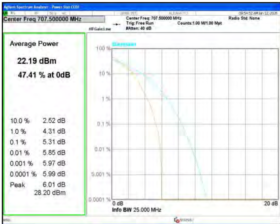
Band12 QPSK BW=1.4MHz Channel=23173 RB Size=1 Position=#0
