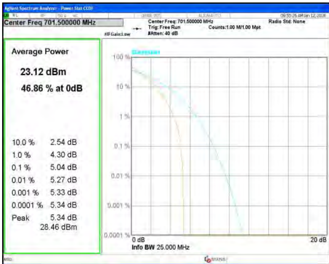
Band12 QPSK BW=5MHz Channel=23155 RB Size=1 Position=#0
