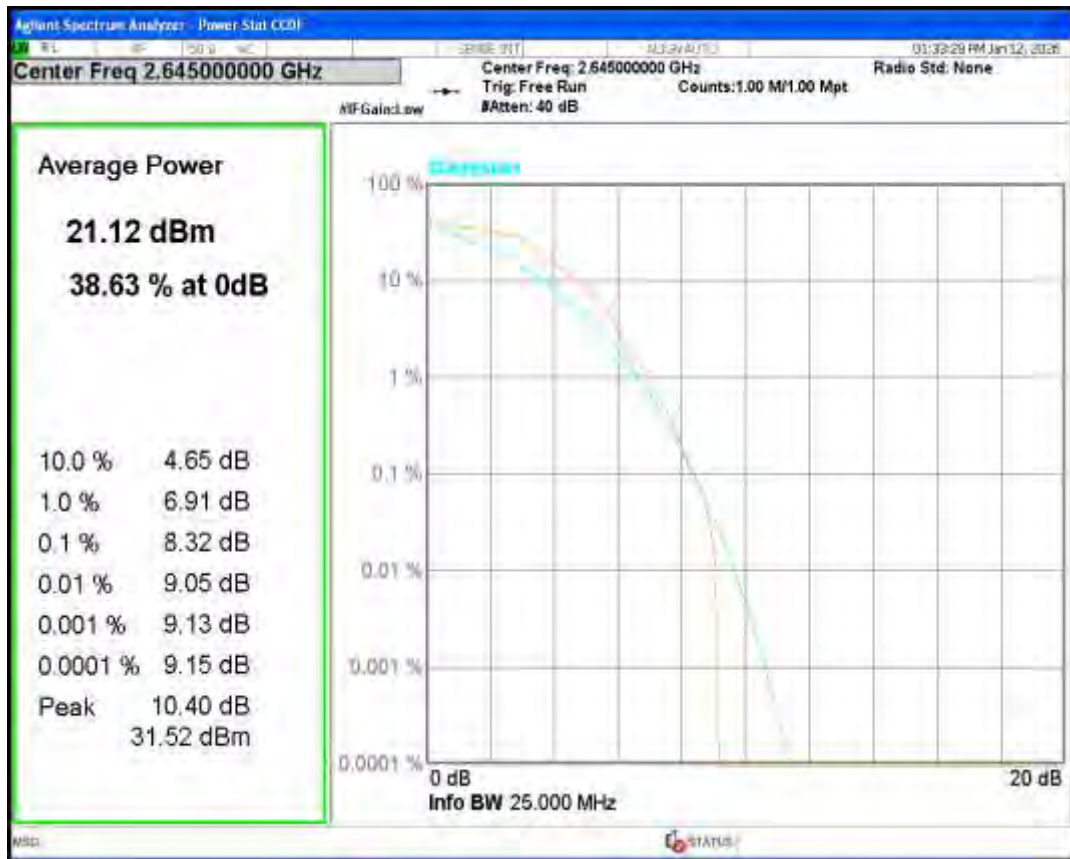
Band5 16QAM BW=1.4MHz Channel=20407 RB Size=1 Position=#0
