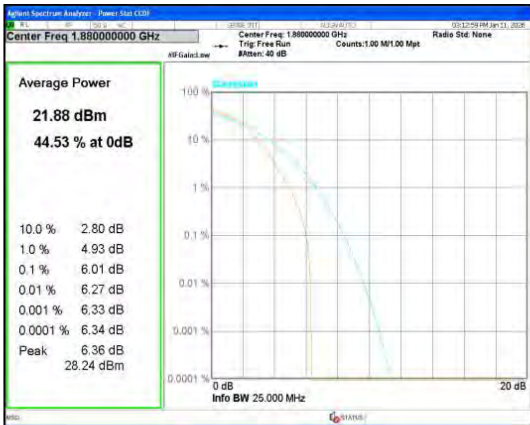
Band2 QPSK BW=1.4MHz Channel=18607 RB Size=1 Position=#0
