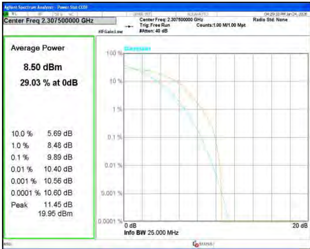
Band40(2305-2315) 16QAM BW=5MHz Channel=38750 RB Size=1 Position=#0
