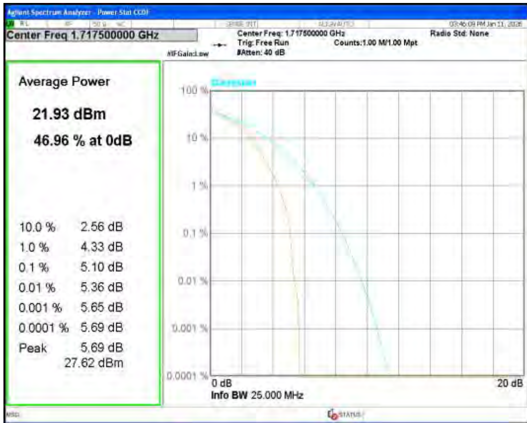
Band4 QPSK BW=15MHz Channel=20175 RB Size=1 Position=#0
