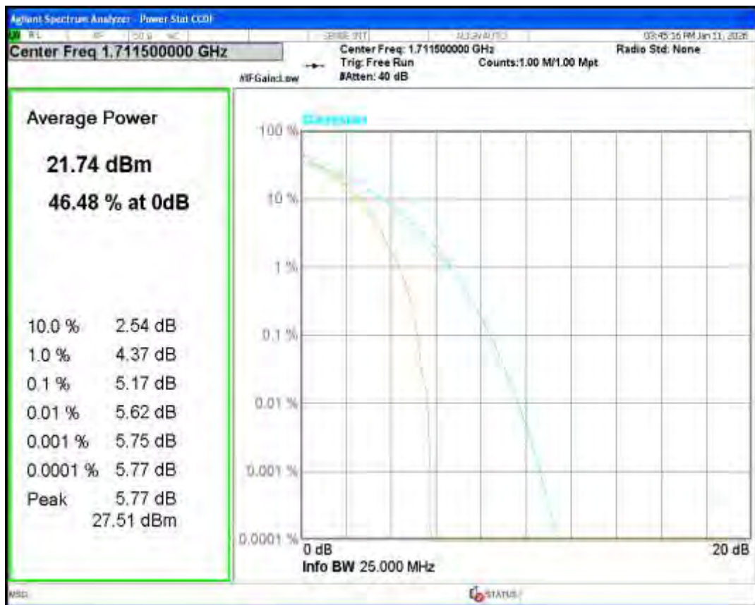
Band4 QPSK BW=3MHz Channel=20175 RB Size=1 Position=#0
