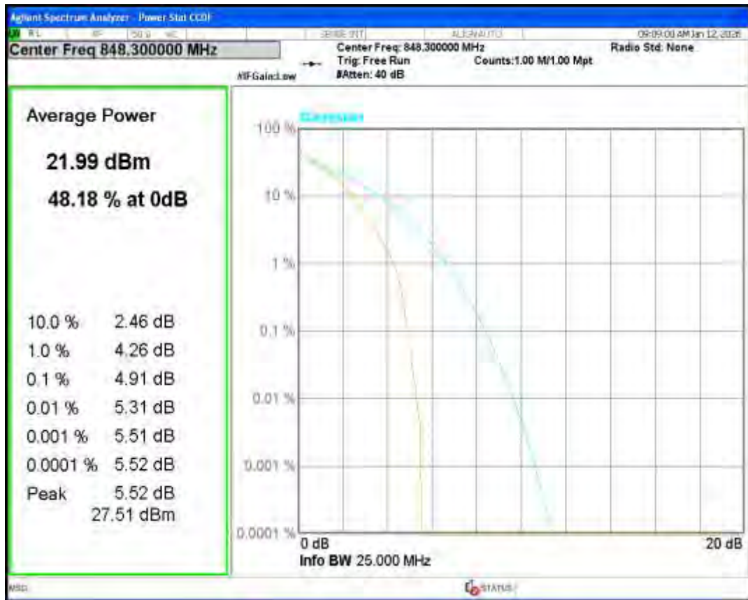
Band5 QPSK BW=3MHz Channel=20415 RB Size=1 Position=#0
