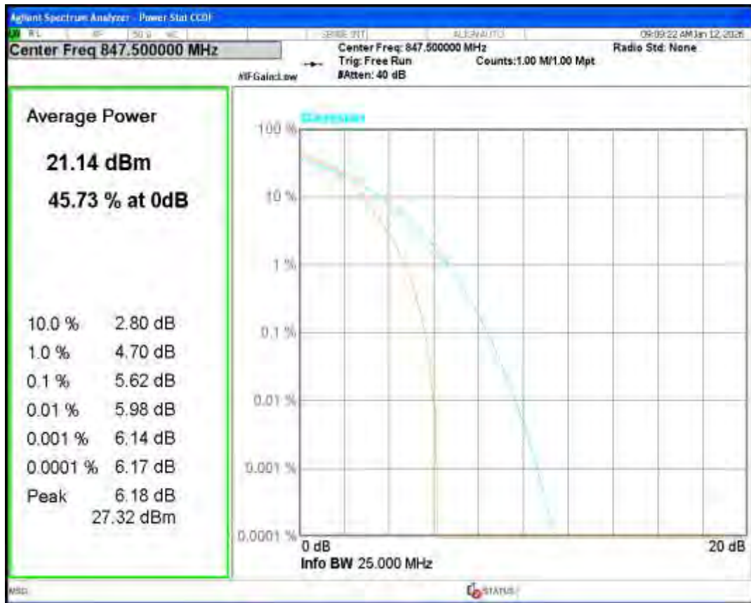
Band5 16QAM BW=5MHz Channel=20425 RB Size=1 Position=#0
