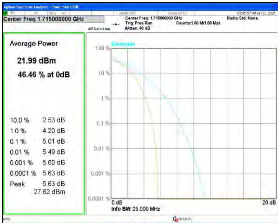
Band4 QPSK BW=10MHz Channel=20175 RB Size=1 Position=#0
