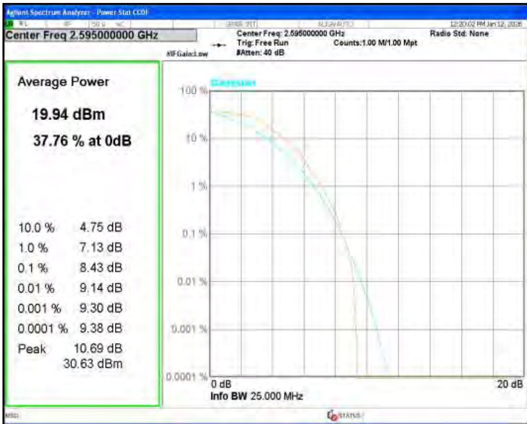
Band38 QPSK BW=15MHz Channel=38175 RB Size=1 Position=#0
