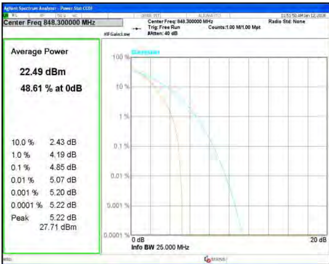
Band26(824-849) QPSK BW=3MHz Channel=26805 RB Size=1 Position=#0
