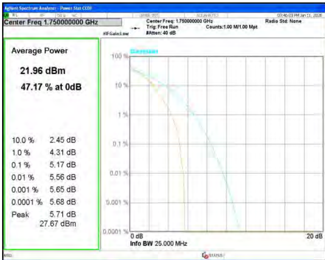
Band4 QPSK BW=15MHz Channel=20025 RB Size=1 Position=#0
