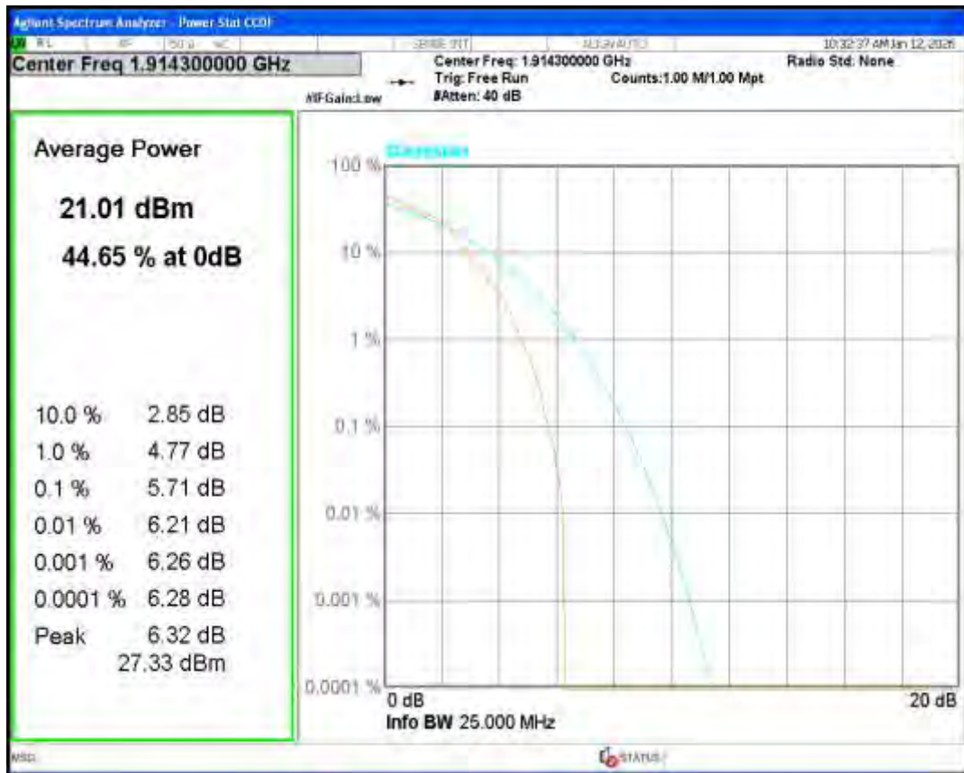
Band25 16QAM BW=3MHz Channel=26055 RB Size=1 Position=#0
