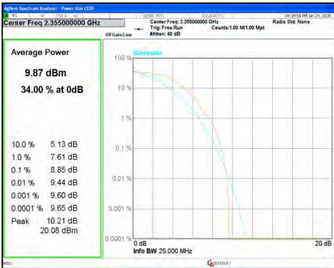
Band40(2350-2360) QPSK BW=5MHz Channel=39225 RB Size=1 Position=#0
