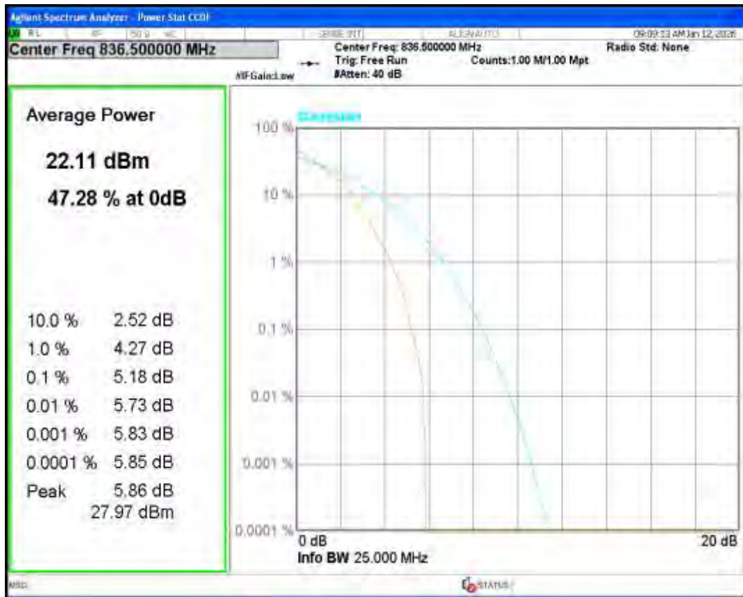
Band5 QPSK BW=3MHz Channel=20635 RB Size=1 Position=#0
