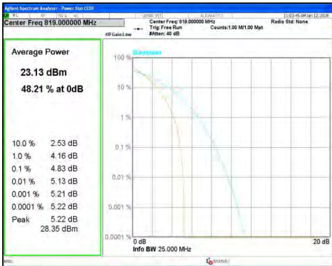
Band26(814-824) QPSK BW=1.4MHz Channel=26783 RB Size=1 Position=#0
