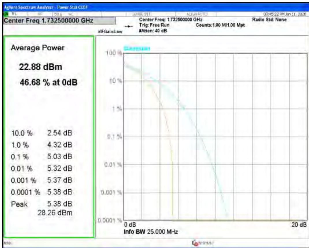
Band4 QPSK BW=3MHz Channel=20385 RB Size=1 Position=#0
