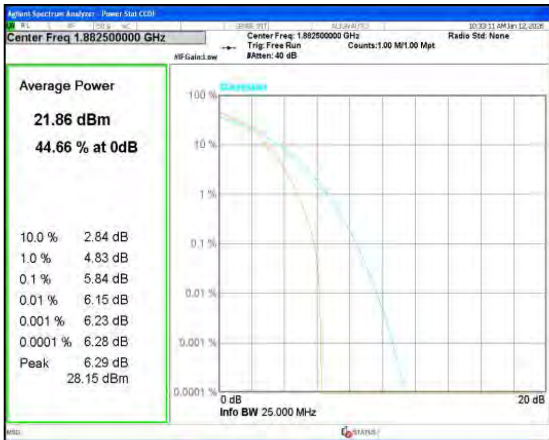
Band25 QPSK BW=1.4MHz Channel=26365 RB Size=1 Position=#0
