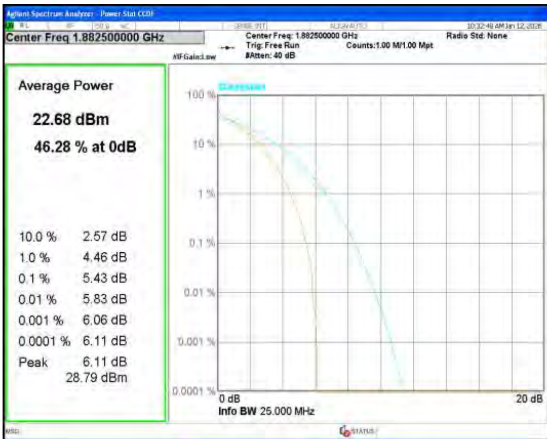
Band25 QPSK BW=3MHz Channel=26675 RB Size=1 Position=#0
