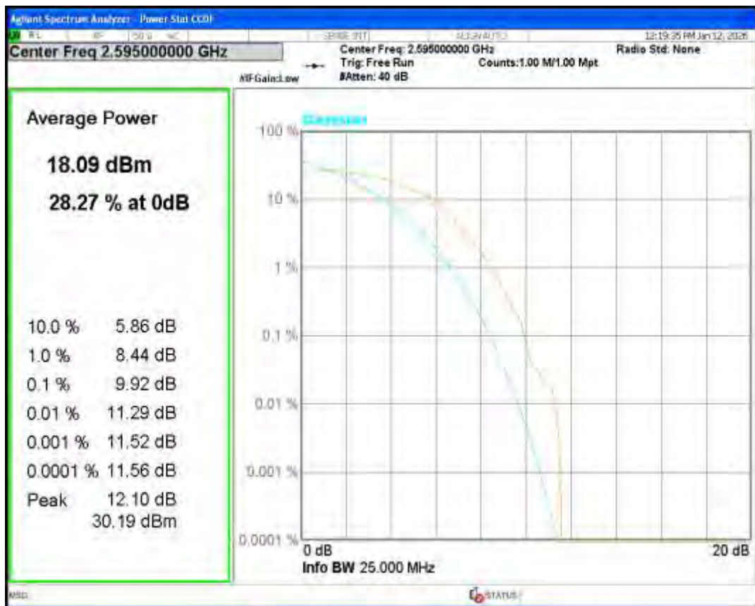
Band38 16QAM BW=5MHz Channel=38225 RB Size=1 Position=#0
