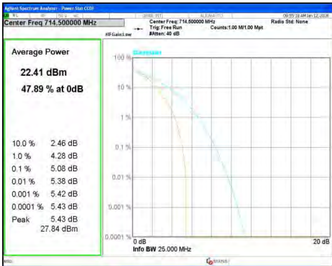
Band12 QPSK BW=5MHz Channel=23095 RB Size=1 Position=#0
