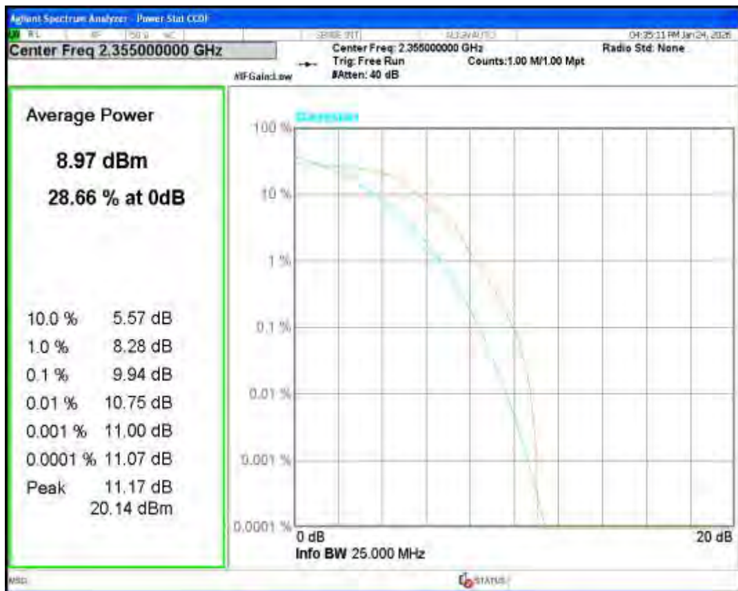
Band41(2555-2655) 16QAM BW=5MHz Channel=40265 RB Size=1 Position=#0
