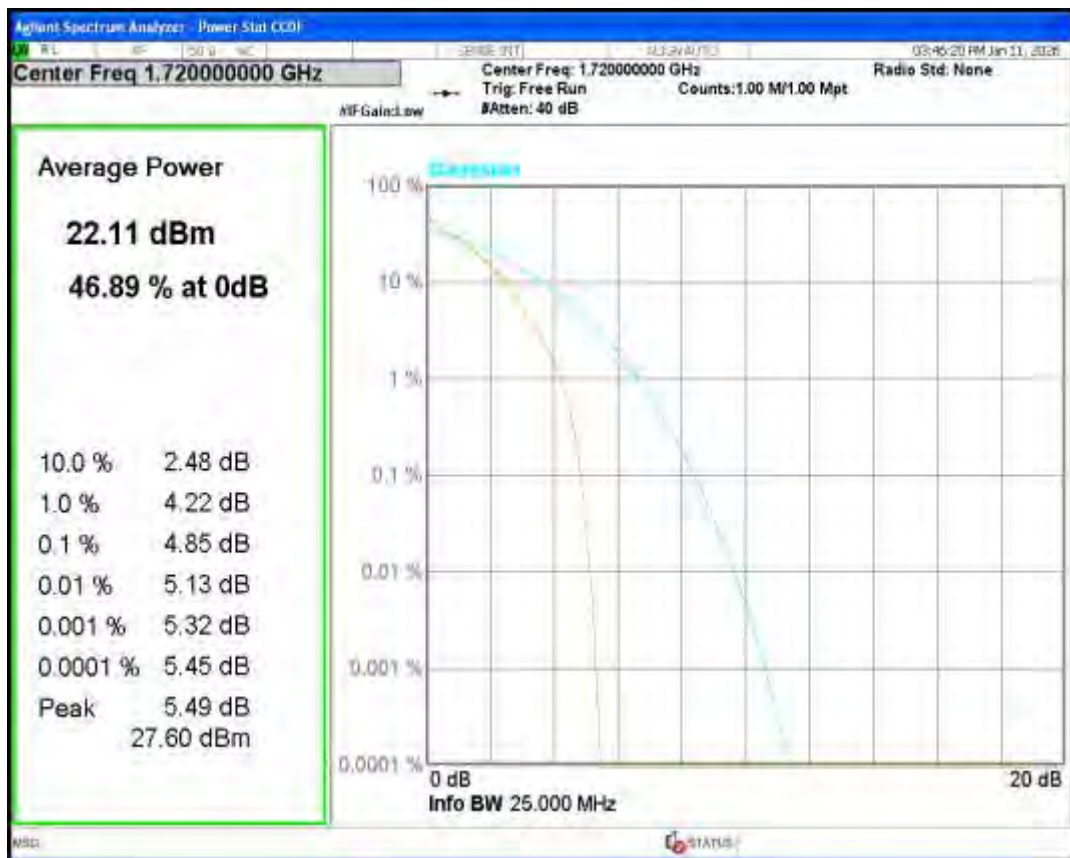
Band4 QPSK BW=20MHz Channel=20175 RB Size=1 Position=#0
