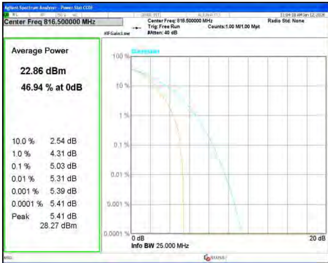
Band26(814-824) QPSK BW=5MHz Channel=26740 RB Size=1 Position=#0
