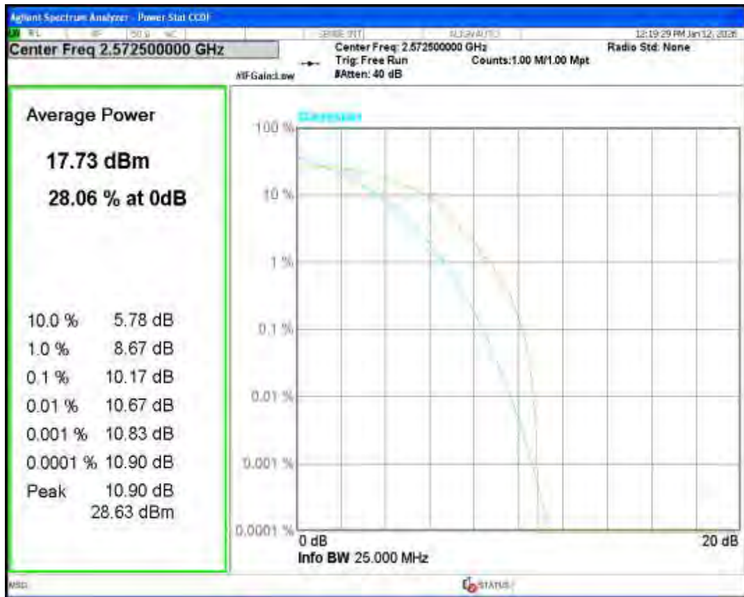
Band38 16QAM BW=5MHz Channel=38000 RB Size=1 Position=#0
