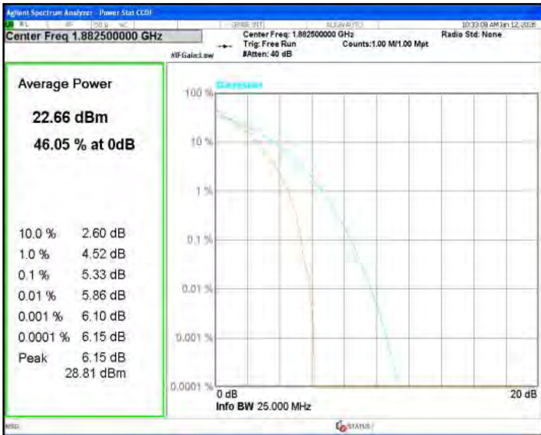
Band25 QPSK BW=5MHz Channel=26665 RB Size=1 Position=#0
