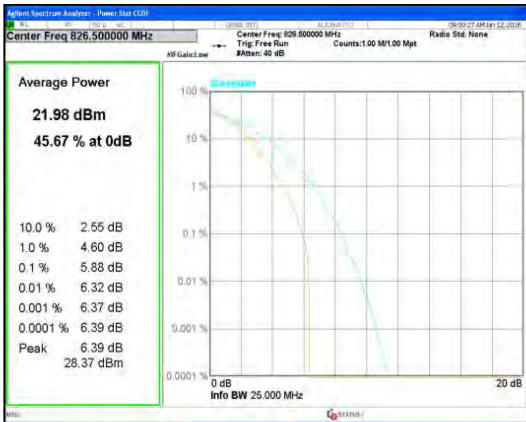
Band5 QPSK BW=5MHz Channel=20625 RB Size=1 Position=#0
