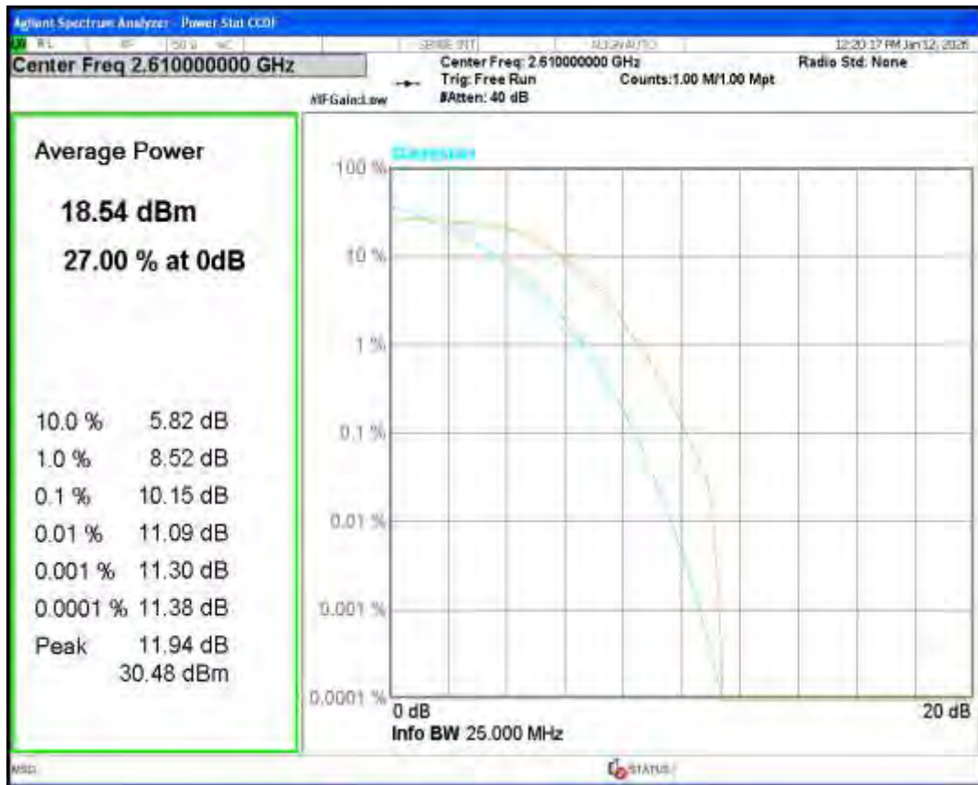
Band4 16QAM BW=1.4MHz Channel=19957 RB Size=1 Position=#0
