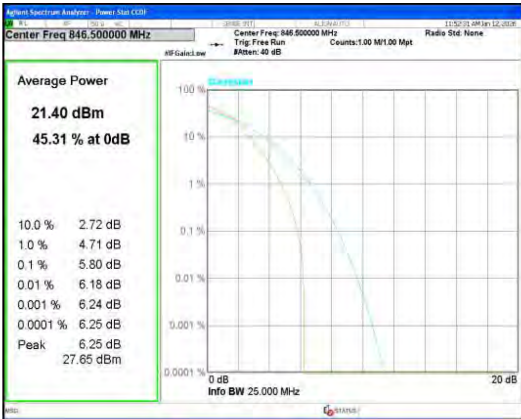
Band26(824-849) 16QAM BW=5MHz Channel=26915 RB Size=1 Position=#0
