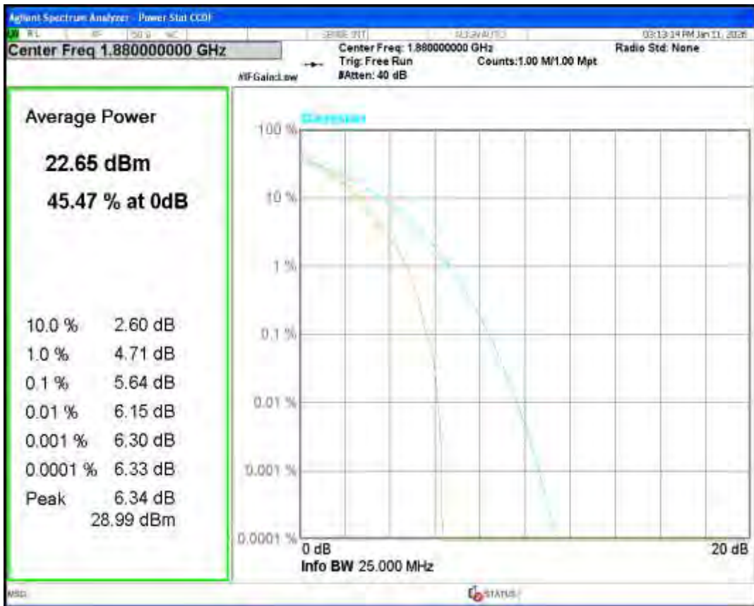
Band2 QPSK BW=10MHz Channel=19150 RB Size=1 Position=#0
