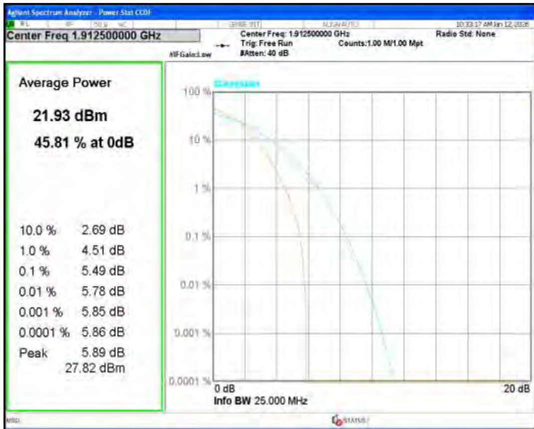
Band25 16QAM BW=5MHz Channel=26365 RB Size=1 Position=#0
