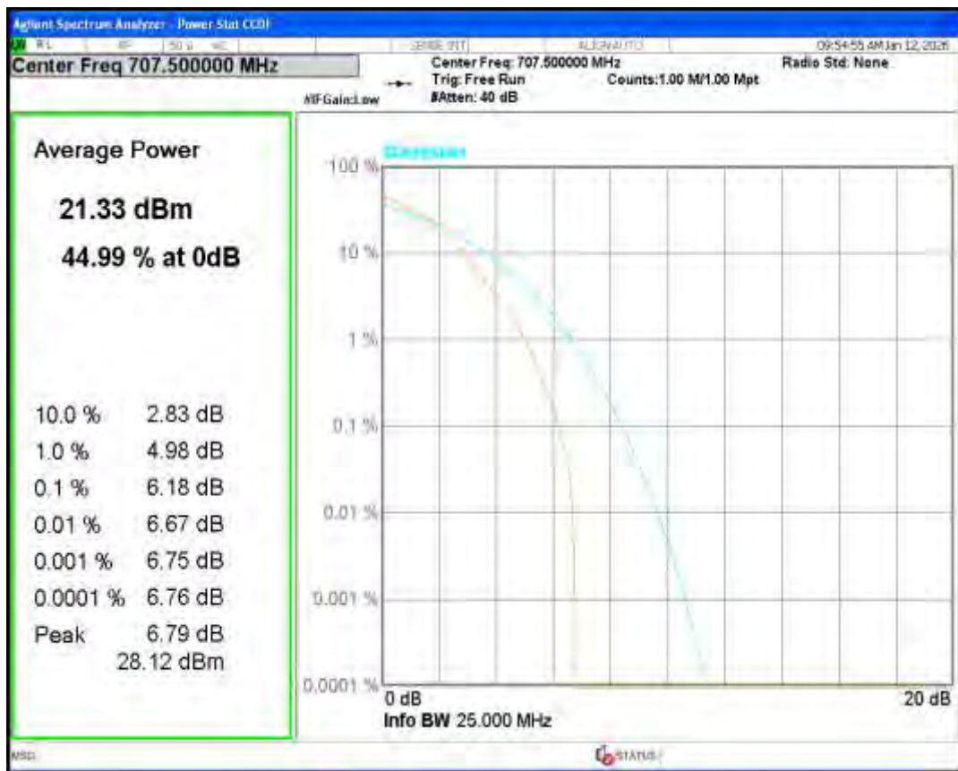
Band12 16QAM BW=1.4MHz Channel=23173 RB Size=1 Position=#0
