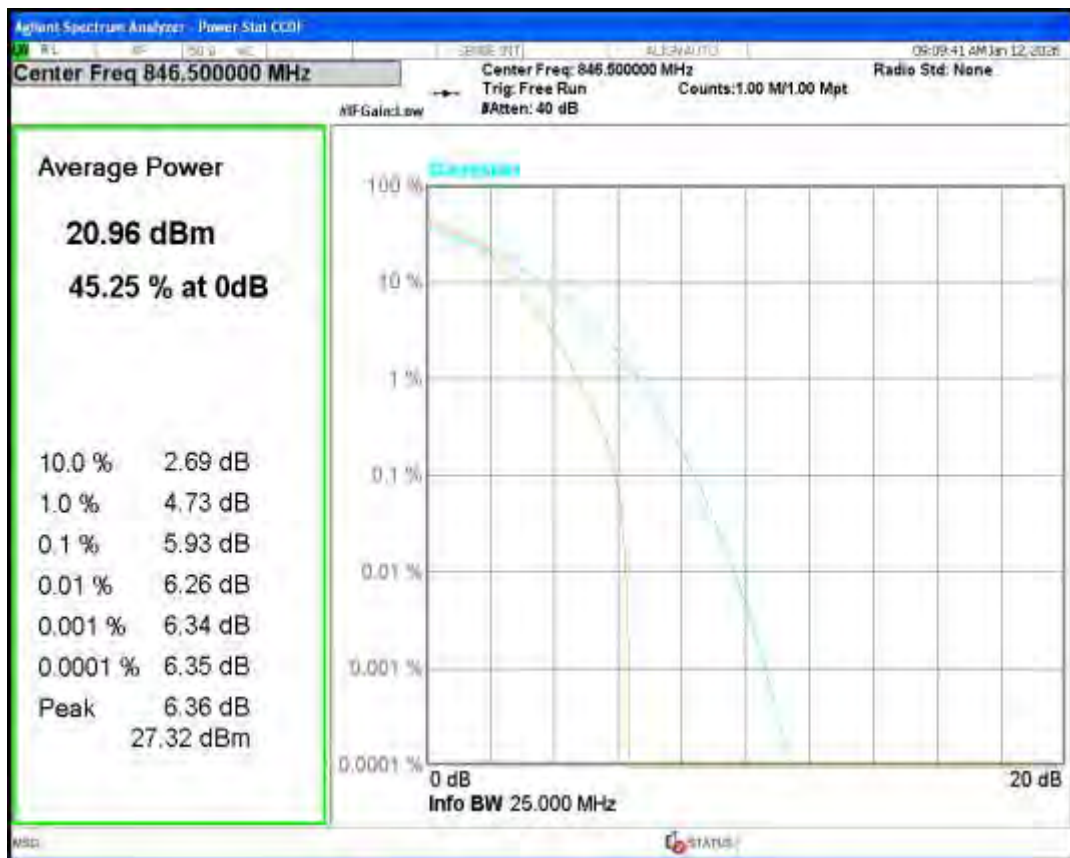
Band5 16QAM BW=3MHz Channel=20635 RB Size=1 Position=#0
