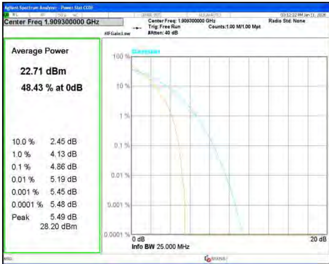
Band2 QPSK BW=3MHz Channel=18615 RB Size=1 Position=#0
