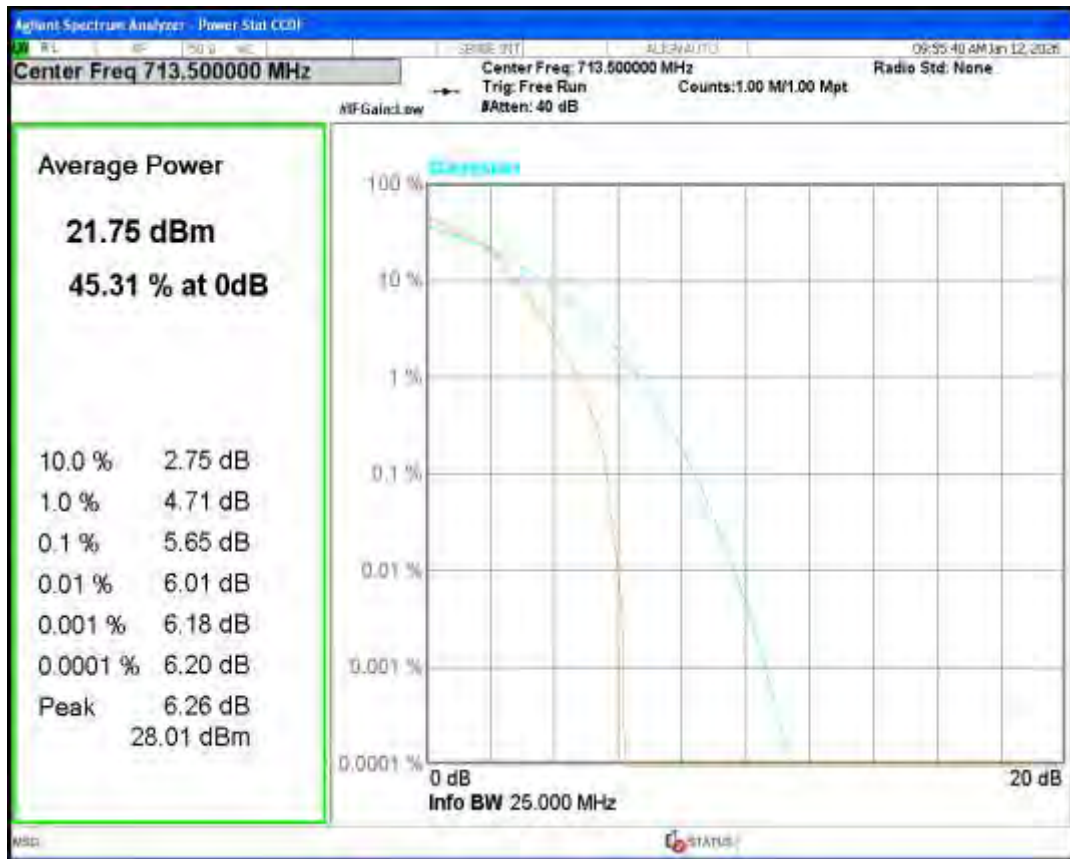
Band12 16QAM BW=5MHz Channel=23035 RB Size=1 Position=#0
