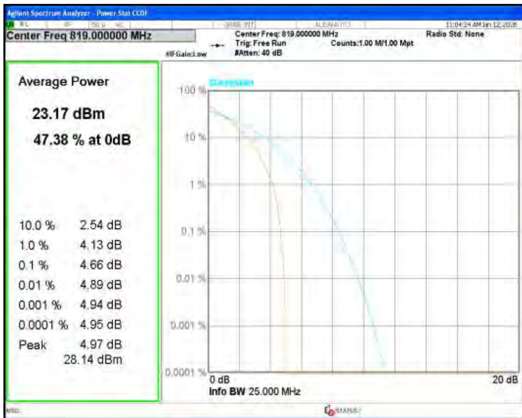
Band26(814-824) QPSK BW=5MHz Channel=26765 RB Size=1 Position=#0
