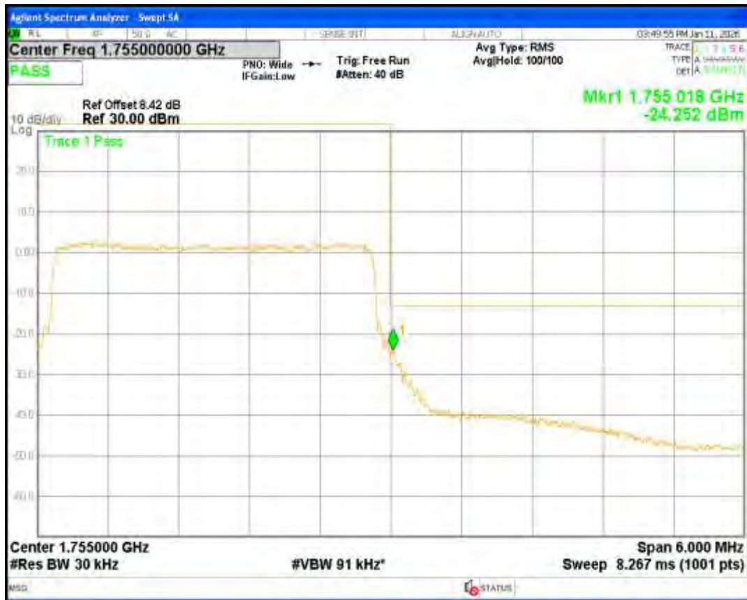
Band4 16QAM BW=5MHz Channel=19975 RB Size=25 Position=#0
