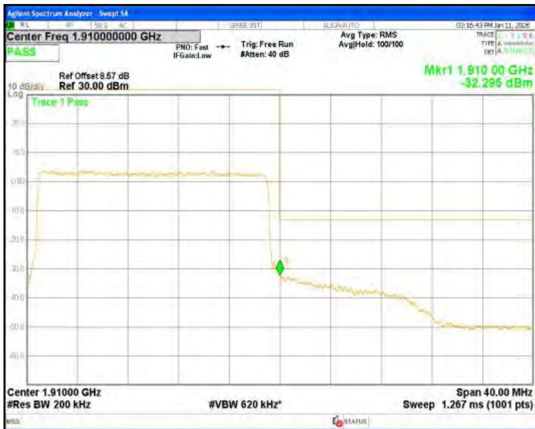
Band25 16QAM BW=1.4MHz Channel=26047 RB Size=6 Position=#0
