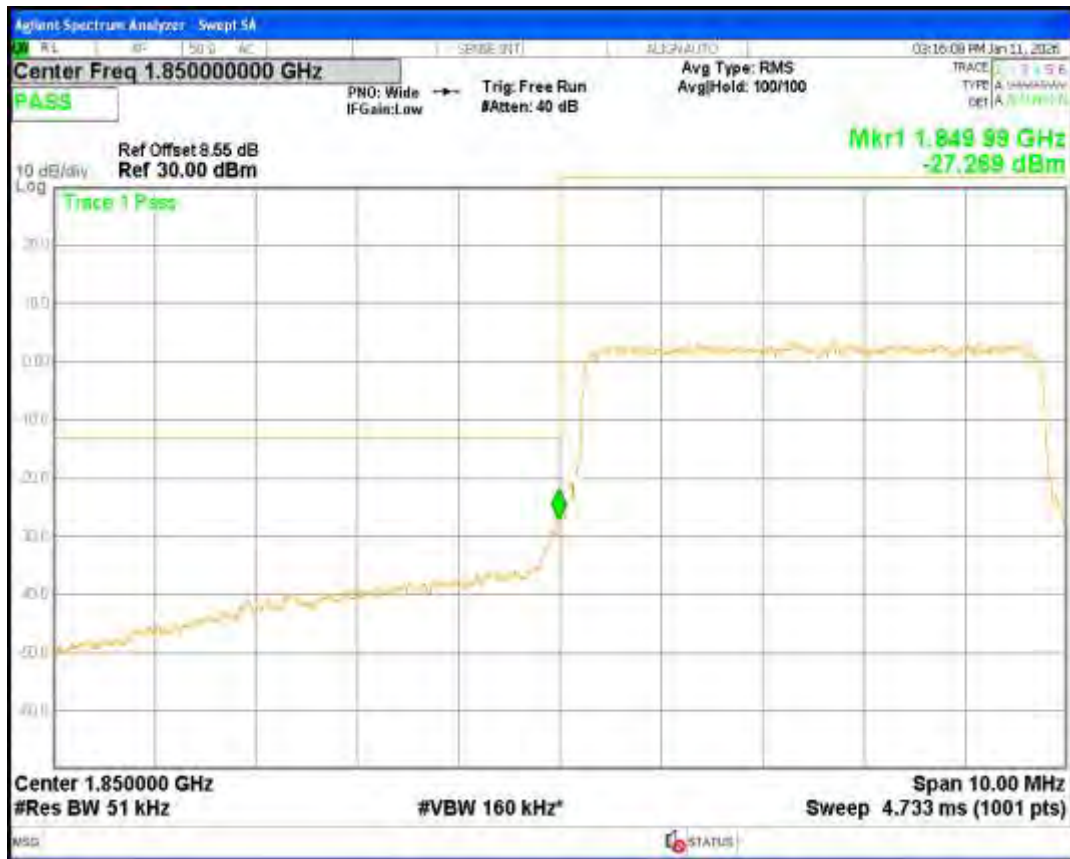
Band2 16QAM BW=5MHz Channel=19175 RB Size=25 Position=#0
