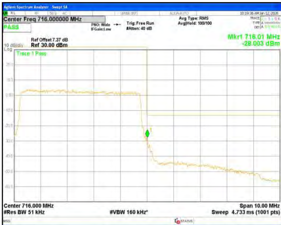
Band17 QPSK BW=10MHz Channel=23780 RB Size=50 Position=#0
