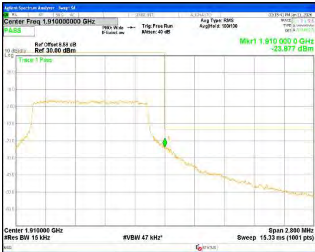
Band2 16QAM BW=3MHz Channel=18615 RB Size=15 Position=#0
