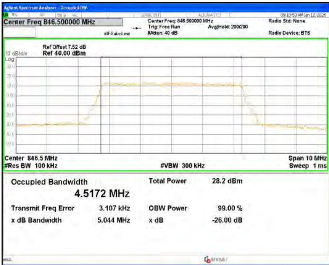
Band5 16QAM BW=5MHz Channel=20525 RB Size=25 Position=#0
