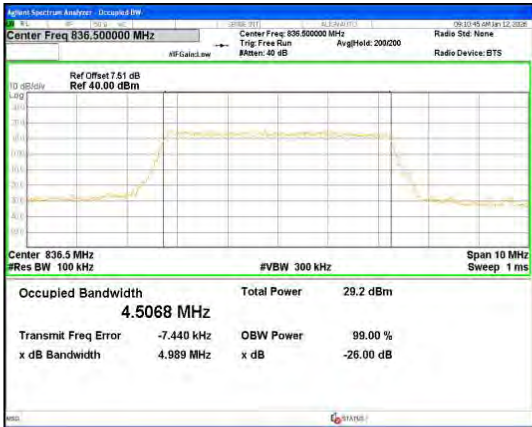
Band5 QPSK BW=5MHz Channel=20625 RB Size=25 Position=#0
