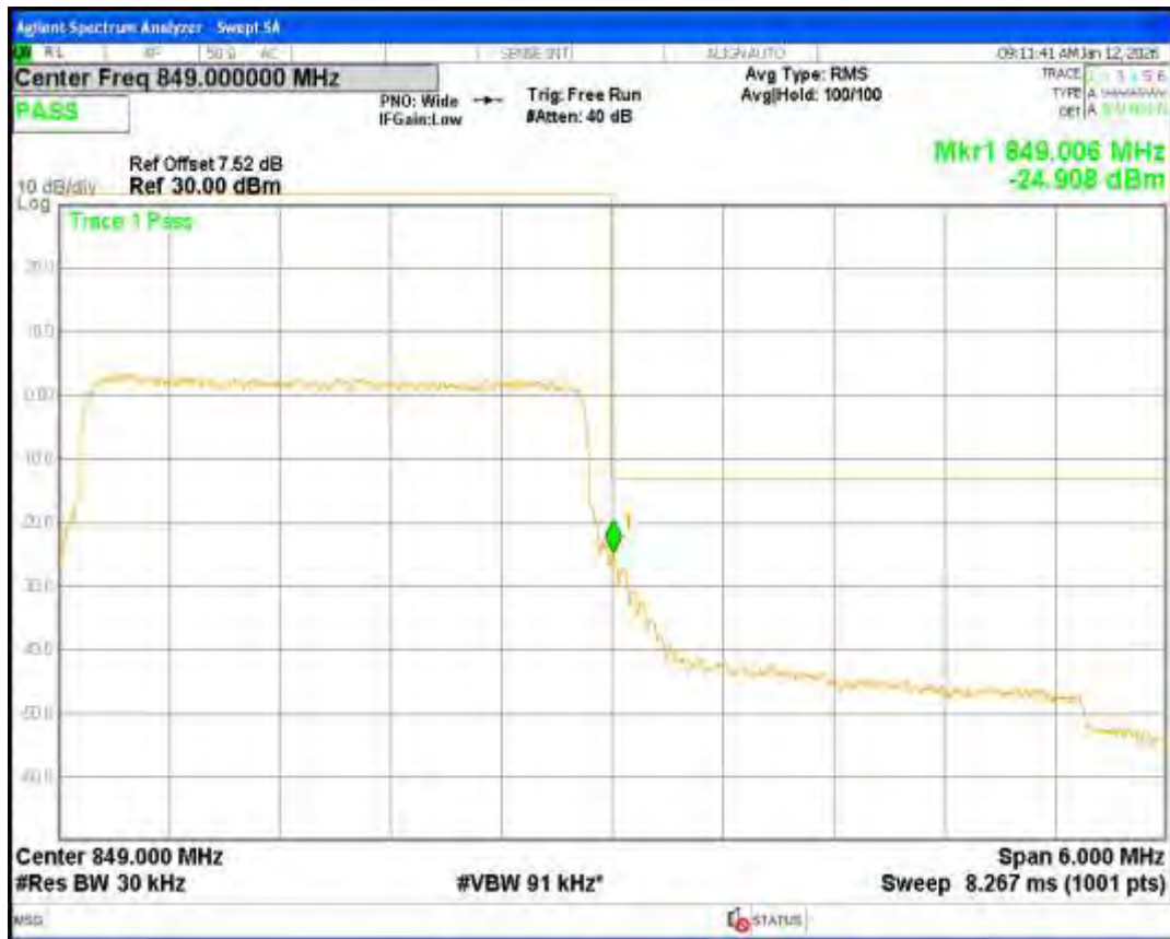
Band5 QPSK BW=5MHz Channel=20425 RB Size=25 Position=#0
