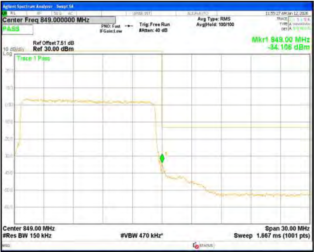
Band38 16QAM BW=5MHz Channel=37775 RB Size=25 Position=#0
