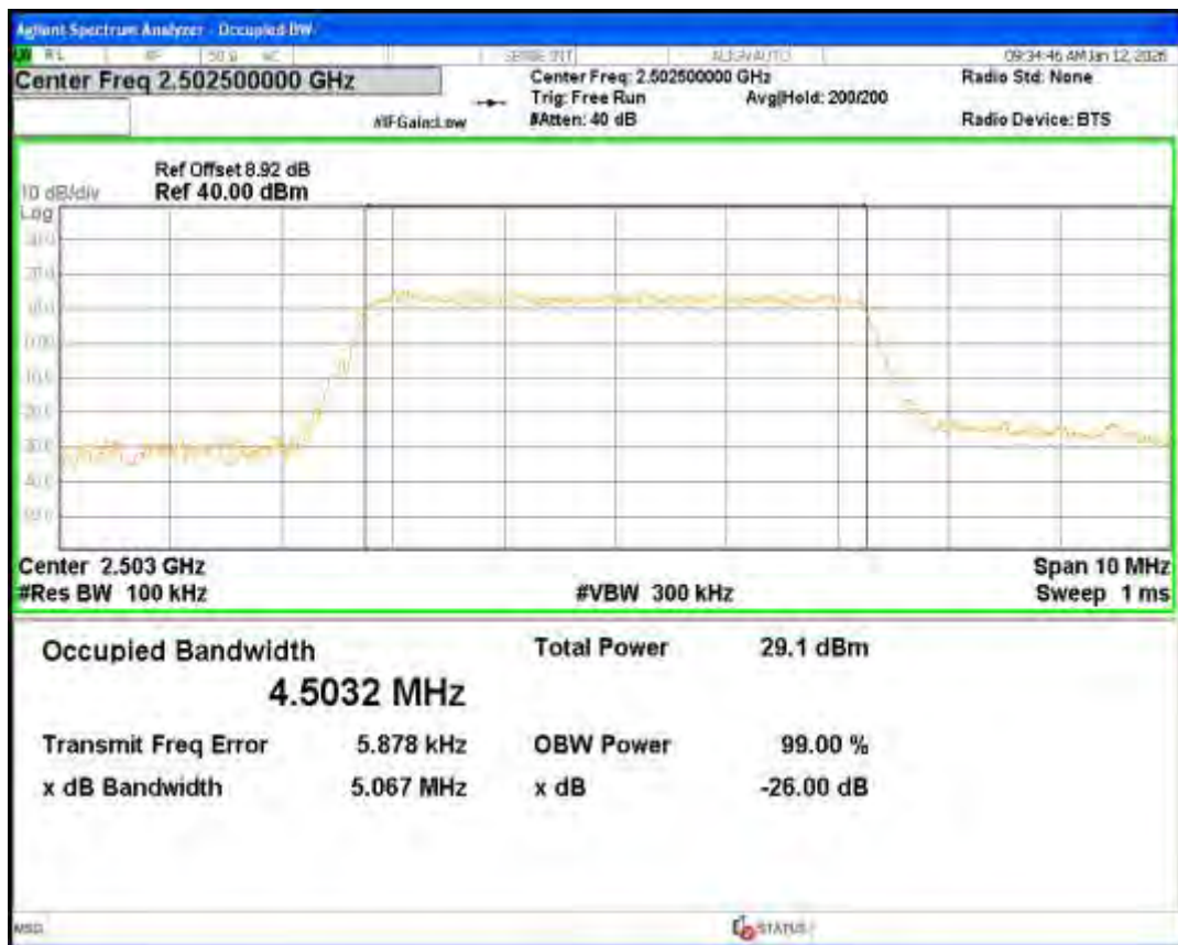
Band7 16QAM BW=5MHz Channel=21100 RB Size=25 Position=#0
