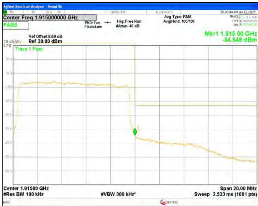
Band25 QPSK BW=15MHz Channel=26115 RB Size=75 Position=#0
