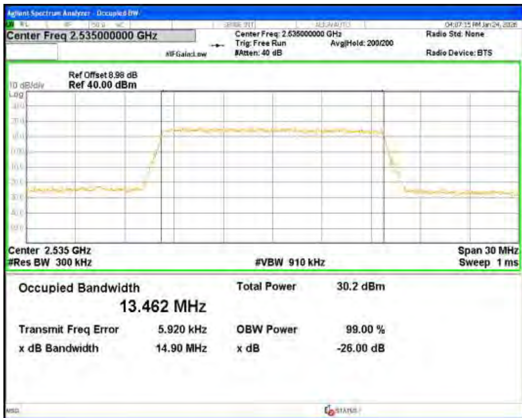
Band7 QPSK BW=15MHz Channel=21375 RB Size=75 Position=#0
