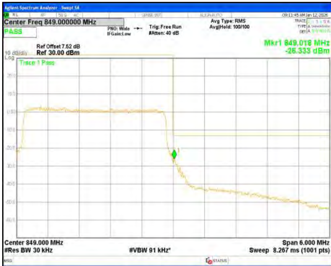
Band5 16QAM BW=5MHz Channel=20425 RB Size=25 Position=#0
