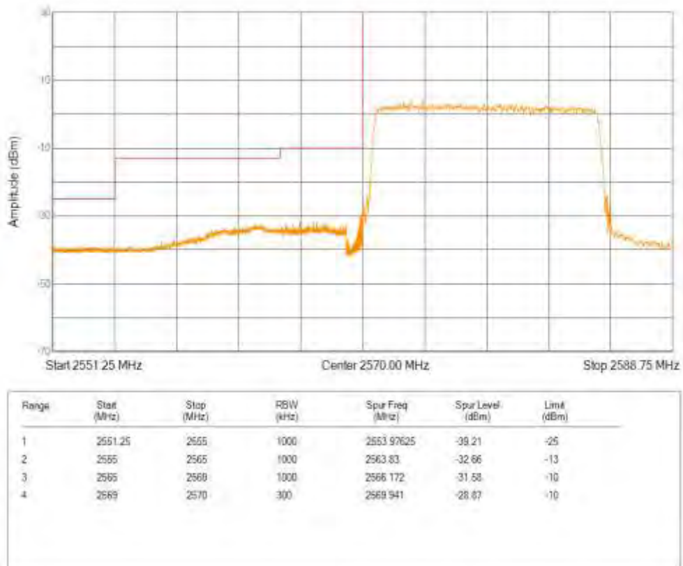
Band38 QPSK BW=15MHz Channel=38175 RB Size=75 Position=#0
