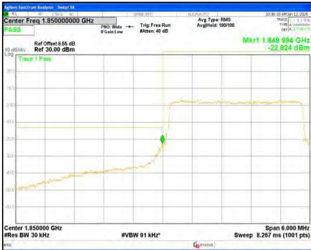
Band25 16QAM BW=3MHz Channel=26675 RB Size=15 Position=#0
