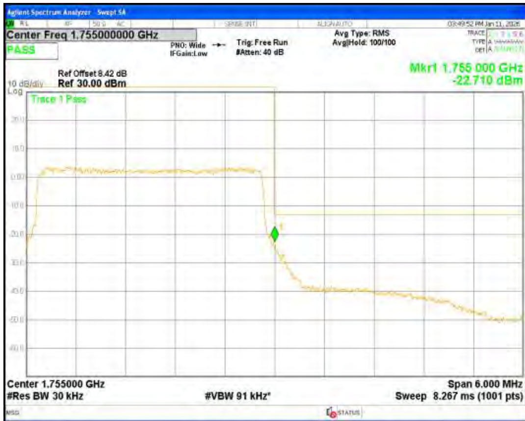
Band4 QPSK BW=5MHz Channel=19975 RB Size=25 Position=#0
