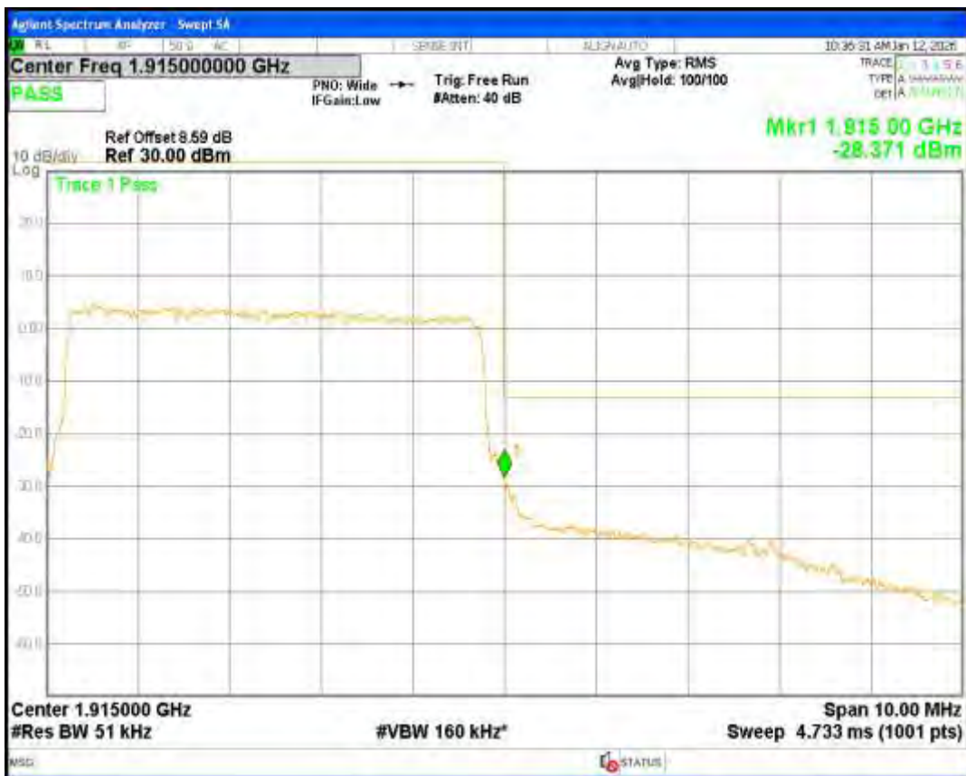
Band25 QPSK BW=10MHz Channel=26090 RB Size=50 Position=#0
