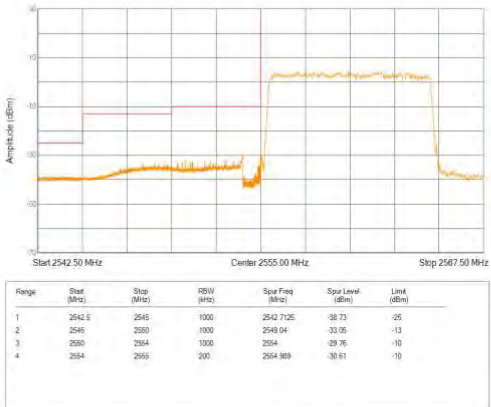
Band41(2555-2655) QPSK BW=10MHz Channel=41190 RB Size=50 Position=#0
