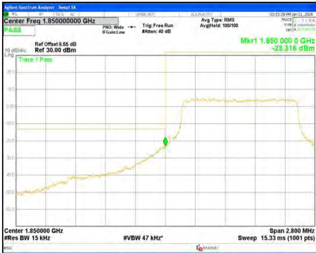
Band2 QPSK BW=1.4MHz Channel=19193 RB Size=6 Position=#0
