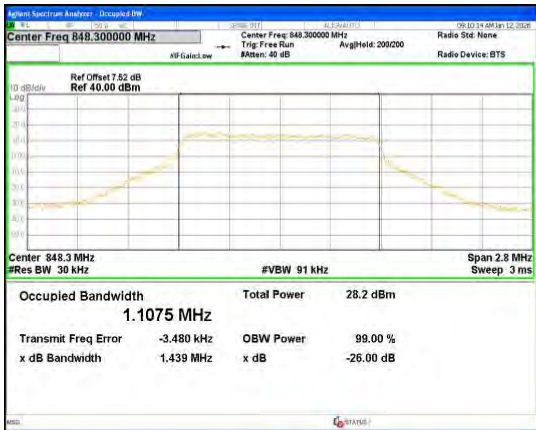
Band5 16QAM BW=3MHz Channel=20415 RB Size=15 Position=#0
