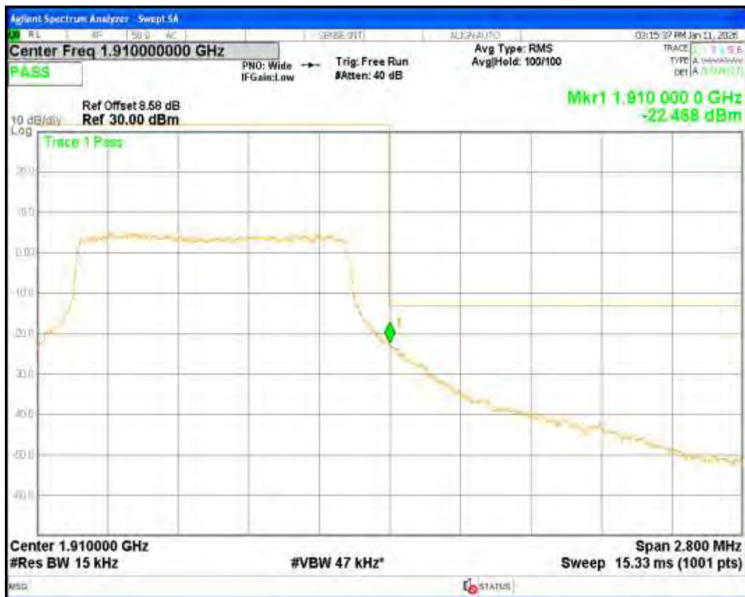
Band2 QPSK BW=3MHz Channel=18615 RB Size=15 Position=#0
