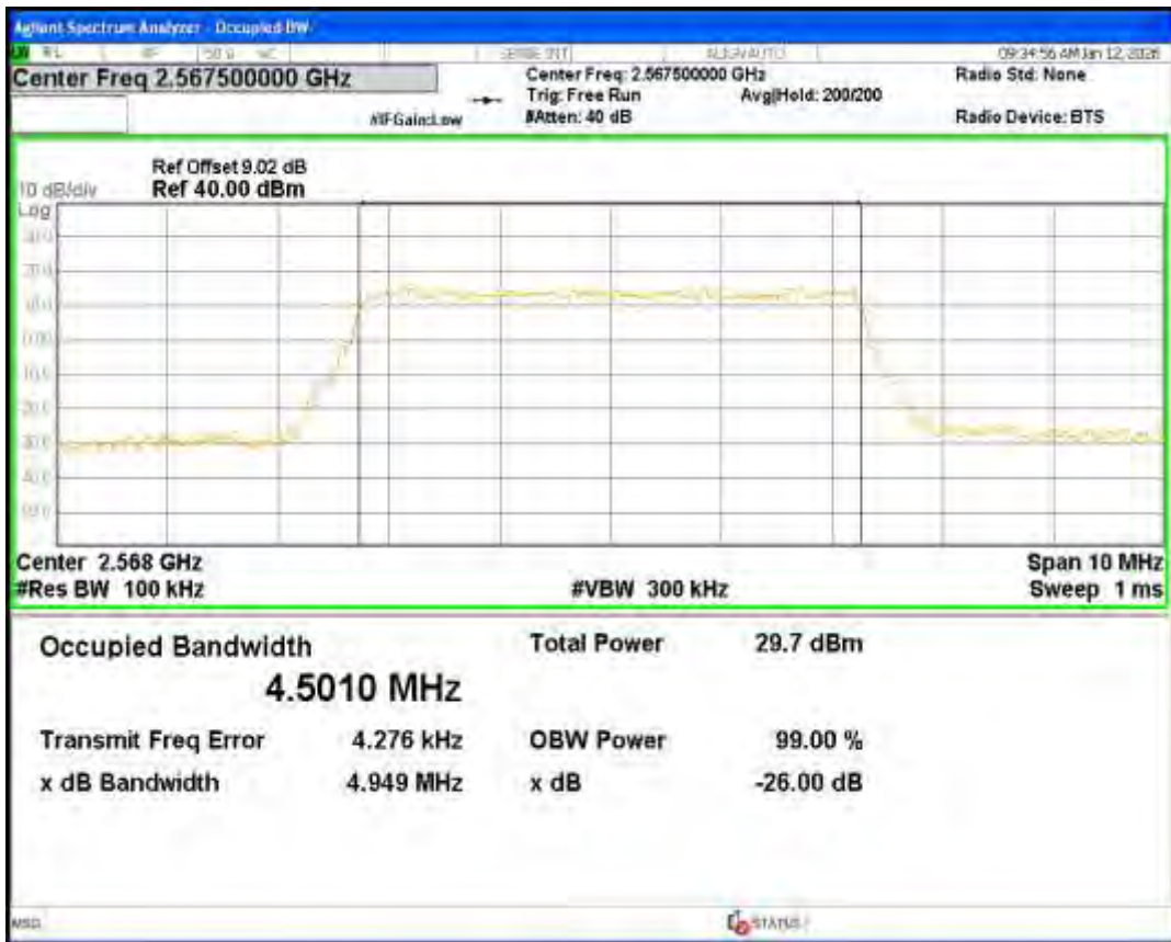
Band7 QPSK BW=10MHz Channel=20800 RB Size=50 Position=#0
