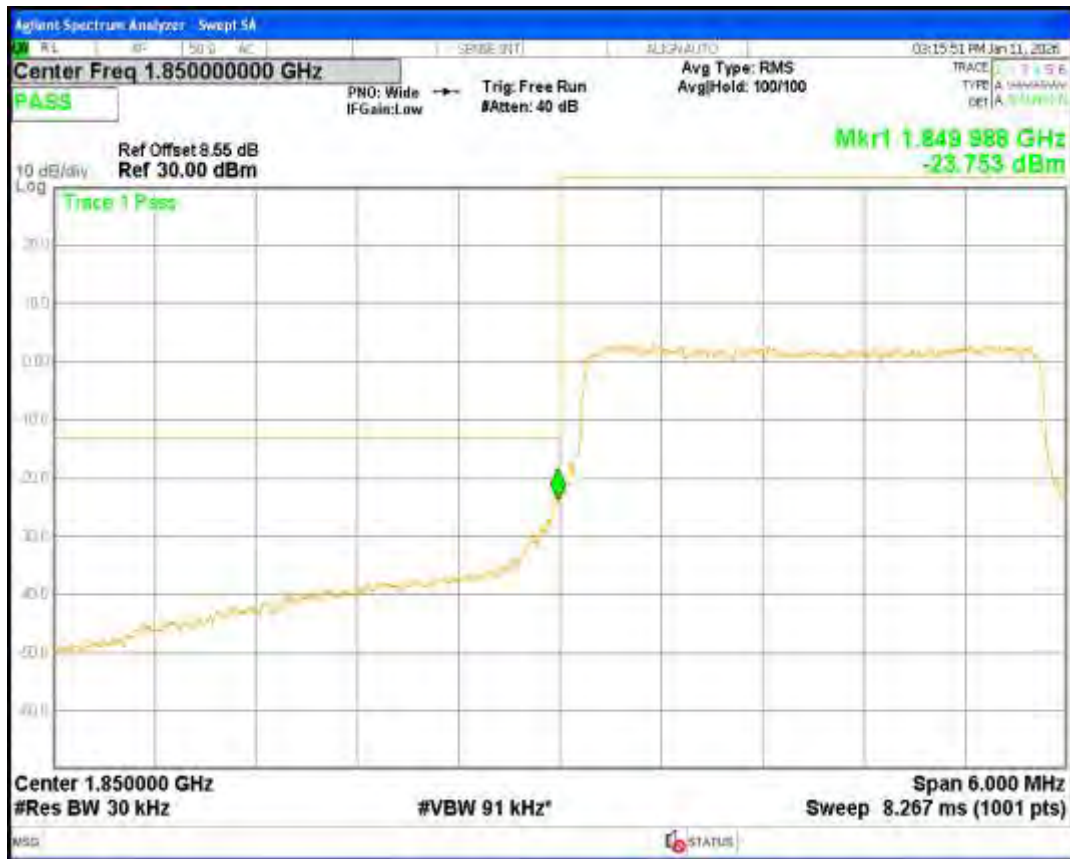
Band2 16QAM BW=3MHz Channel=19185 RB Size=15 Position=#0
