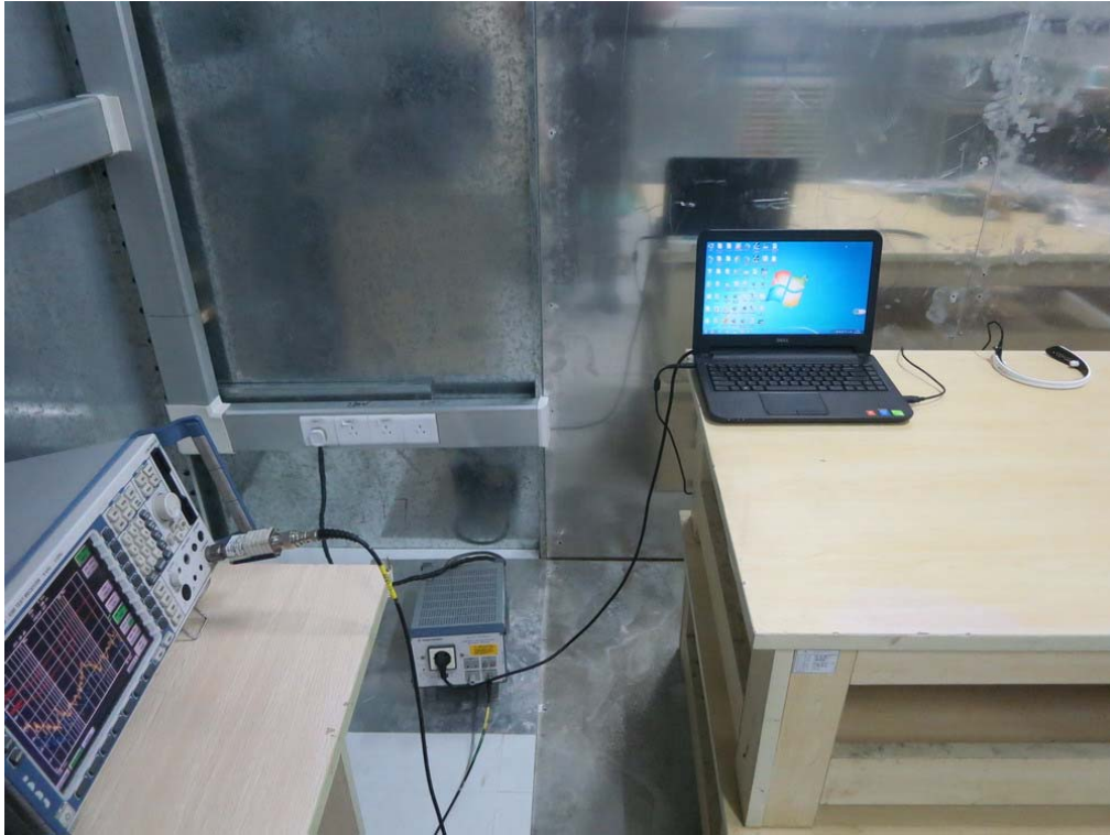
FCC RADIATED EMISSION TEST SETUP
