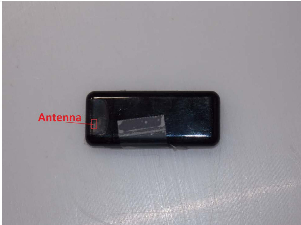
Antenna Location – The antenna is 5 mm from the back (tested) surface of the device.
