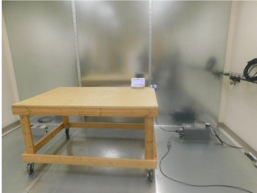
AC Power Line Conducted Emissions
