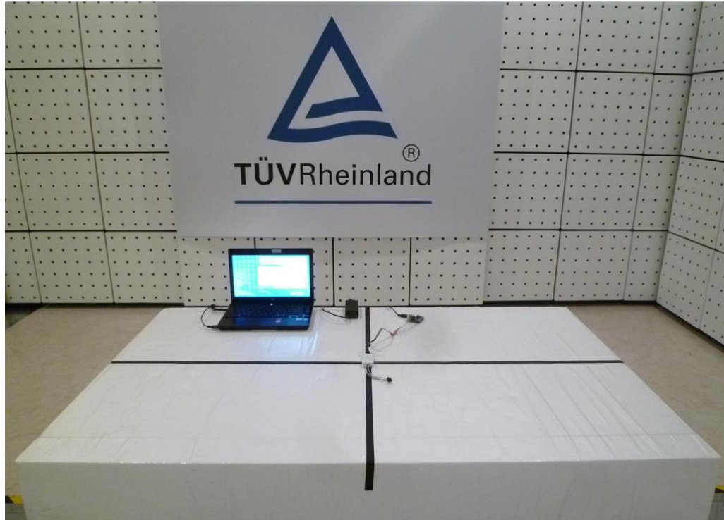
Photograph 1: Set-up for Spurious Emissions (Front View)
