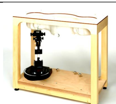
Fig 5.8 Photo of SAM Phantom
