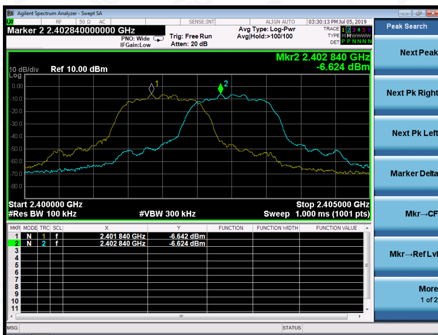
TEST PLOT FOR FREQUENCY SEPARATION
