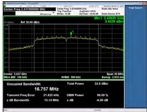
6 dB Bandwidth, Channel 6, 802.11g, 6Mbps
