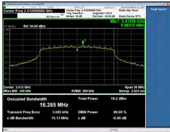
6 dB Bandwidth, Channel 1, 802.11g, 6Mbps
