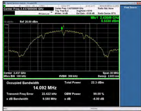
6 dB Bandwidth, Channel 6, 802.11b, 1 Mbps
