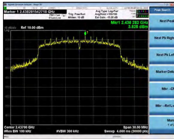
Reference Plot, 802.11n, MCS0 Channel 6, 3.8 dBm
