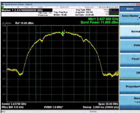
Output Power, Channel 6, 802.11b, 11Mbps
