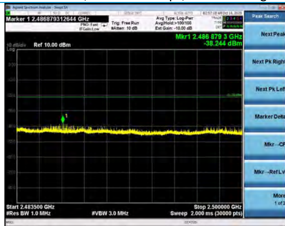
2.4835-2.5 GHz, Terminated Method, 1 MHz RBW Channel 11, 802.11b 1Mbps, Peak Reading
