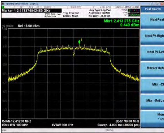
Reference Plot, 802.11g, 6Mbps Channel 1, 0.5 dBm
