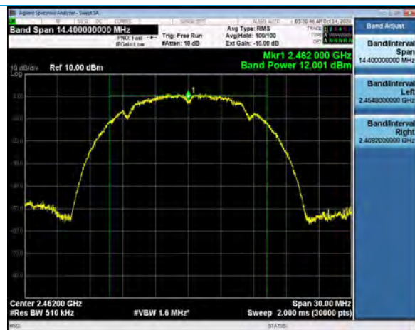
Output Power, Channel 11, 802.11b, 11Mbps
