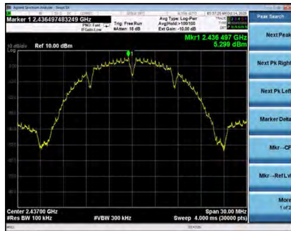
Reference Plot, 802.11b, 1Mbps Channel 6, 5.3 dBm
