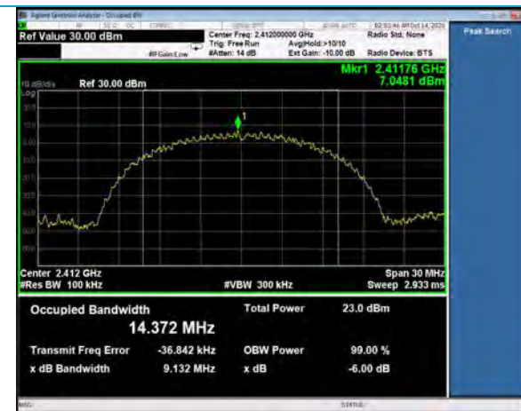
6 dB Bandwidth, Channel 1, 802.11b, 11Mbps
