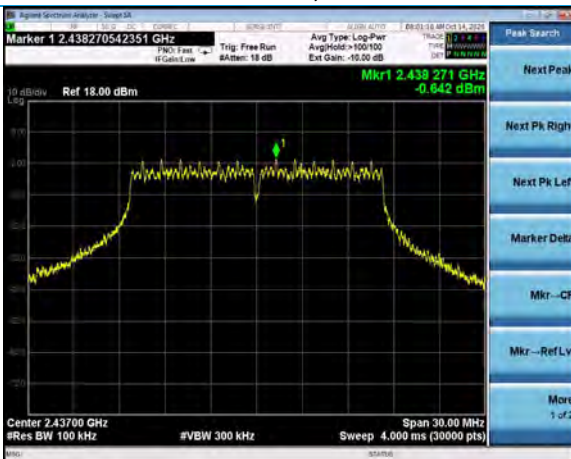
Reference Plot, 802.11g, 54Mbps Channel 6, -0.6 dBm
