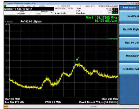
30-200 MHz, Horizontal Antenna, Vertical EUT Channel 11
