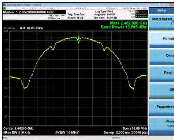
Output Power, Channel 11, 802.11b, 1Mbps
