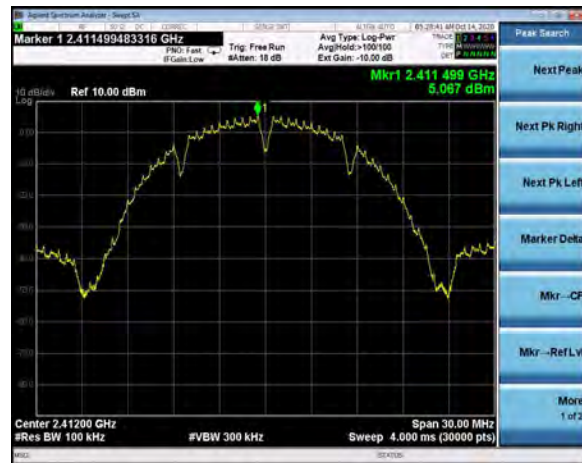
Reference Plot, 802.11b, 1Mbps Channel 1, 5.0 dBm
