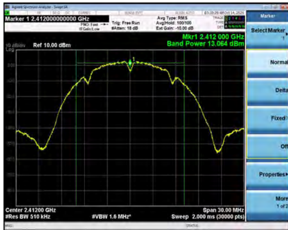
Output Power, Channel 1, 802.11b, 1Mbps
