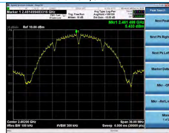
Reference Plot, 802.11b, 1Mbps Channel 11, 5.4 dBm
