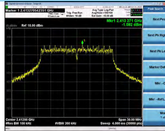
Reference Plot, 802.11g, 54Mbps Channel 1, -1.1 dBm
