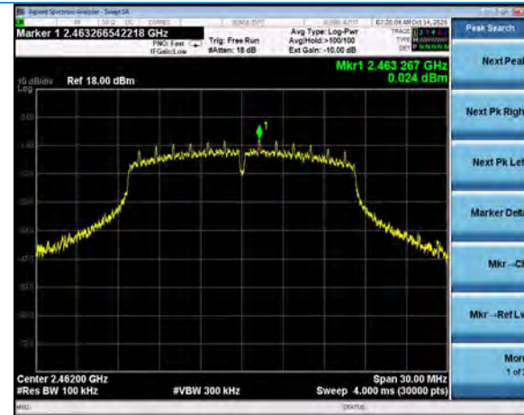
Reference Plot, 802.11g, 6Mbps Channel 11, 0.0 dBm
