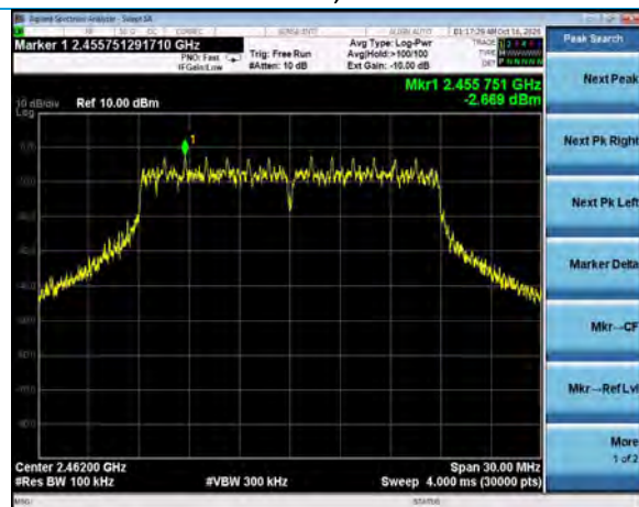
Reference Plot, 802.11n, MCS7 Channel 11, -2.7 dBm
