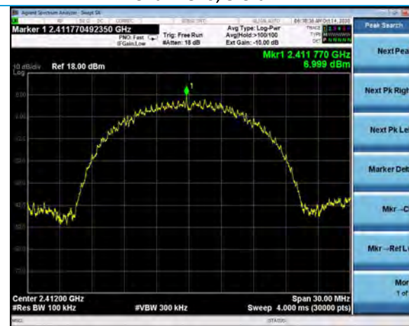
Reference Plot, 802.11b, 11Mbps Channel 1, 7.0 dBm
