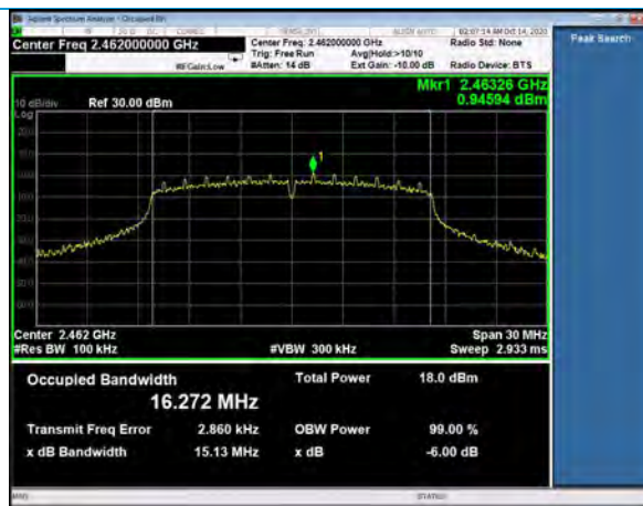
6 dB Bandwidth, Channel 11, 802.11g, 6Mbps
