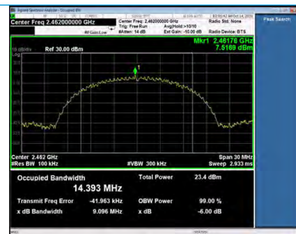
6 dB Bandwidth, Channel 11, 802.11b, 11Mbps
