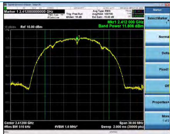
Output Power, Channel 1, 802.11b, 11Mbps
