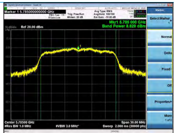
Output Power, Channel 157, 802.11a, 6Mbps
