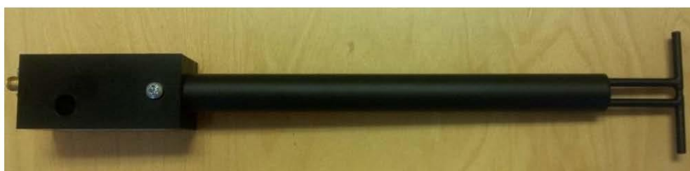
Figure 1 – MVG COMOSAR Validation Dipole
