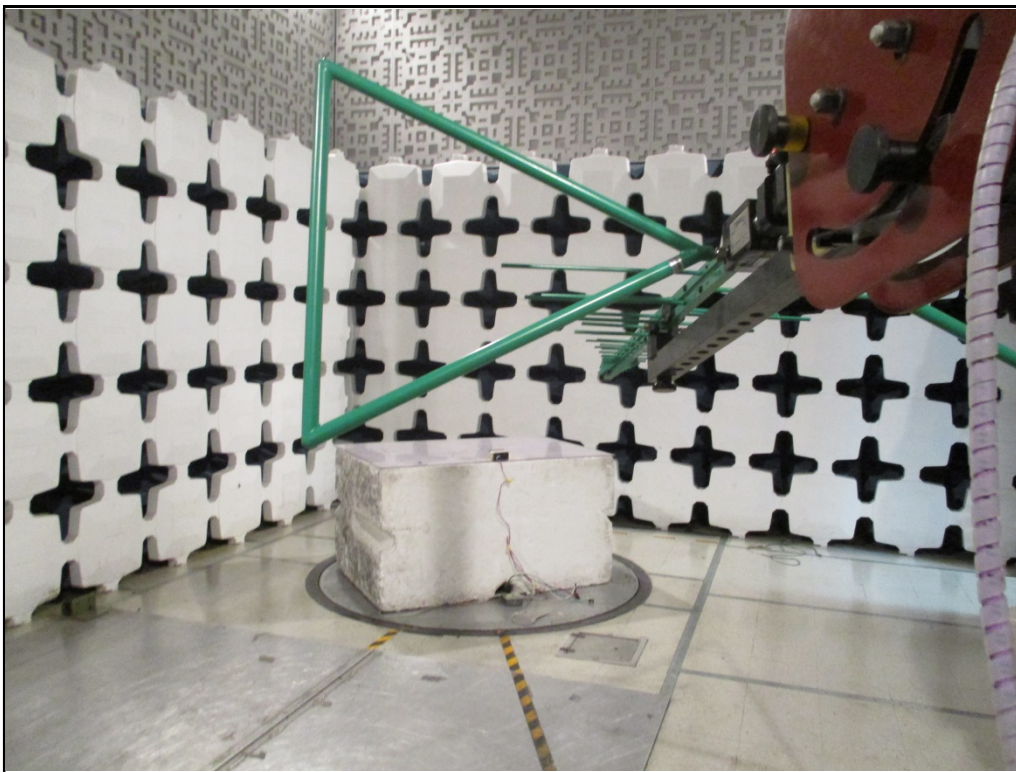
Test Setup for Effective Isotropic Radiated Power – Horizontal Polarization
