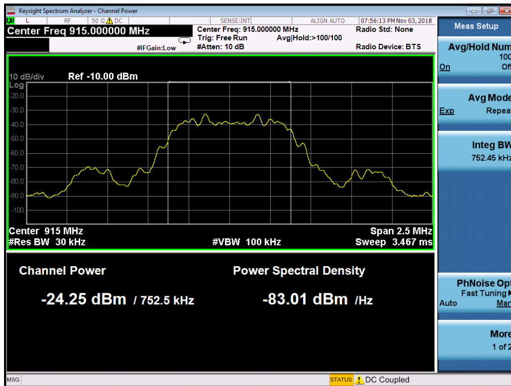
Channel Power – Mid Channel
