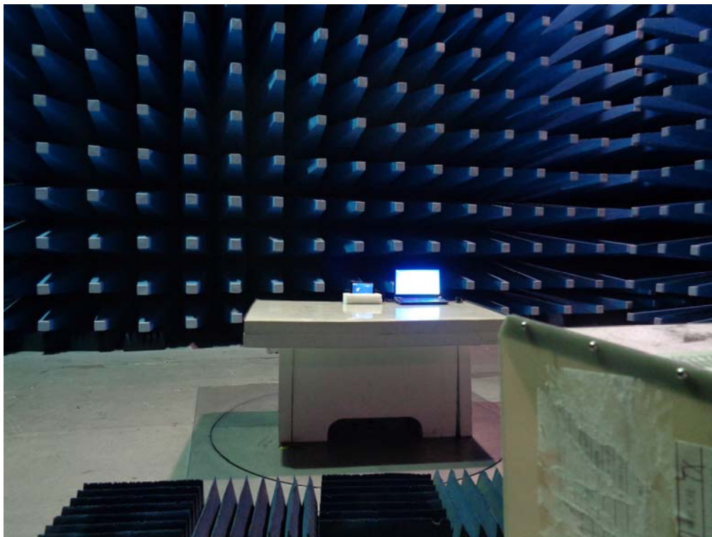
Radiated Emissions Setup Above 1GHz Front View
