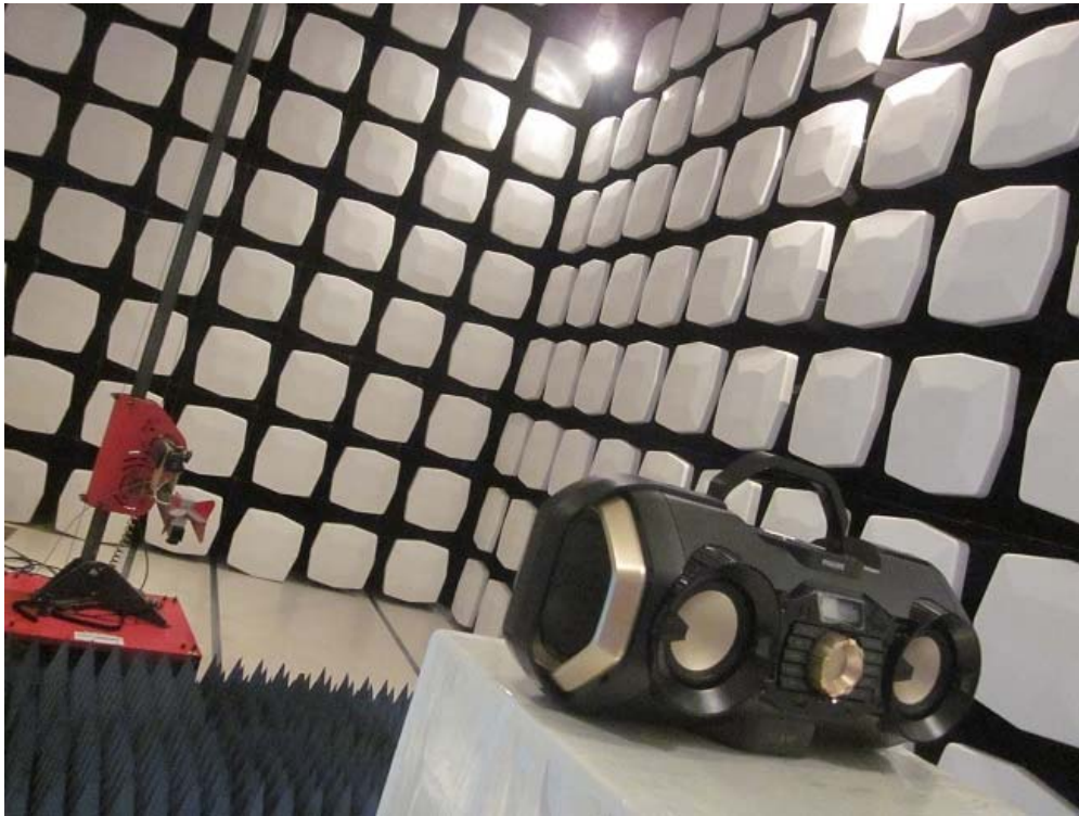
Measurement of Radiated Emission Test Set Up
