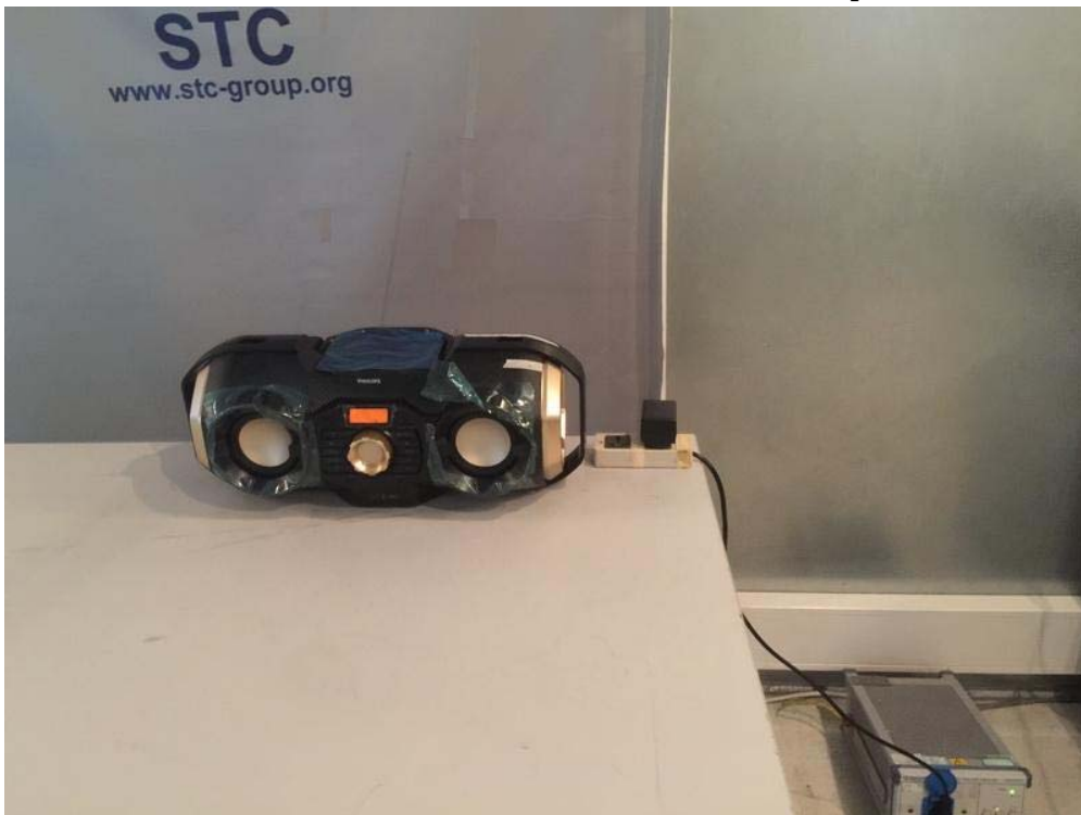
Measurement of Conducted Emission Test Set Up
