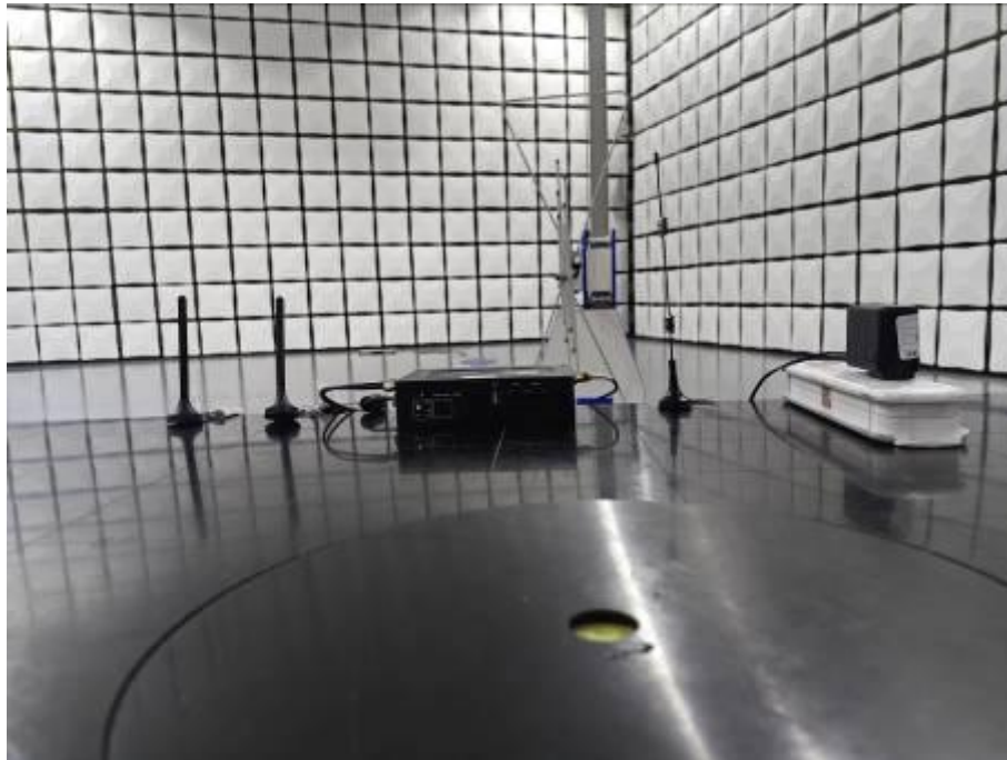
Radiated Emissions Test Setup (30-1000MHz)
