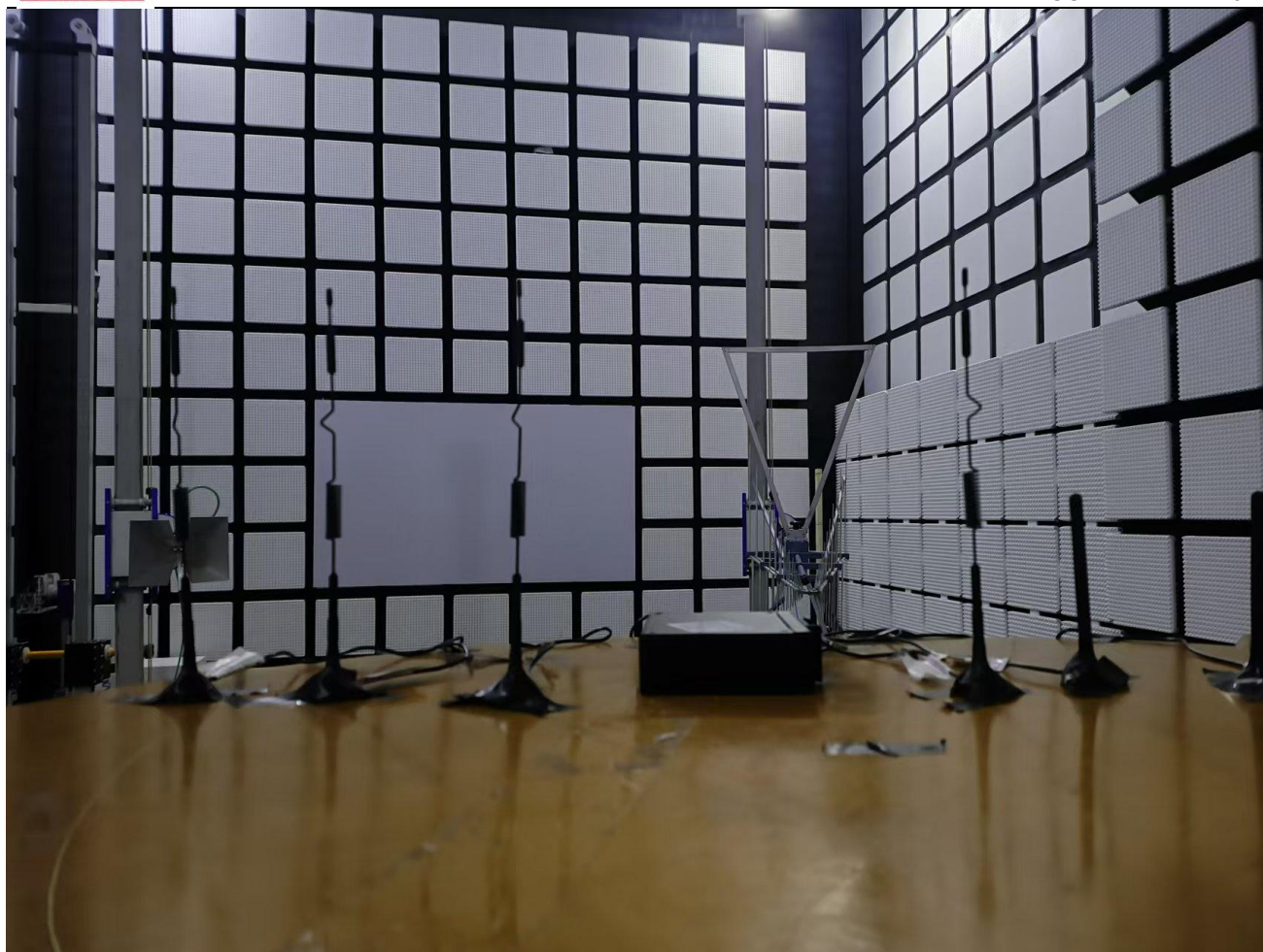
RF Radiated Test setup (RSE)
