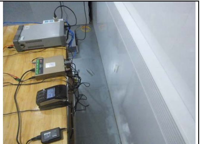
Conducted Emissions Test Setup – Rear View
