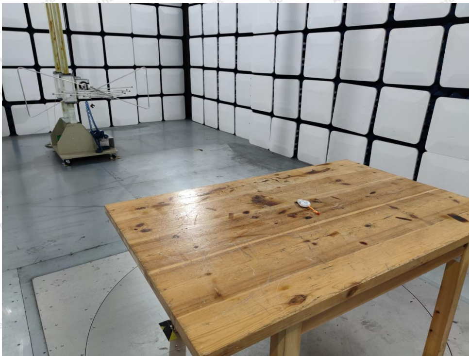
Photo of Radiation Emission Test
