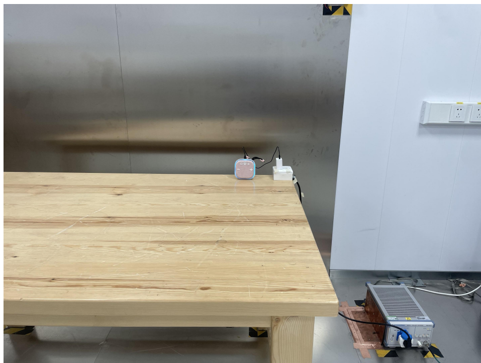
Radiated Emission Test View|(Below 1G)
