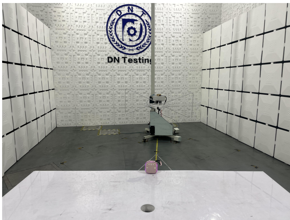
Radiated Emission Test View|(Below 1G)
