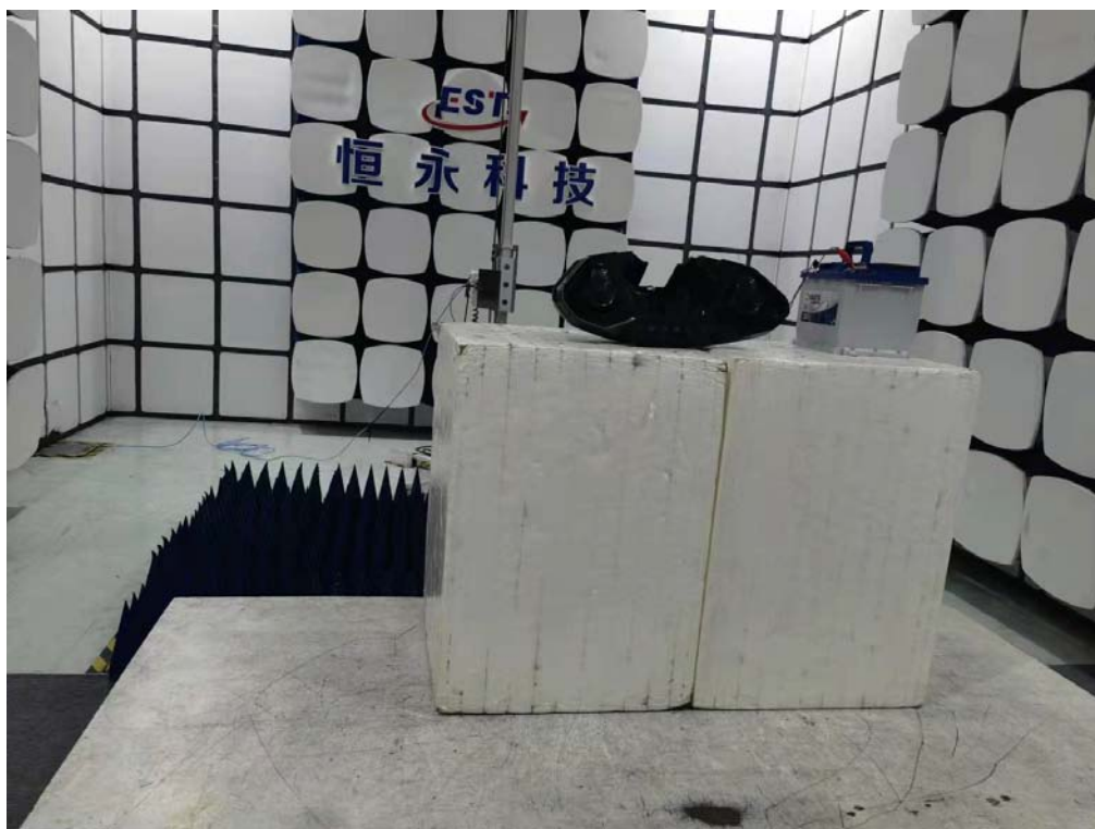
Radiated emission test: Above 1GHz
