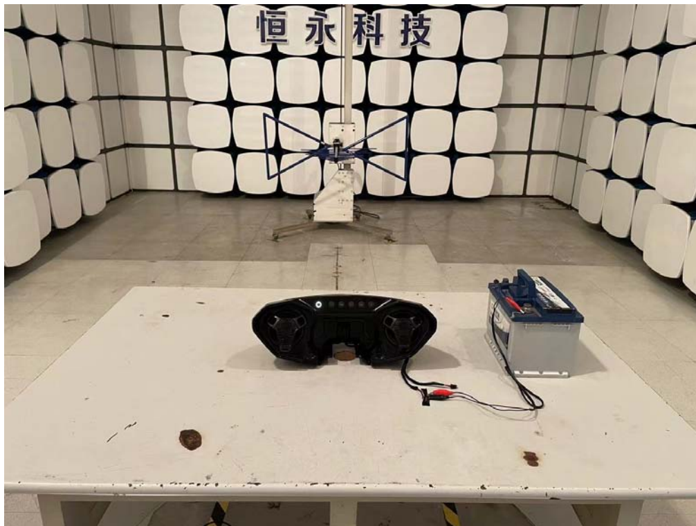
Radiated emission test: Below 1GHz
