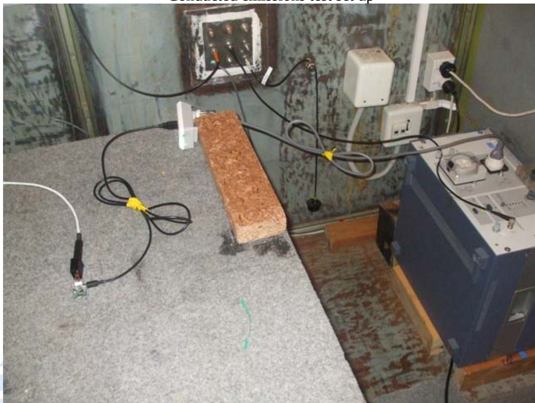
Conducted emissions test set up
