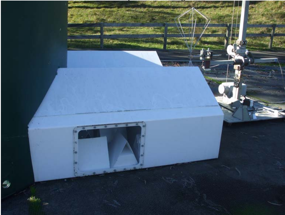
Cone enclosure up close showing the cones
