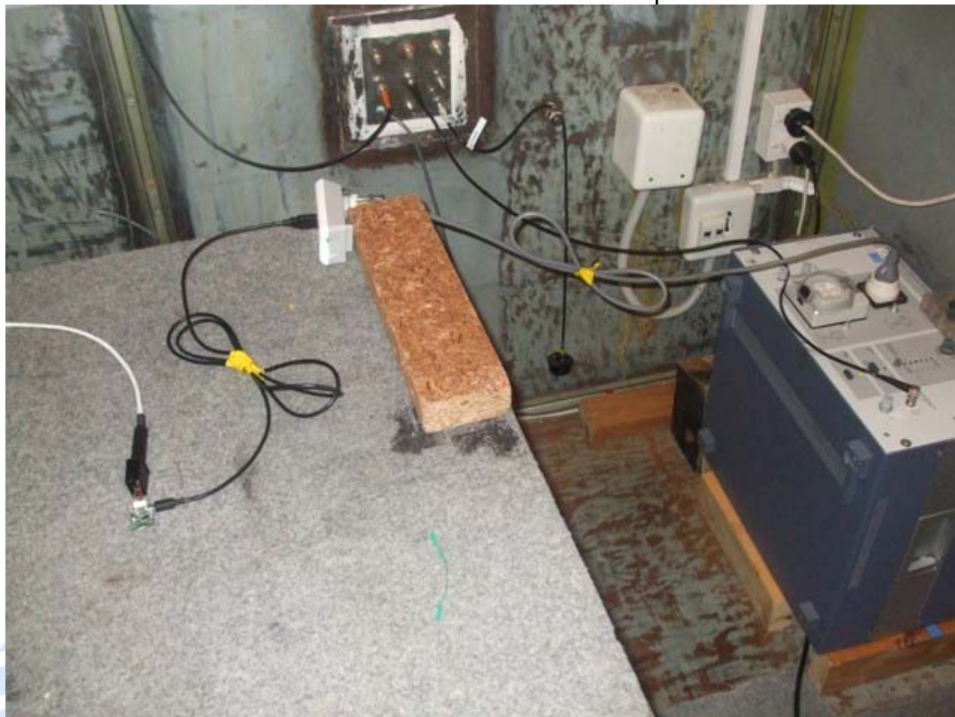
Conducted emissions test set up
