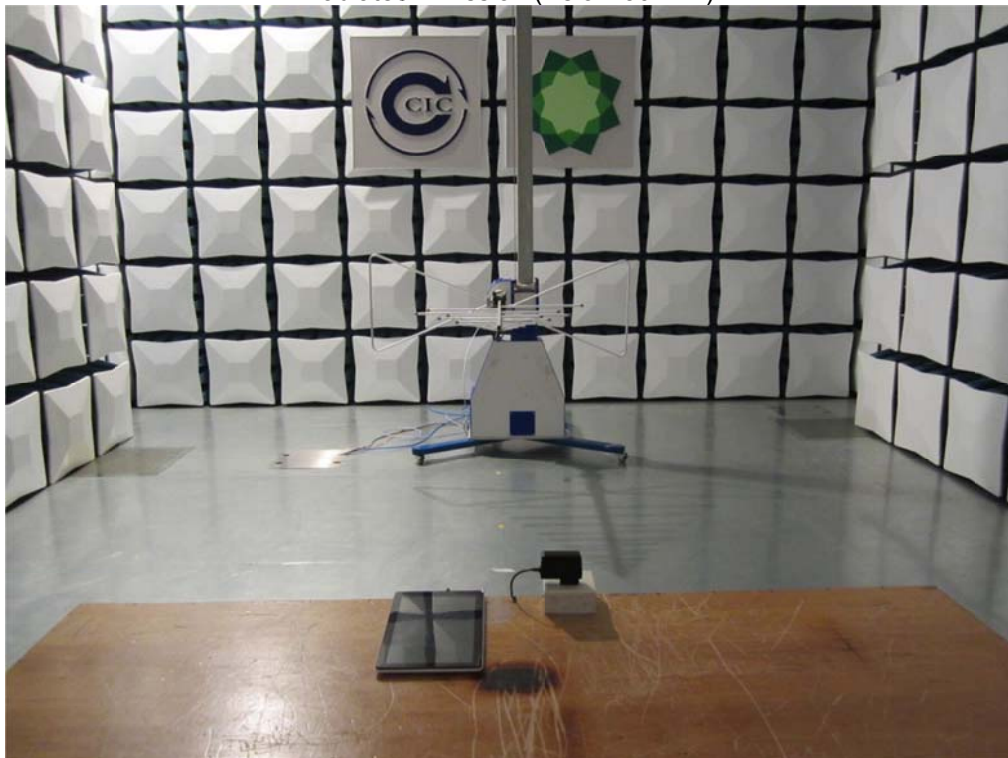
Radiated Emission (Below 30MHz)
