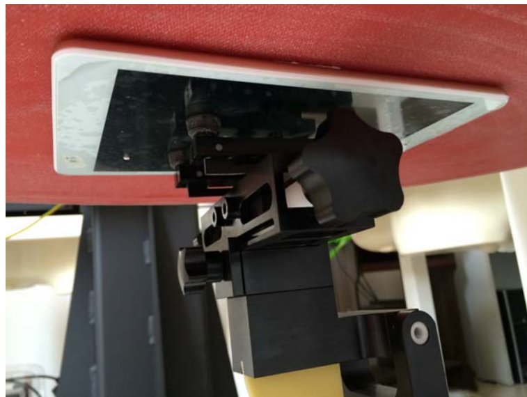
0mm Body Rear Side Setup Photo
