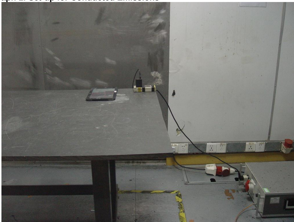
Photograph 2: Set-up for Spurious Emissions for below 30MHz
