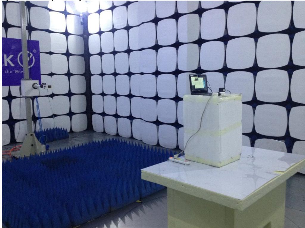
Photograph 5: Set-up for Spurious Emissions for 26.5 - 40GHz
