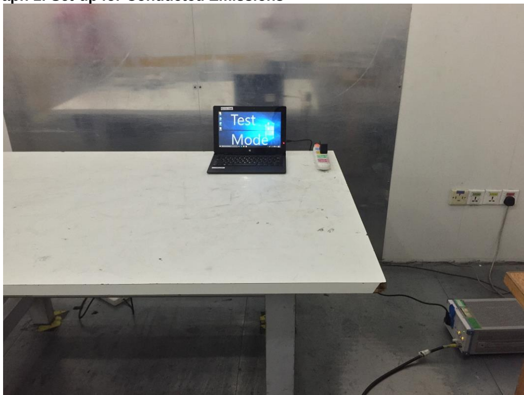
Photograph 2: Set-up for Spurious Emissions for below 30MHz
