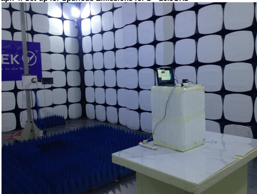
Photograph 4: Set-up for Spurious Emissions for 1 - 26.5GHz
