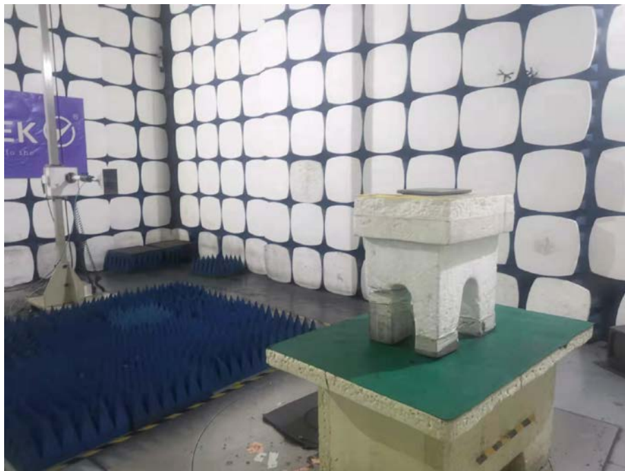
Spurious Emission Test Setup (Above 1GHz)
