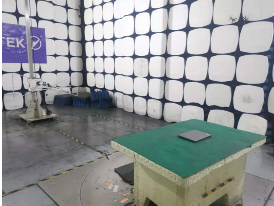
Spurious Emission Test Setup (Above 1GHz)
