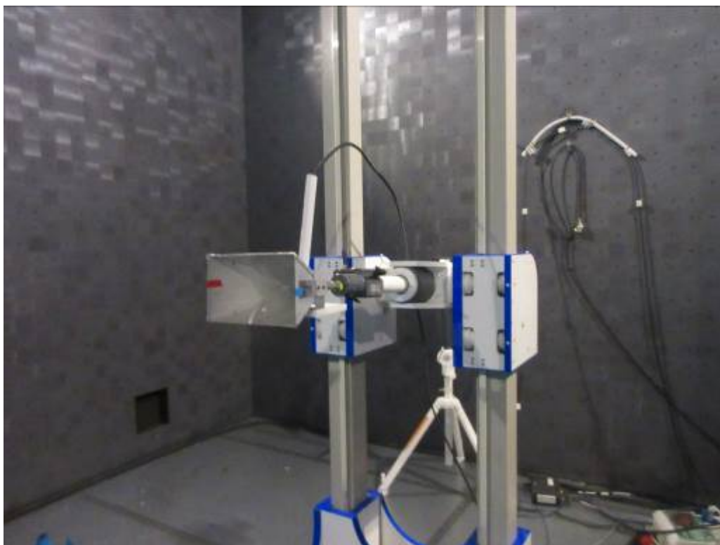
TEST SETUP PHOTO(S) RADIATED EMISSIONS ( F > 30\text{MHz} )
