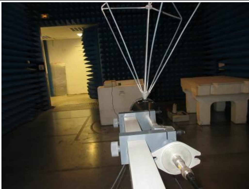
TEST SETUP PHOTO(S) RADIATED EMISSIONS (30MHz>F>300MHz)
