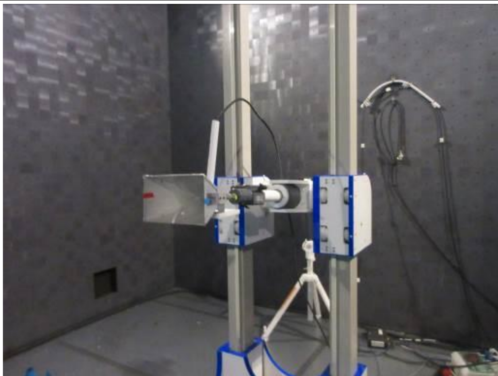
TEST SETUP PHOTO(S) RADIATED EMISSIONS ( F > 30\text{MHz} )
