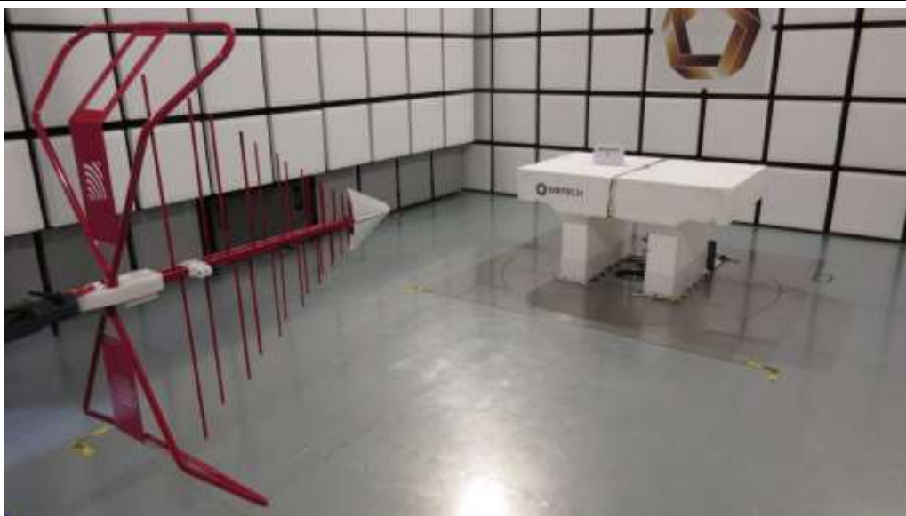
TEST SETUP PHOTO(S) – 30 MHz TO 1 GHz
