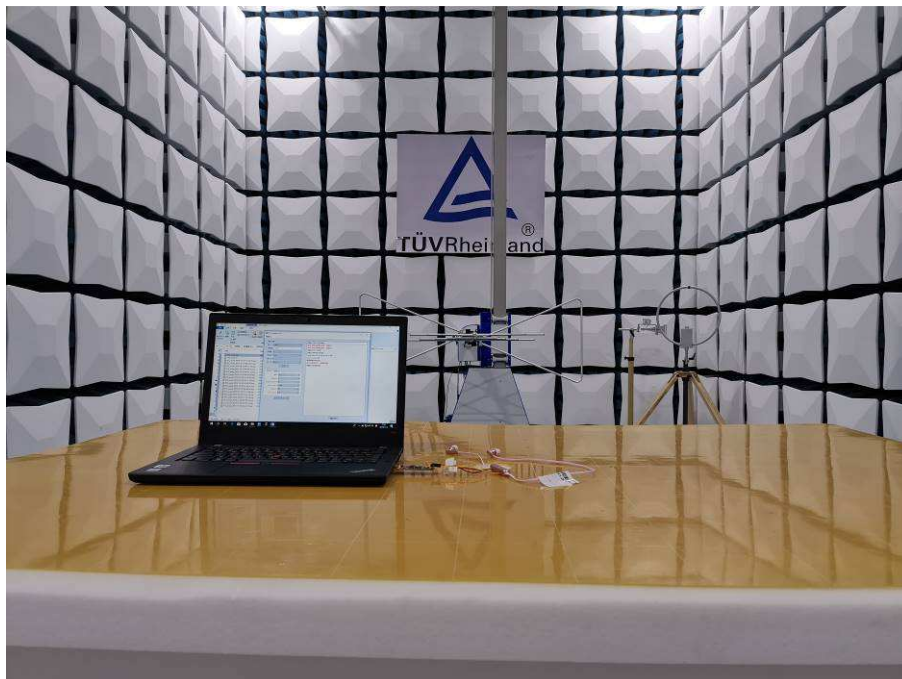
Photograph 2: Set-up for Radiated Spurious Emission, 30MHz ~ 1GHz
