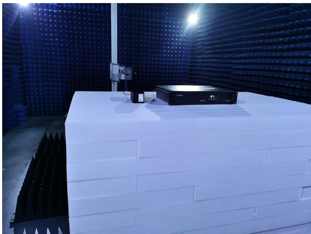
Photo of Radiated Emission Measurement (Above 1G)
