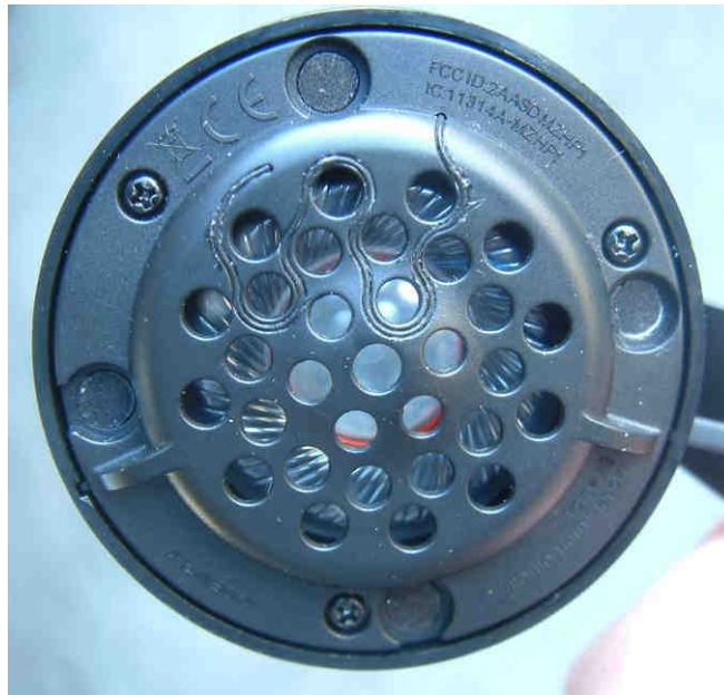
Cushion removed (right side, with label and proximity sensor)
