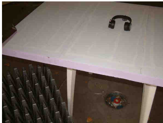
Radiated emission (Pre-scan test setup)
