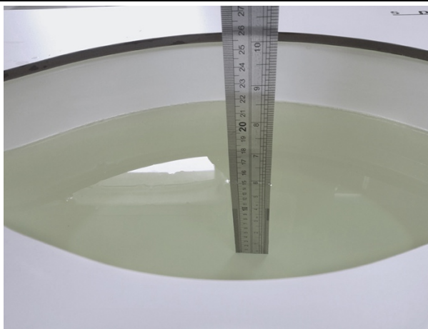
Liquid depth in the body phantom (2450MHz)
