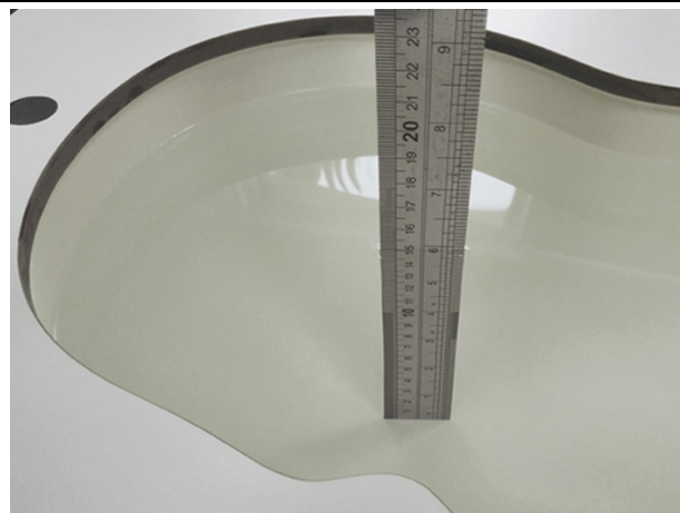
Liquid depth in the head phantom (2450MHz)
