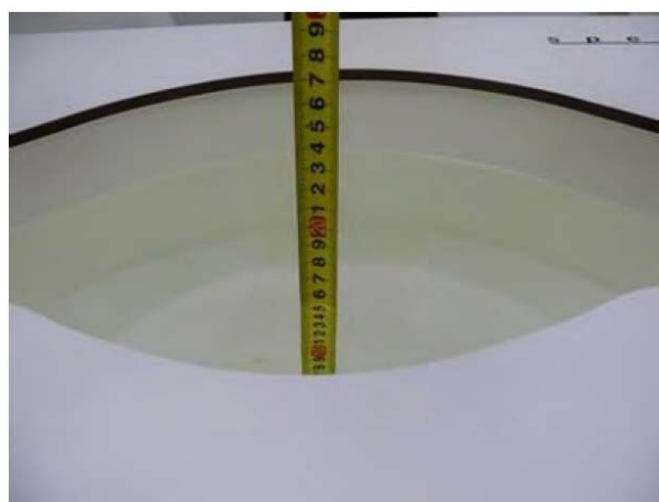
Liquid depth in the body phantom (1900MHz)
