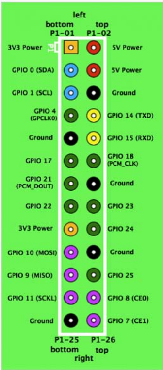
Figure 13: The Raspberry Pi Model B (Rev. 1 and Rev. 2) board GP I/O connector.
