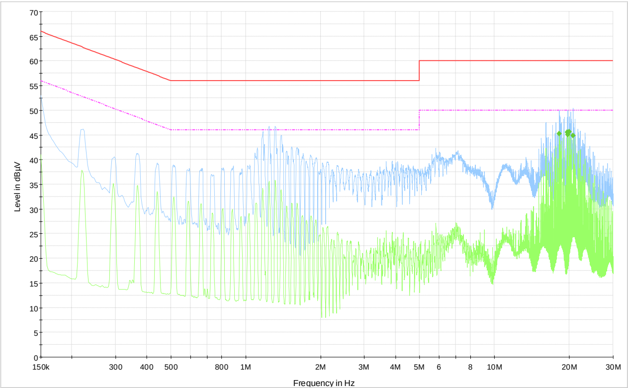
Plot 8.1-1: Conducted emissions on phase line
