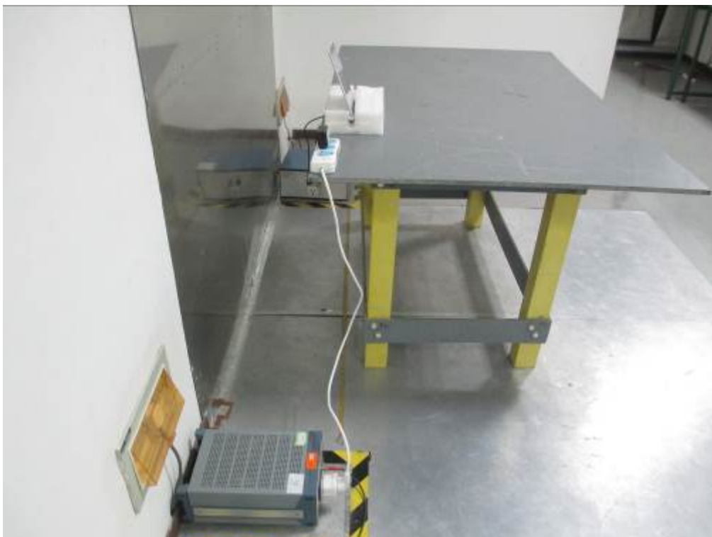
Conducted Emissions Test Setup – Side View
