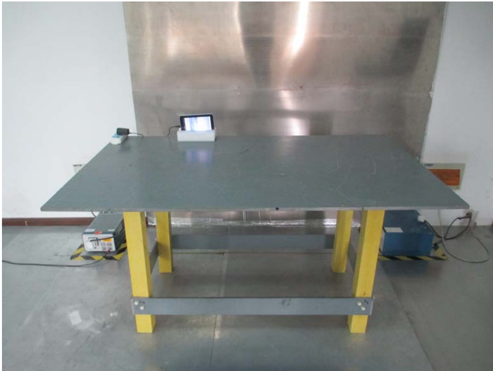
Conducted Emissions Test Setup Front View
