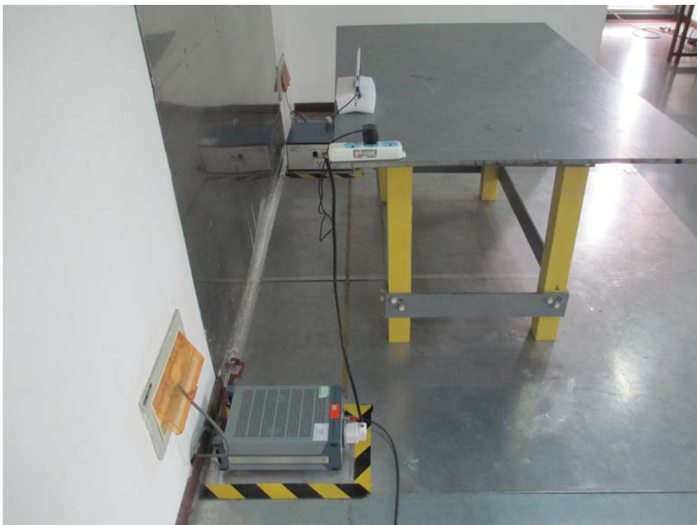
Conducted Emissions Test Setup Side View
