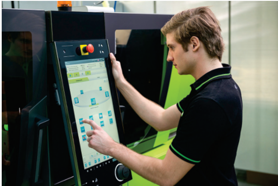
Fig. 29: CC300 Operator Panel installed in an industrial cabinet
