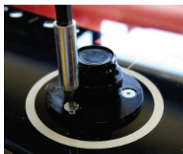
Fig. 39: Unscrew the cap holder of the rotary/push button
