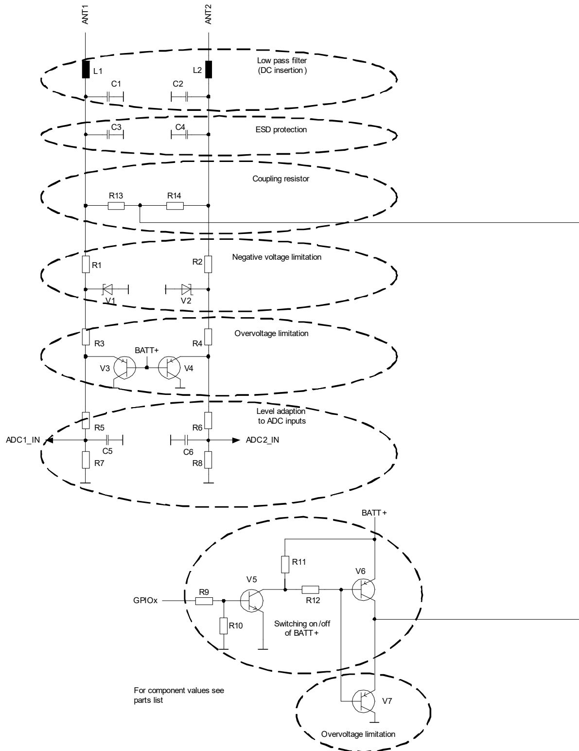
Figure 29: Antenna detection circuit sample - Schematic
