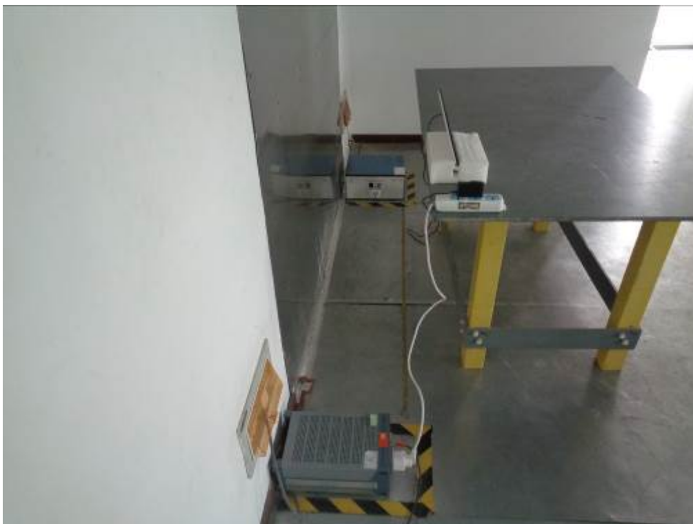
Conducted Emissions Test Setup – Side View
