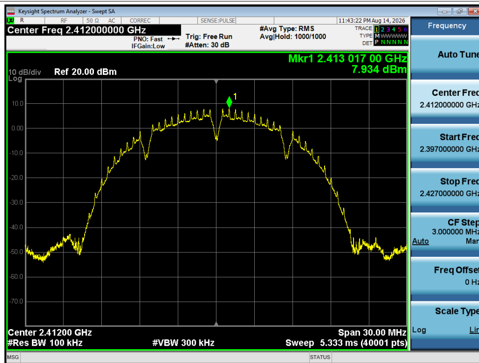
Tx. Spurious NVNT b 2412MHz Ant1 Ref
