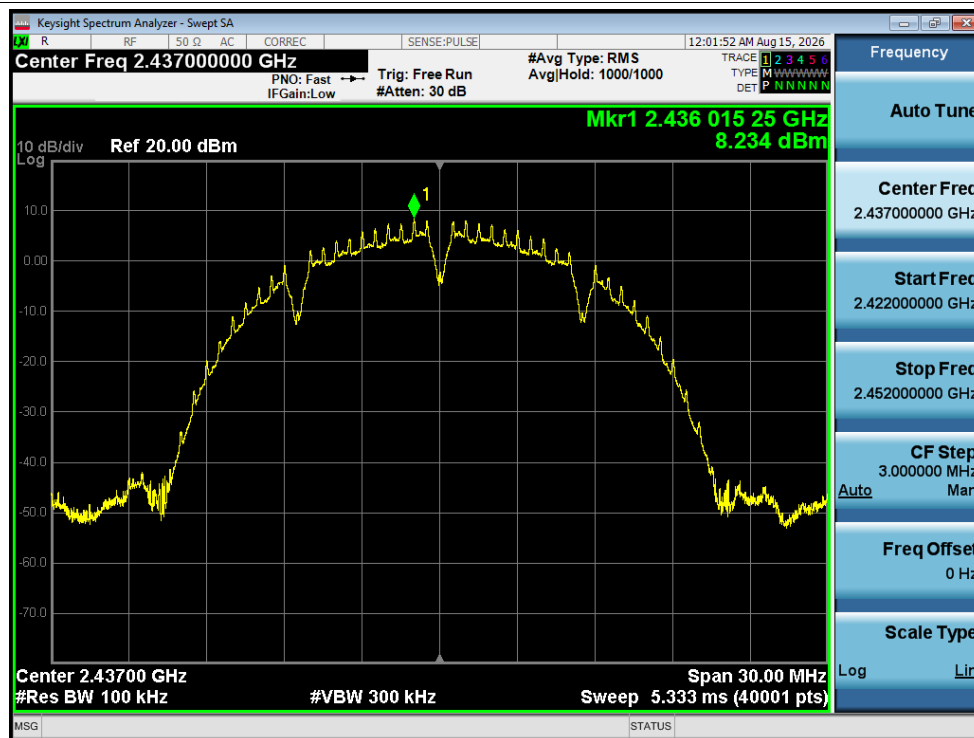
Tx. Spurious NVNT b 2437MHz Ant1 Ref
