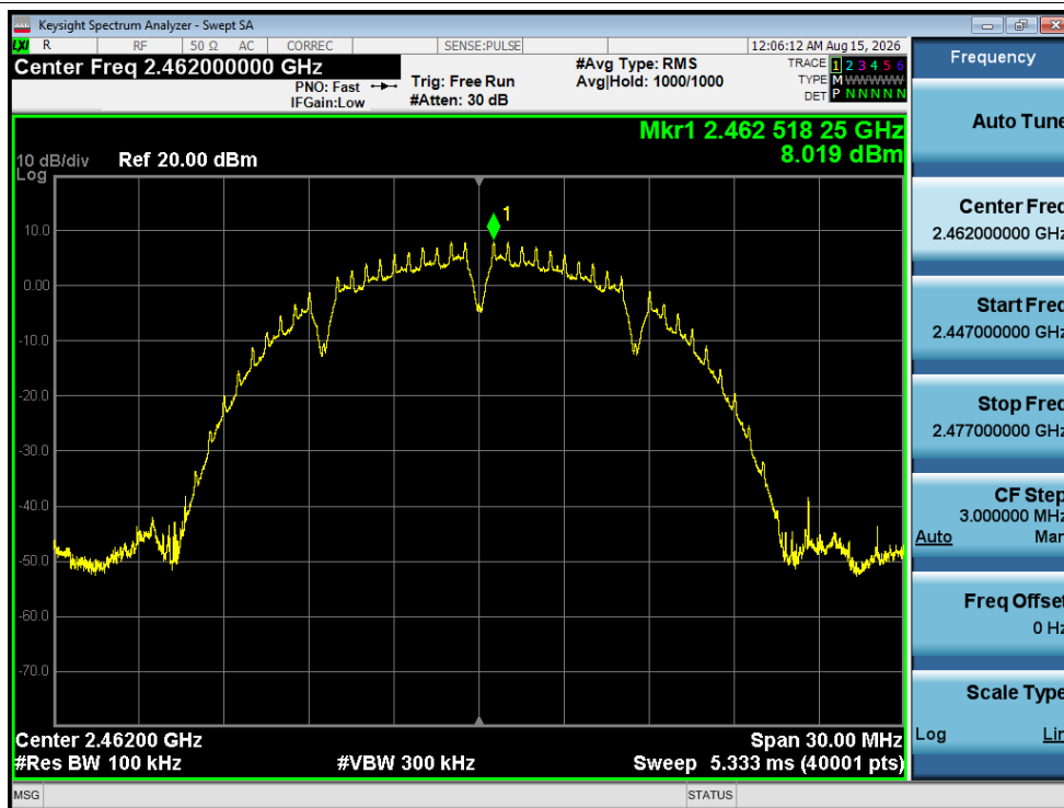
Tx. Spurious NVNT b 2462MHz Ant1 Ref
