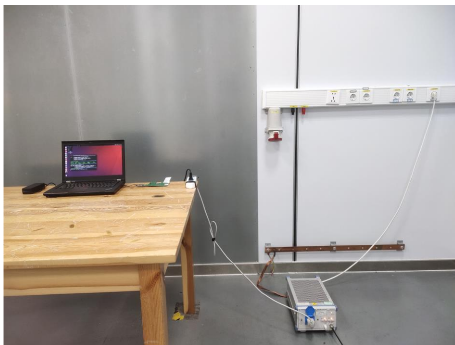
Fig. 4 Power line conducted emission setup photo
