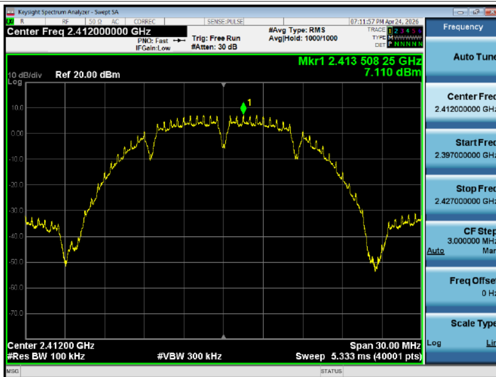
Tx. Spurious NVNT b 2412MHz Ant2 Ref
