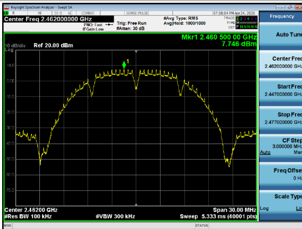
Tx. Spurious NVNT b 2462MHz Ant1 Ref
