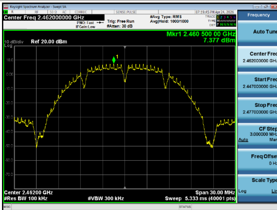
Tx. Spurious NVNT b 2462MHz Ant2 Ref
