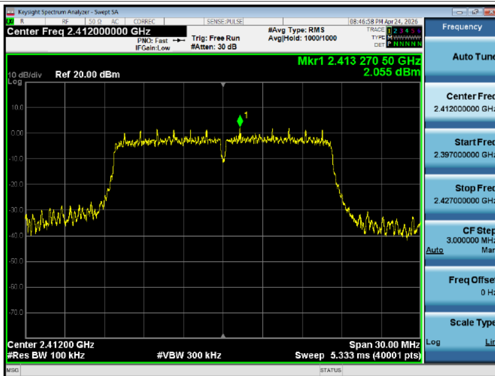
Tx. Spurious NVNT g 2412MHz Ant2 Ref
