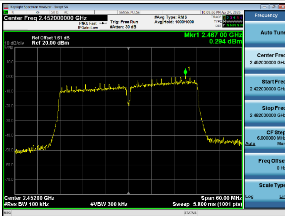
Band Edge NVNT n40 2452MHz Ant2 Ref
