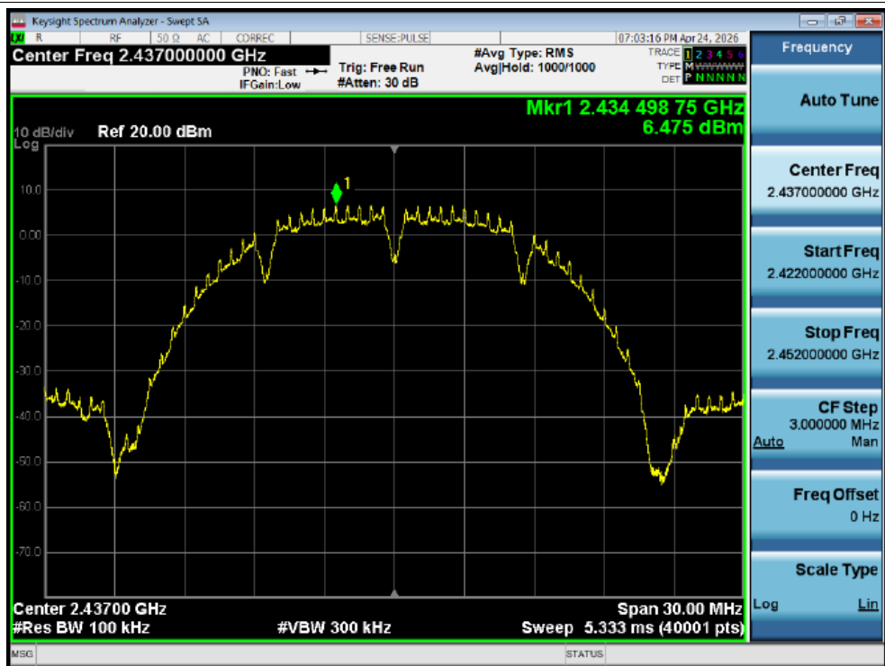
Tx. Spurious NVNT b 2437MHz Ant1 Ref
