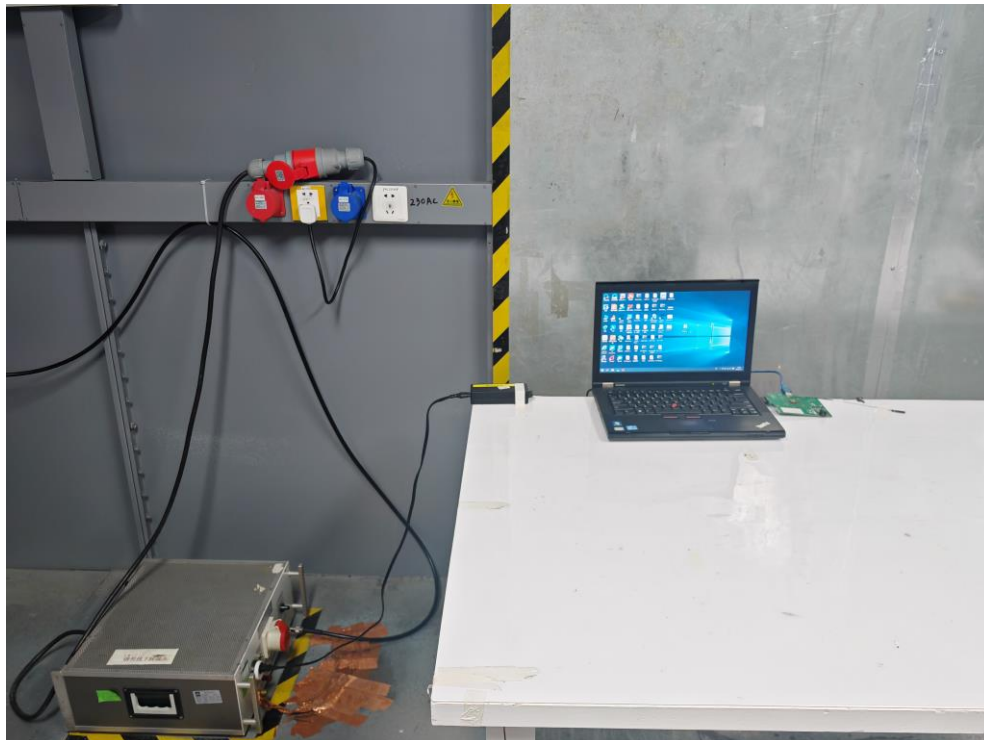
6.2. Photo of Conducted Emission test
