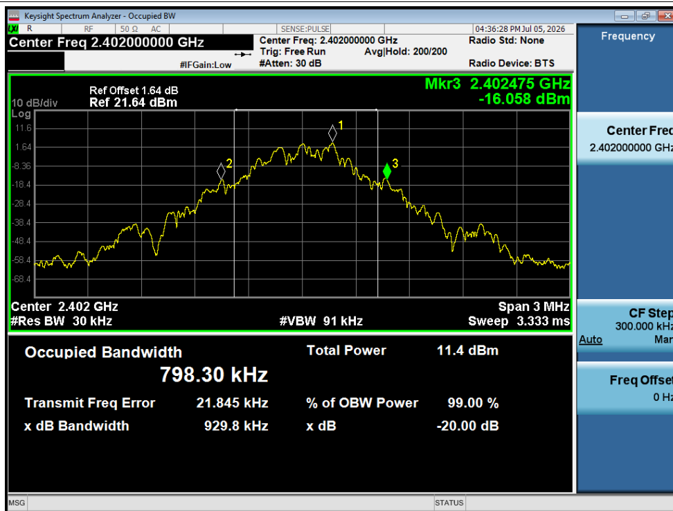
-20dB Bandwidth NVNT 1-DH5 2402MHz Ant1
