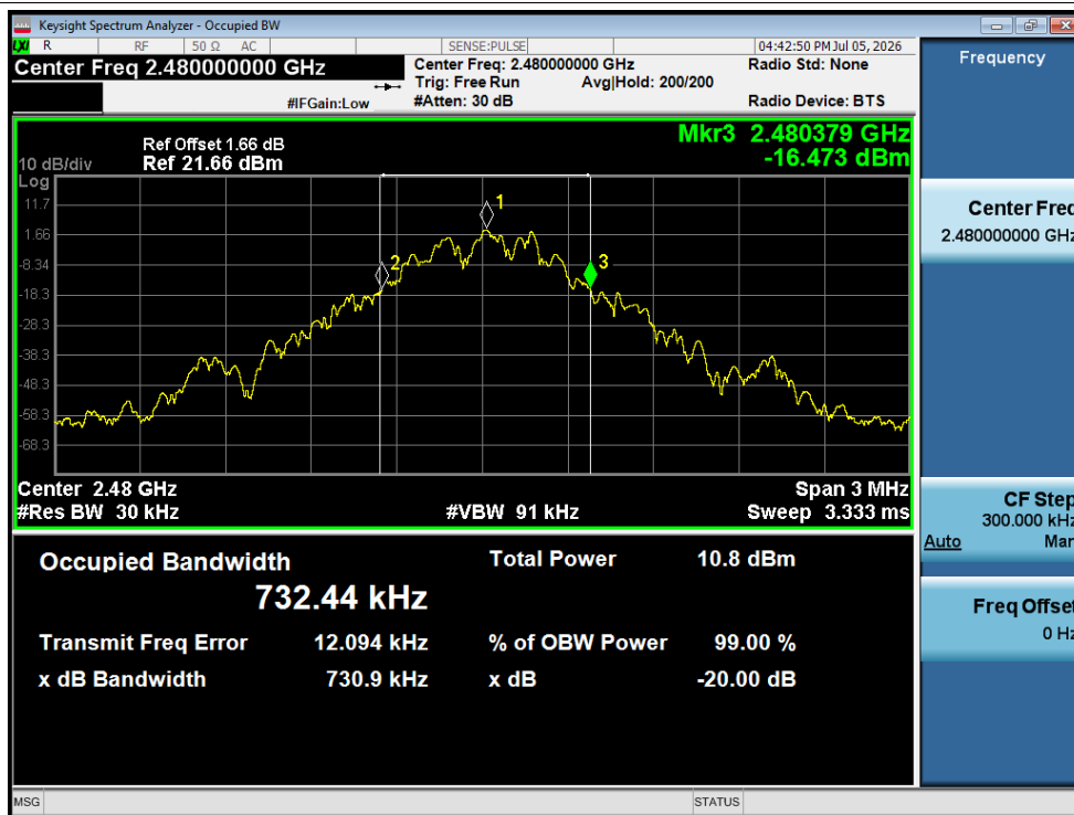
-20dB Bandwidth NVNT 1-DH5 2480MHz Ant1
