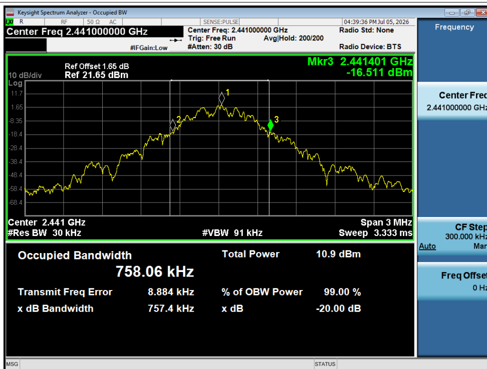
-20dB Bandwidth NVNT 1-DH5 2441MHz Ant1
