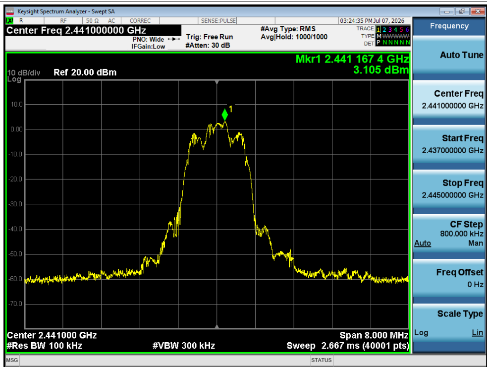
Tx. Spurious NVNT 2-DH5 2441MHz Ant1 Ref
