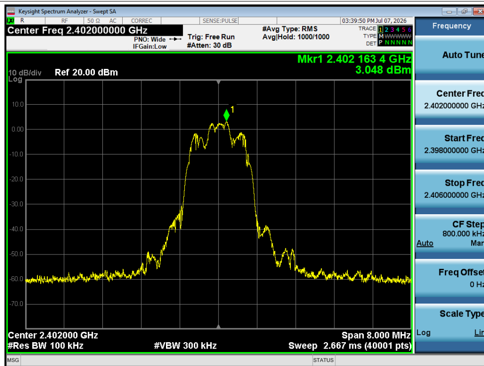
Tx. Spurious NVNT 2-DH5 2402MHz Ant1 Ref
