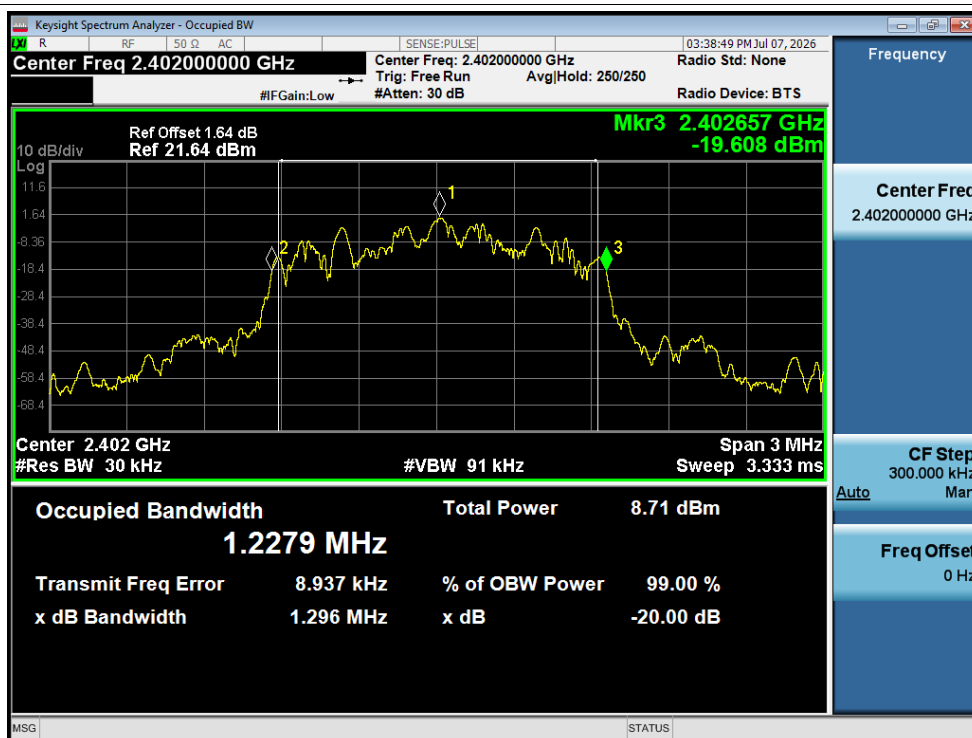
-20dB Bandwidth NVNT 2-DH5 2402MHz Ant1
