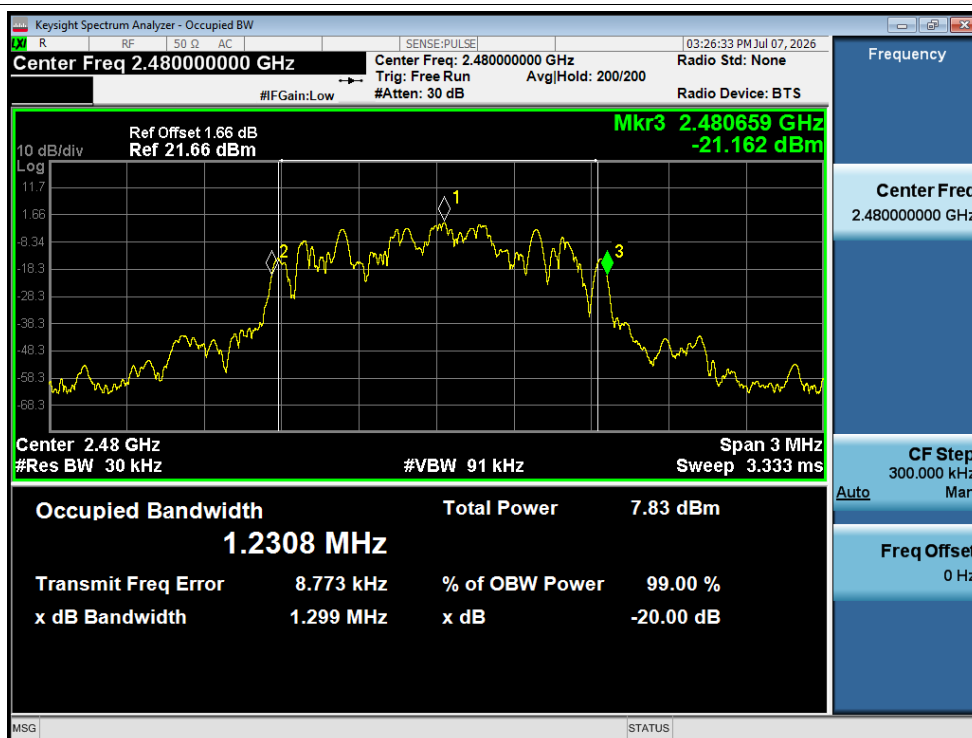
-20dB Bandwidth NVNT 2-DH5 2480MHz Ant1
