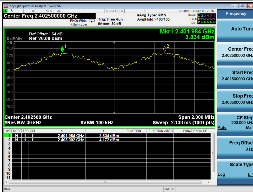
CFS NVNT 1-DH5 2402MHz Ant1
