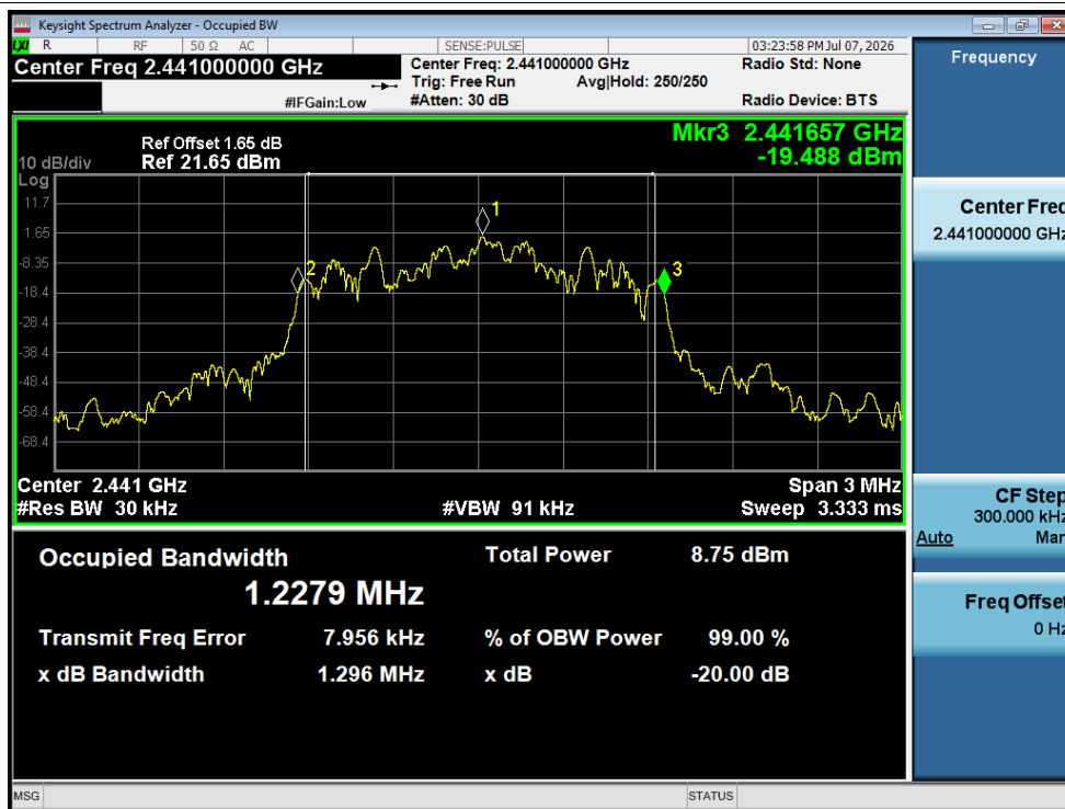
-20dB Bandwidth NVNT 2-DH5 2441MHz Ant1
