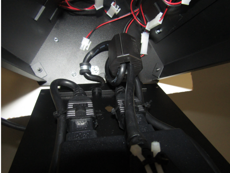
Figure A2: fair-rite Part # 0431176451 ( 2 pass) on AC power cord inside enclosure
