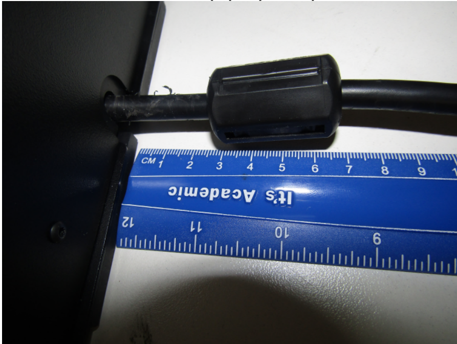
Figure A3: fair-rite Part # 0431167281 ( 1 pass) on AC power cord outside enclosure
